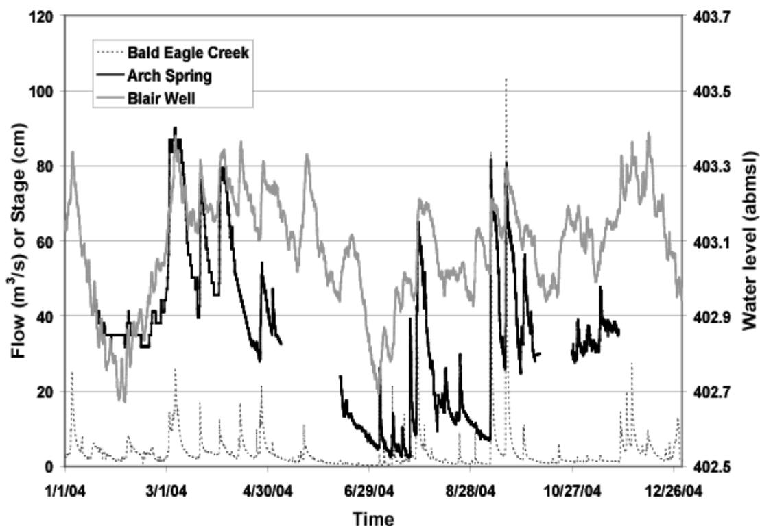
Figure 3-2: Example plot of 2004 data from Blair County water resources: interpolated water level from Arch Spring; interpolated discharge from Bald Eagle Creek at Tyrone; and interpolated water level data from the Blair County drought monitoring well. The gaps in the Arch Spring data in May and October resulted from instrument down time.
