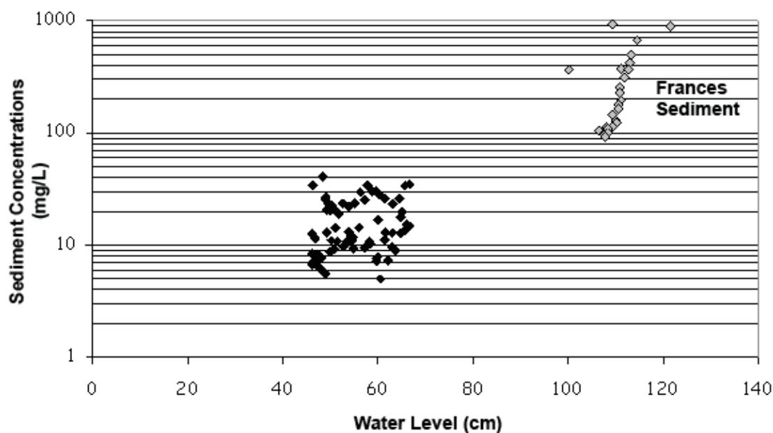
Figure 5-6: Sediment concentrations associated with 2004 samples storms at Arch Spring
