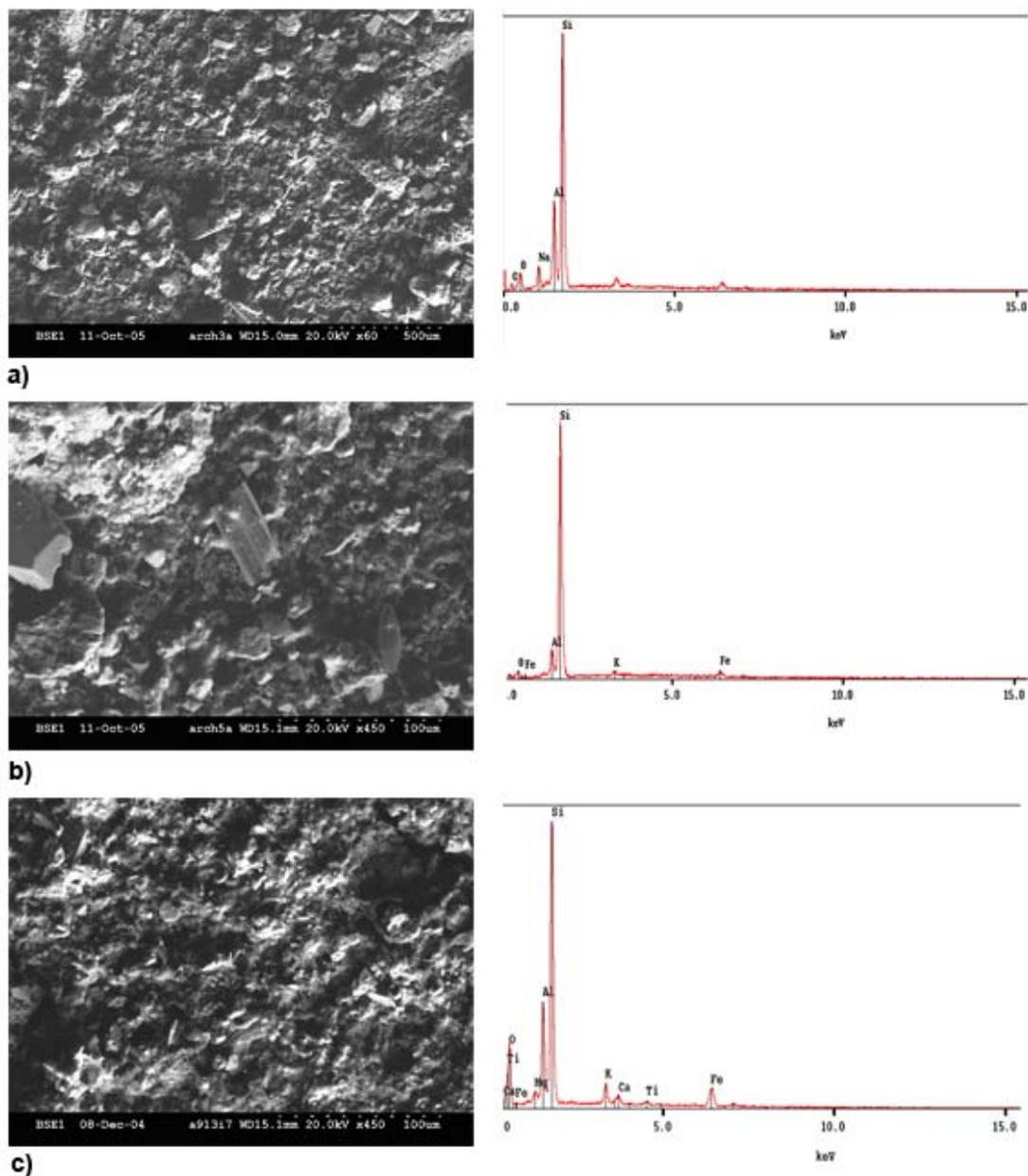
Figure 5-7: SEM images of Arch Spring sediment across a range of conditions including Hurricane Frances. a) This sample was collected by the sampler at 4:19am on 9/9/04 and is the most concentrated sediment collected at the site. b) This sample was collected by the sampler on 9/9/04 at 8:19am. c) This sample was collected by the sampler on 9/1/03 at the peak sediment concentration associated with a small storm event.
