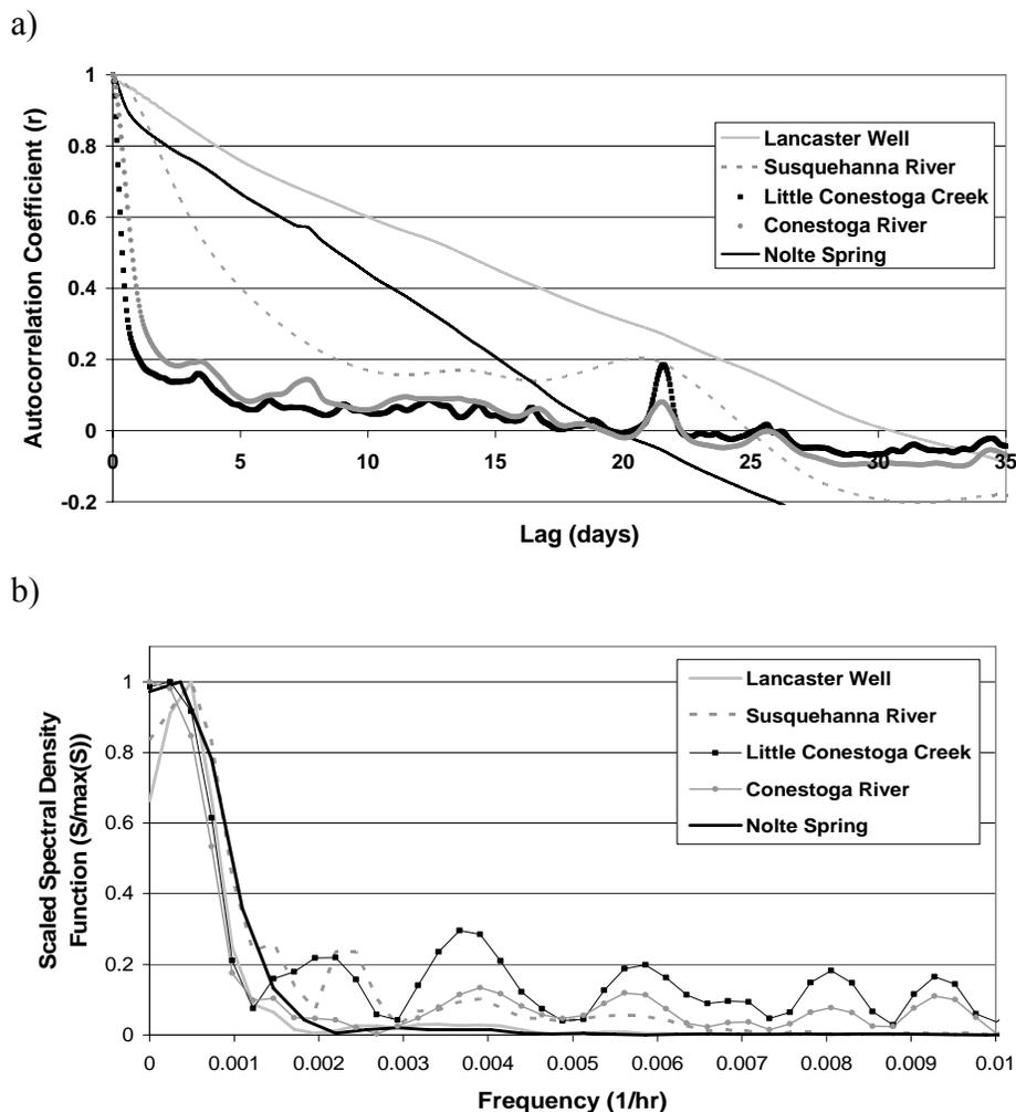
Figure 3-6: a) Plot of 2003 autocorrelation functions for water resources in Lancaster County: Nolte Spring, Conestoga River at Conestoga; Little Conestoga Creek near Millersville; Susquehanna River at Marietta; and the Lancaster County drought monitoring well.
