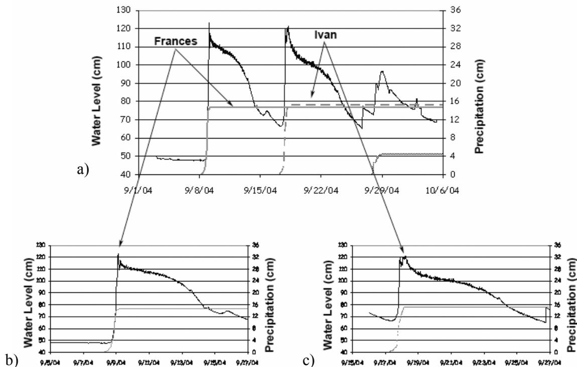
Figure 5-4: Water level data recorded at Arch Spring and cumulative precipitation data recorded at the Blair County – Altoona Airport in September of 2004
