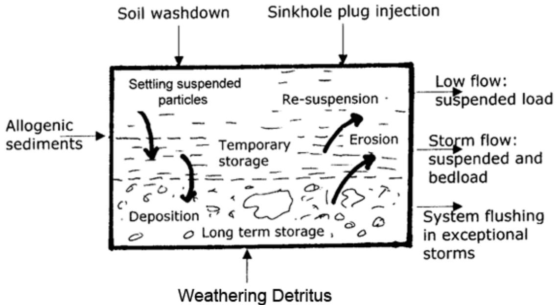
Figure 2-1: The conduit system as a mixing chamber. Sketch shows principal inputs, storage, rearrangement, and transport.
