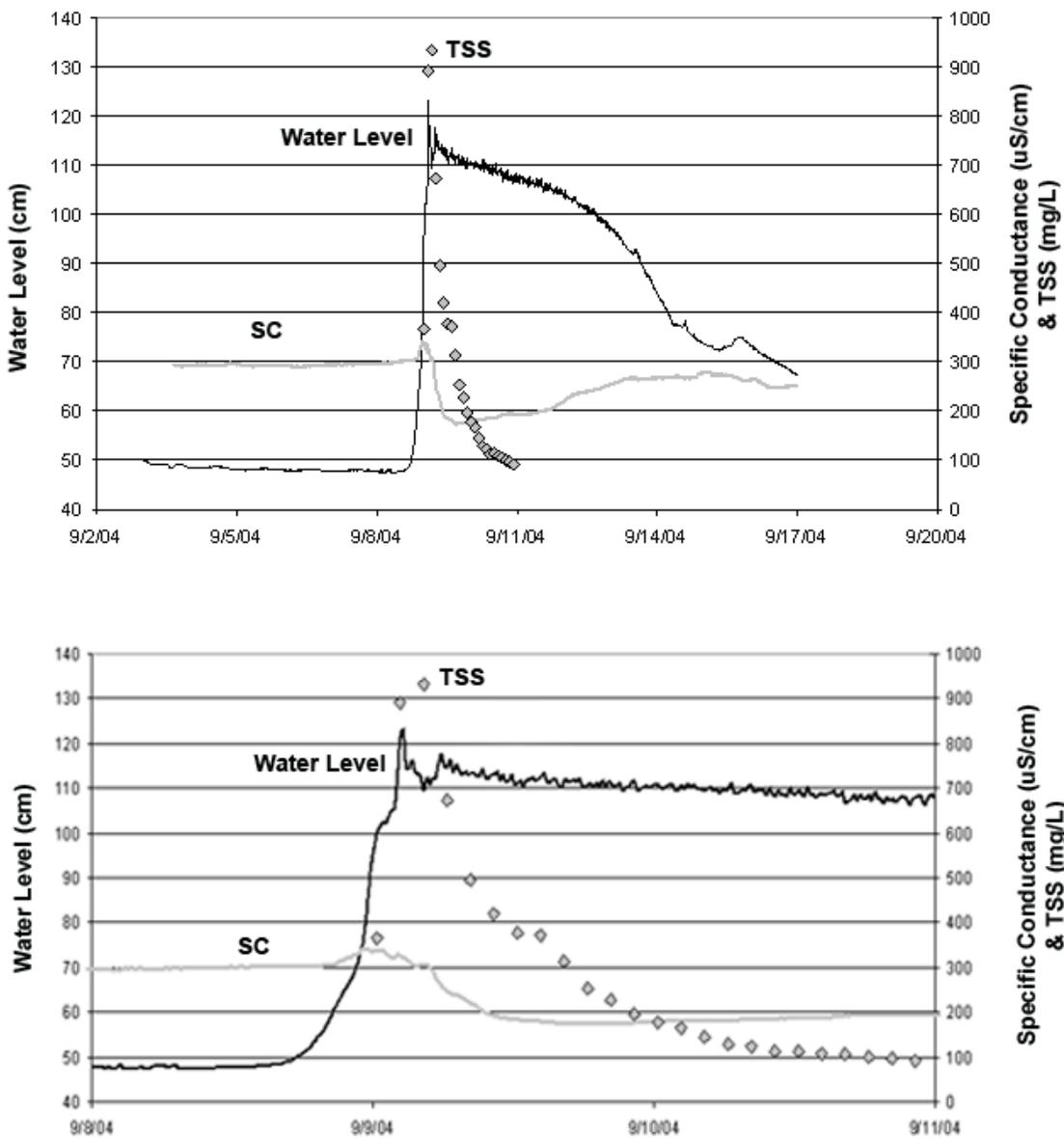
Figure 5-5: Arch Spring water level, specific conductance, and total suspended solids associated with Hurricane Frances. Lower graph shows magnified scale for the Frances event.
