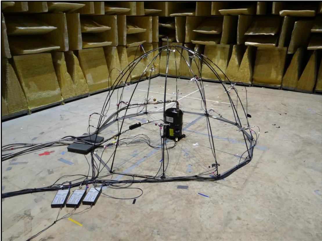
*Figure 2-5. Radiated sound power level measurement setup in hemi-anechoic chamber.*
