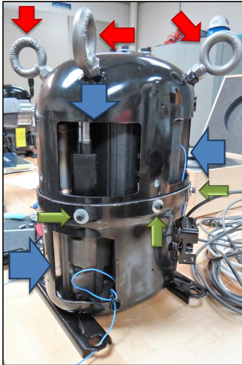
*Figure 2-8. Inoperable compressor used for transmissibility testing.*
