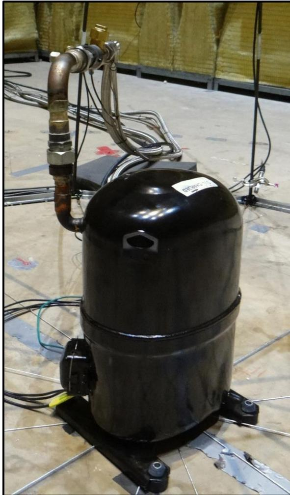
*Figure 1-1. Hermetic reciprocating refrigerant compressor provided by Bristol Compressors International, LLC.*
