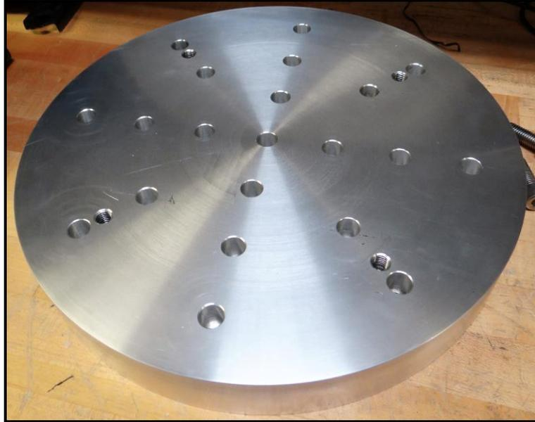
*Figure 2-10. Aluminum fixture plate fabricated for transmissibility testing.*
