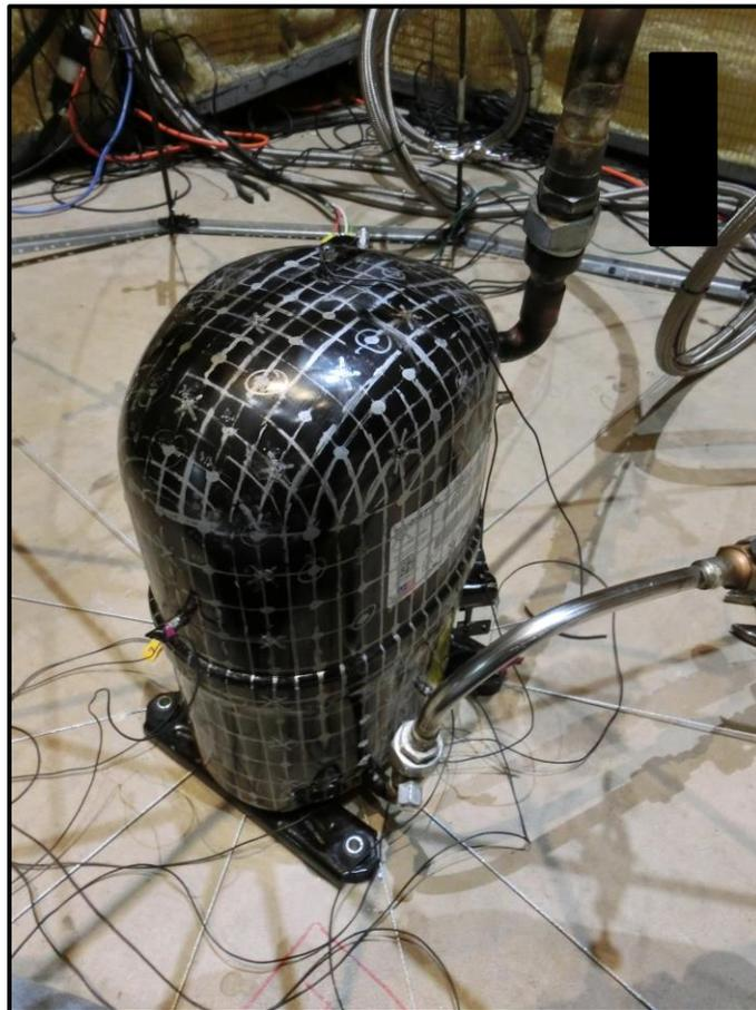
*Figure 2-13. Compressor unit instrumented with accelerometers, used for mobility measurements.*
