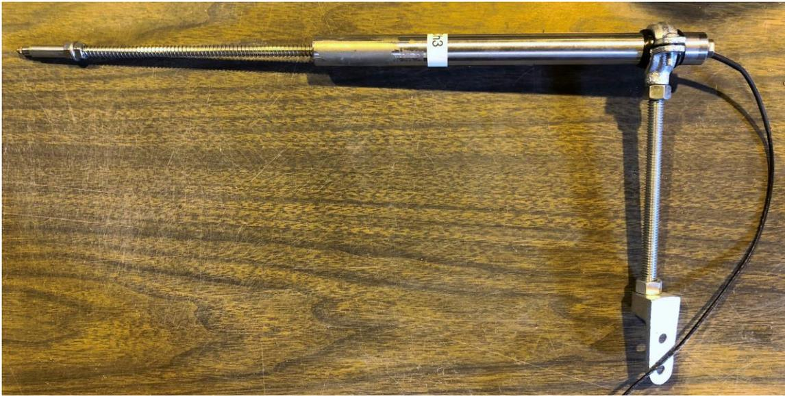
Figure 3-7 LVDT by OMEGA (Model LD621-100)
