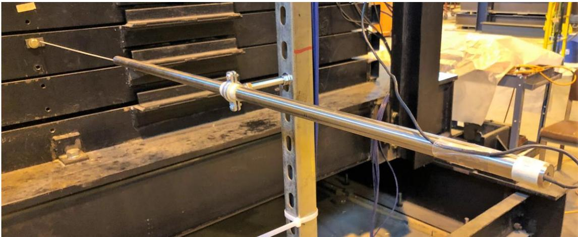
Figure 3-6. LVDT by TE connectivity (Model DC-EC 10000)
