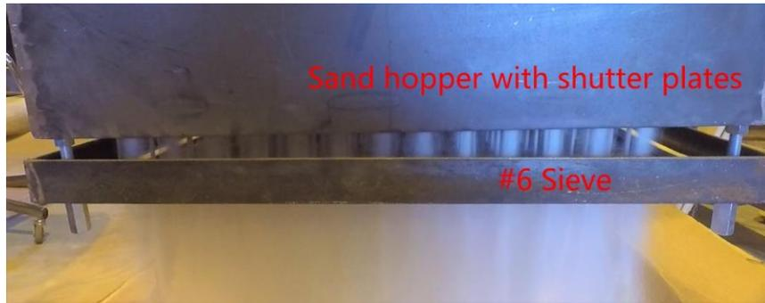
Figure 3-12. Uniform deposition of sand as it passes through the pluviator system
