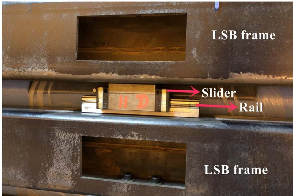
Figure 3-2. The assembly mechanism of frames and pairs of slider & rail
