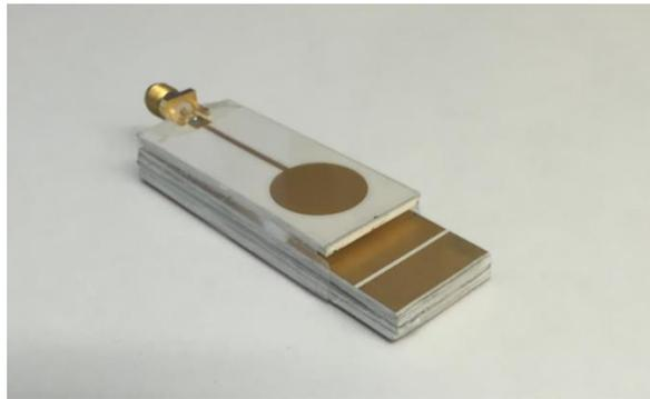
Figure 3-14. Antenna prototype of the proposed dual-band MS artificial ground plane enabled integrated antenna.
