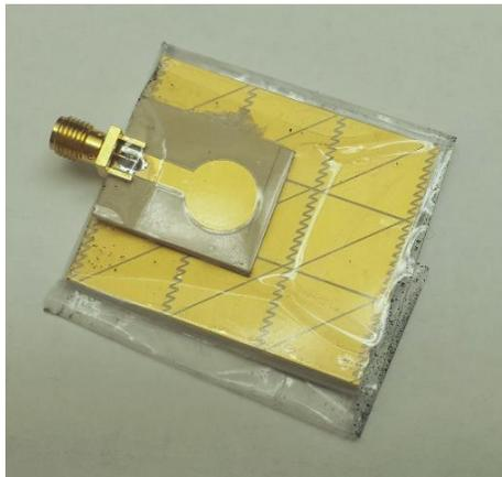
Figure 2-24. Antenna prototype of the ICMS enabled integrated CP antenna design.
