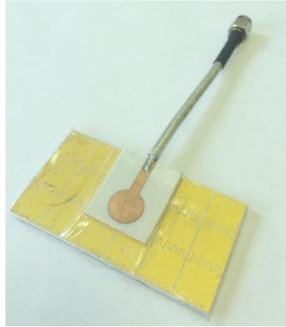
Figure 2-13. Antenna prototype of the 1D loaded ICMS artificial ground plane enabled integrated antenna.
