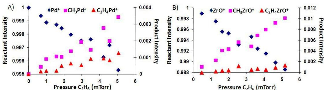
Figure 4-2. a)  $\text{Pd}^+$  and b)  $\text{ZrO}^+$  are reacted with 0 – 5 mTorr  $\text{C}_2\text{H}_6$  at 20 eV in the lab frame. The branching ratios display the decrease in reactant intensity with the concomitant rise in product intensity as the pressure of gas in the reaction cell is increased. Reproduced from reference 31.
