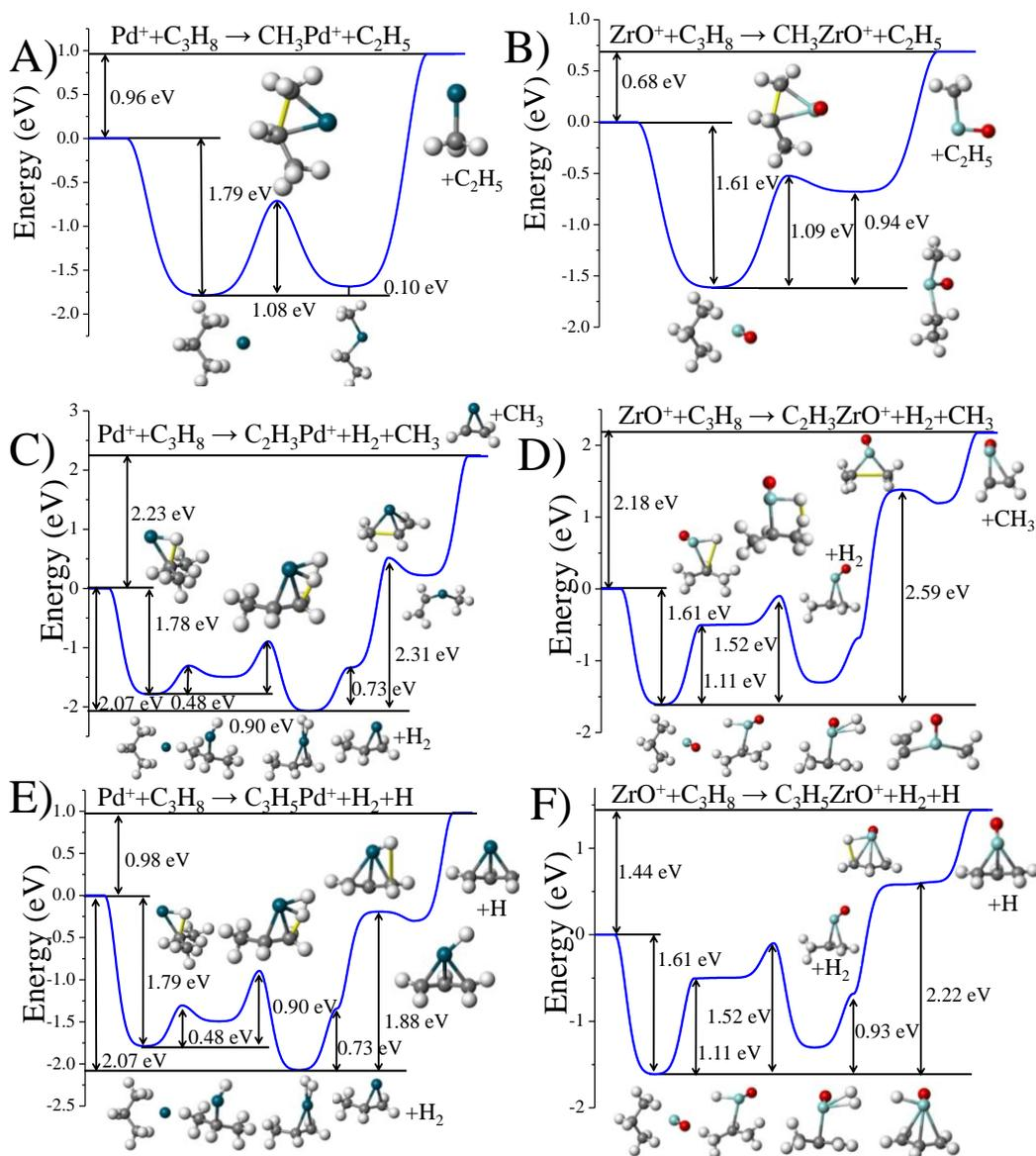
Figure 4-9. Reaction profiles for a)  $\text{Pd}^+$  and b)  $\text{ZrO}^+$  forming  $\text{CH}_3\text{M}^+$ , c)  $\text{Pd}^+$  and d)  $\text{ZrO}^+$  forming  $\text{C}_2\text{H}_3\text{M}^+$ , and e)  $\text{Pd}^+$ , f)  $\text{ZrO}^+$  forming  $\text{C}_3\text{H}_5\text{M}^+$ . Reproduced from reference 31.
