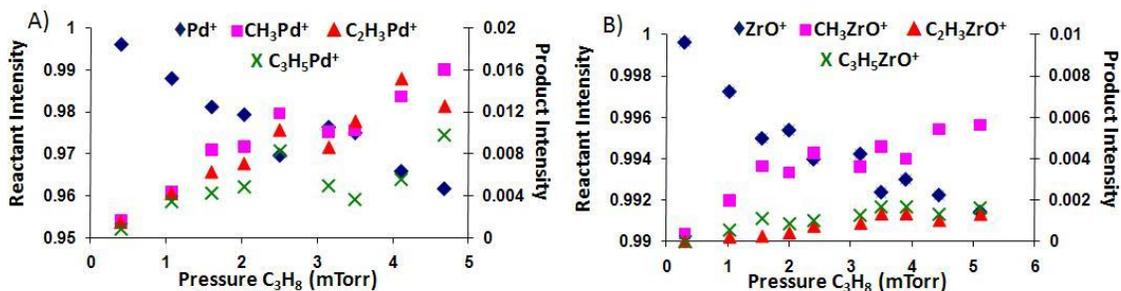
Figure 4-7. a) Pd<sup>+</sup> and b) ZrO<sup>+</sup> are reacted with 0 – 5 mTorr C<sub>3</sub>H<sub>8</sub> at 20 eV in the lab frame. The branching ratios display a decrease in reactant intensity with the concomitant rise in product intensity as the pressure of gas in the reaction cell is increased. Reproduced from reference 31.
