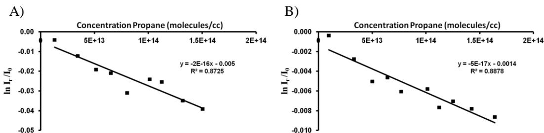
Figure 4-8. Plot of the logarithmic ratios of reactant intensity in the presence and absence of propane ( $\ln I_r/I_0$ ) vs. concentration of propane for a) Pd<sup>+</sup> and b) ZrO<sup>+</sup>.
