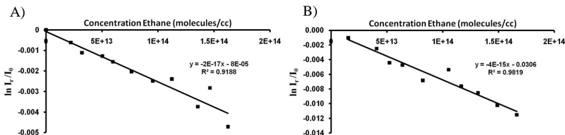
Figure 4-3. Plot of the logarithmic ratios of reactant intensity in the presence and absence of ethane ( $\ln I_r/I_0$ ) vs. concentration of ethane for a)  $\text{Pd}^+$  and b)  $\text{ZrO}^+$ .
