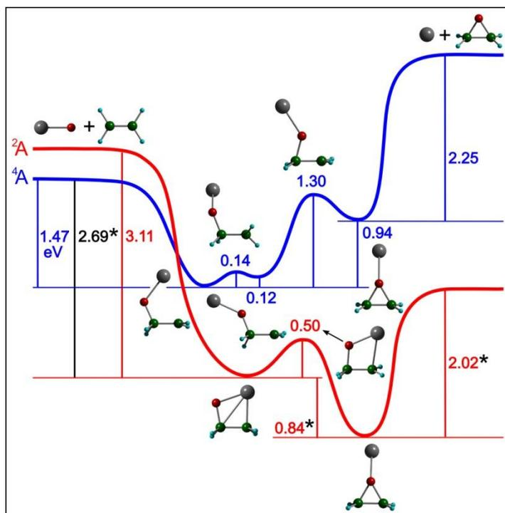
Figure 5-6. Calculated reaction profile for oxidation of  $C_2H_4$  to ethylene oxide by  $PdO^+$ . Profiles for doublet and quartet states are shown. The reaction is exothermic by 1.93 eV in the doublet state and endothermic by 1.72 eV in the quartet state. The energy differences labelled by \* allows for the determination of the most favourable reaction energy by undergoing a spin-crossover that is exothermic by 1.51 eV. Reproduced from reference 18.
