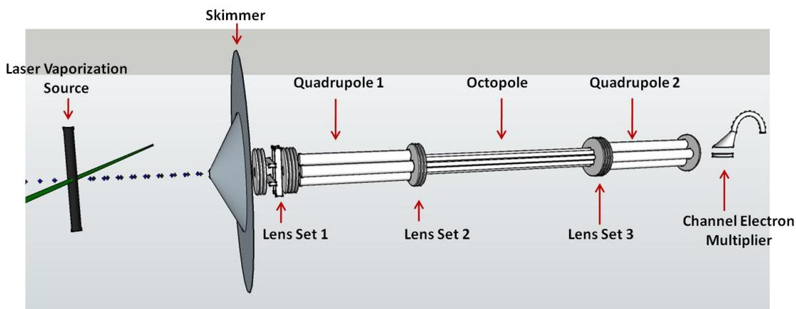
Figure 2-1. Guided-Ion-Beam Mass Spectrometer
