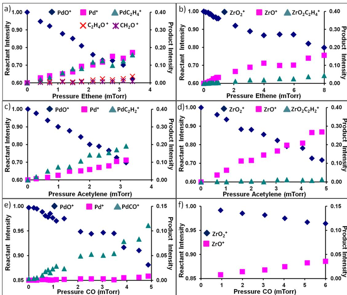
Figure 5-4. Branching ratios presented in normalized ion intensities for the reaction of a)  $\text{PdO}^+$  and b)  $\text{ZrO}_2^+$  with  $\text{C}_2\text{H}_4$ , c)  $\text{PdO}^+$  and d)  $\text{ZrO}_2^+$  with  $\text{C}_2\text{H}_2$ , and e)  $\text{PdO}^+$  and f)  $\text{ZrO}_2^+$  with CO.
