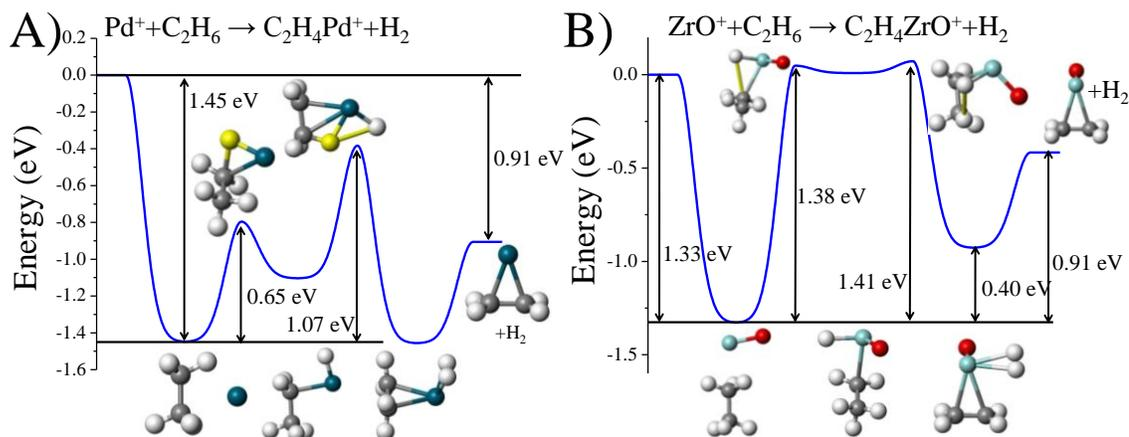
Figure 4-5. Energy profiles for the reaction of a)  $\text{Pd}^+$  and b)  $\text{ZrO}^+$  with ethane to form  $\text{C}_2\text{H}_4\text{Pd}^+$  and  $\text{C}_2\text{H}_4\text{ZrO}^+$ . Reproduced from reference 31.
