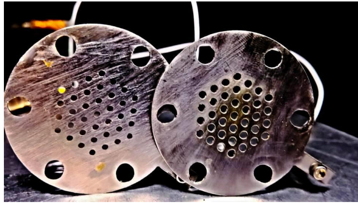
Figure 5-18. Extraction grid set after arc testing
