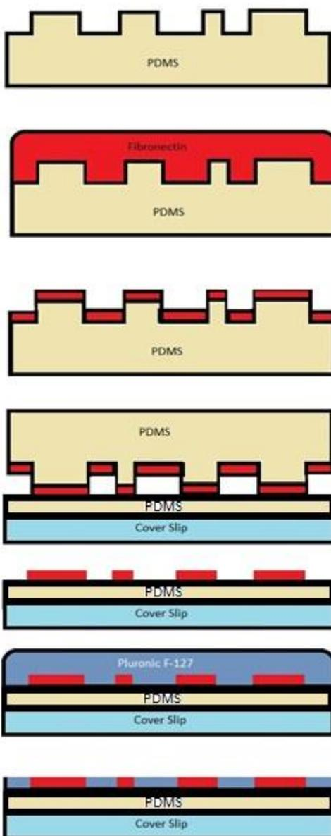
Figure 5. Microcontact printing protocol
