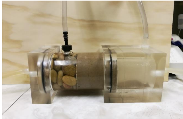
Figure 3-1. Flow cell for soil specimen
