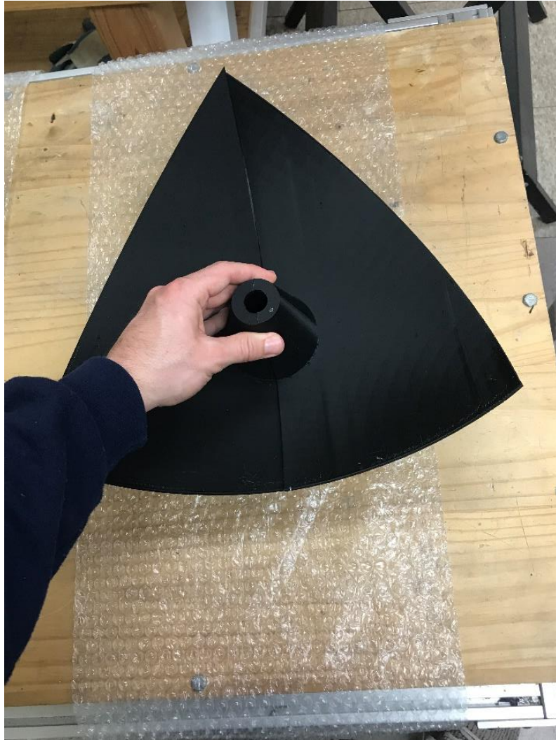
Figure 25. Resulting face piece after assembling two halve pieces together.
