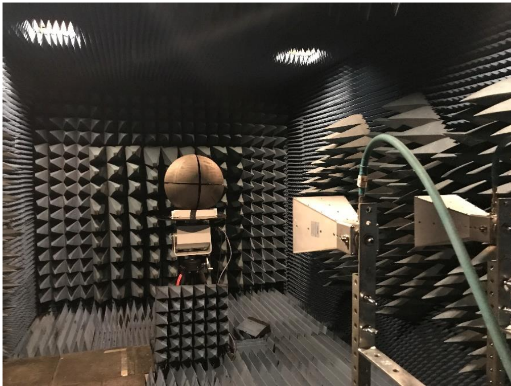
Figure 28. Down range picture of the experimental setup used in the anechoic chamber.
