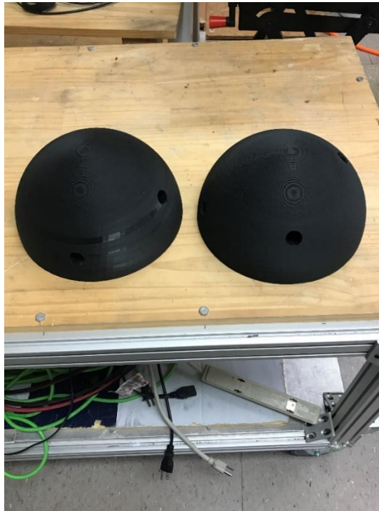
Figure 27. Two halves of the 3-D printed central connector piece.
