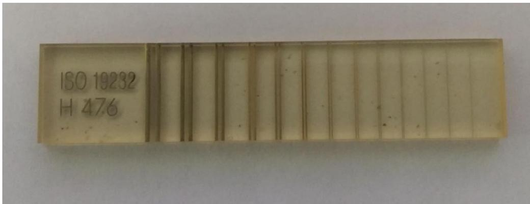
Figure 5 Duplex Wire gauge used to calculate the  $SR_b$
