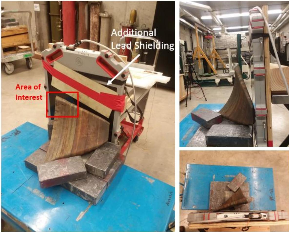
Figure 37 Optimal positioning of the fin in the DR system
