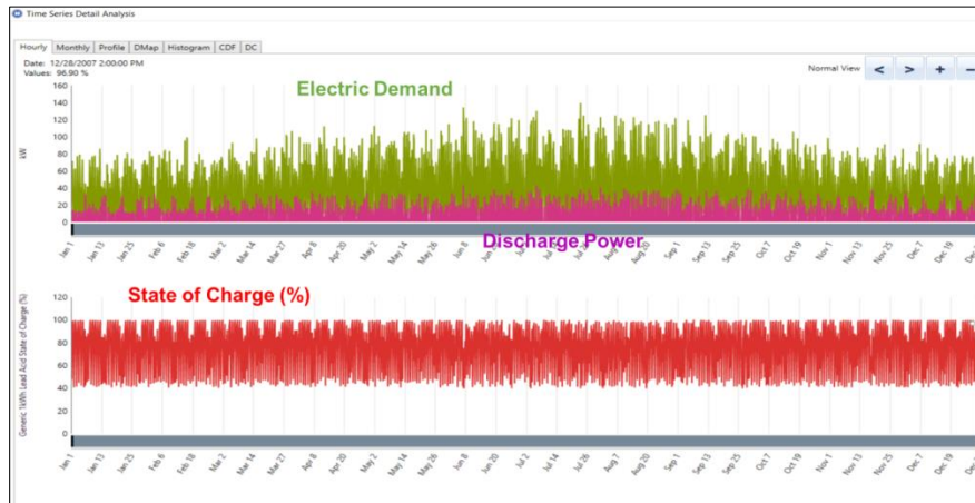
Fig.24 Lead-acid battery state of charge in Bldg.661
