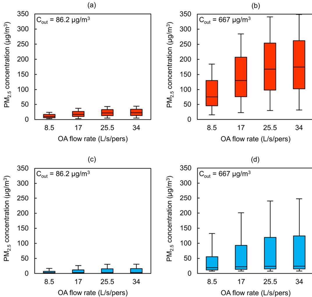
Figure 3. PM<sub>2.5</sub> concentration vs. OA flow rate: (a) AHU filter only,  $C_{out} = 86.2 \mu\text{g}/\text{m}^3$ ; (b) AHU filter only,  $C_{out} = 667 \mu\text{g}/\text{m}^3$  (c) AHU filter + OA filter,  $C_{out} = 86.2 \mu\text{g}/\text{m}^3$ ; (d) AHU filter + OA filter,  $C_{out} = 667 \mu\text{g}/\text{m}^3$ .
