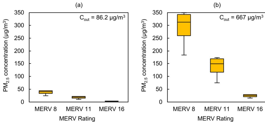
Figure 5. Indoor  $PM_{2.5}$  concentration vs. MERV Rating, AHU filter only: (a)  $C_{\text{out}} = 86.2 \mu\text{g}/\text{m}^3$ ; (b)  $C_{\text{out}} = 667 \mu\text{g}/\text{m}^3$ .
