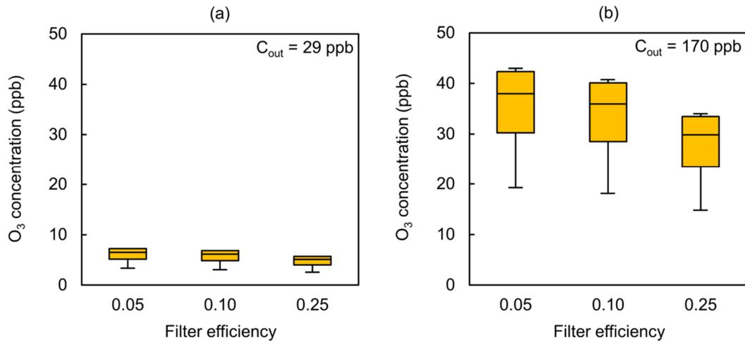
Figure 7. Indoor ozone concentration vs. filter efficiency, AHU filter only: (a)  $C_{out} = 29$  ppb; (b)  $C_{out} = 170$  ppb.
