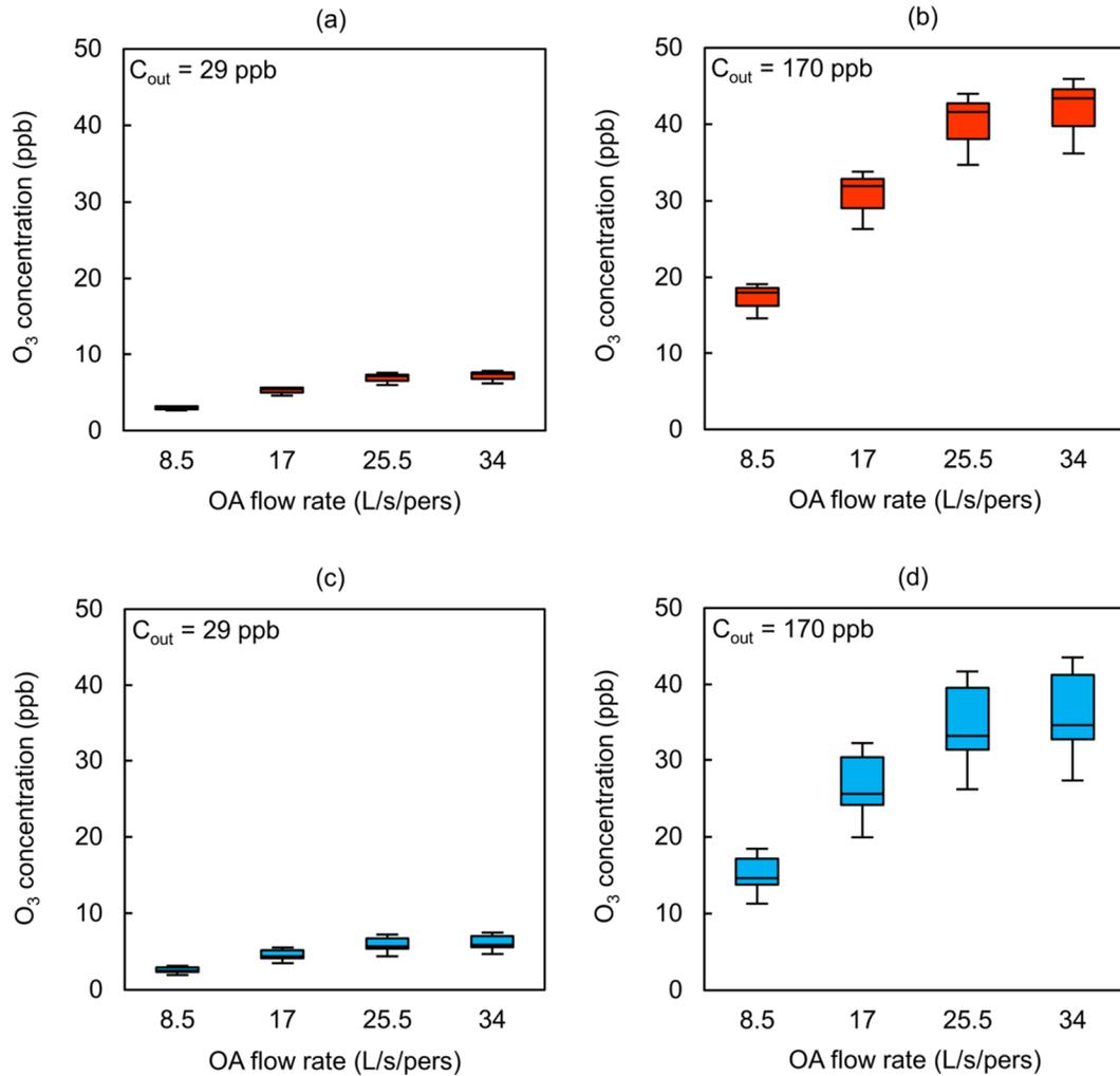
Figure 4. Indoor ozone concentration vs. OA flow rate: (a) AHU filter only,  $C_{out} = 29$  ppb; (b) AHU filter only,  $C_{out} = 170$  ppb (c) AHU filter + OA filter,  $C_{out} = 29$  ppb; (d) AHU filter + OA filter,  $C_{out} = 170$  ppb.
