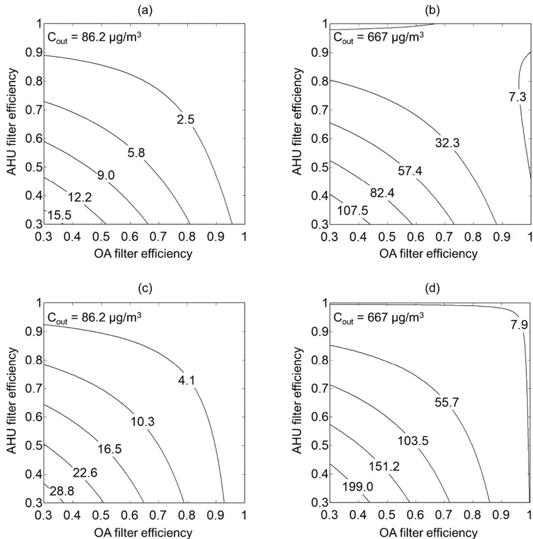
Figure 6. Indoor  $\text{PM}_{2.5}$  concentration vs. filter efficiency, AHU filter + OA filter: (a) OA flow rate = 8.5 L/s/pers,  $C_{\text{out}} = 86.2 \mu\text{g}/\text{m}^3$ ; (b) OA flow rate = 8.5 L/s/pers,  $C_{\text{out}} = 667 \mu\text{g}/\text{m}^3$ ; (c) OA flow rate = 34 L/s/pers,  $C_{\text{out}} = 86.2 \mu\text{g}/\text{m}^3$ ; (d) OA flow rate = 34 L/s/pers,  $C_{\text{out}} = 667 \mu\text{g}/\text{m}^3$ .
