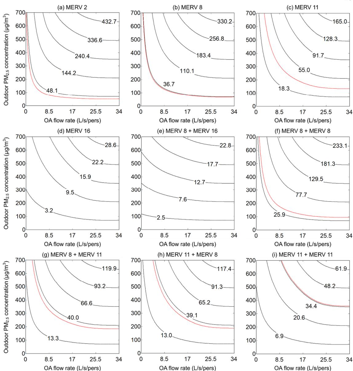
Figure 9. Combined effects of OA flow rate and filters on indoor  $PM_{2.5}$  concentration under outdoor concentration from 0 to  $700 \mu\text{g}/\text{m}^3$ : (a) MERV 2; (b) MERV 8; (c) MERV 11; (d) MERV 16; (e) MERV 8 + MERV 16; (f) MERV 8 + MERV 8; (g) MERV 8 + MERV 11; (h) MERV 11 + MERV 8; (i) MERV 11 + MERV 11.
