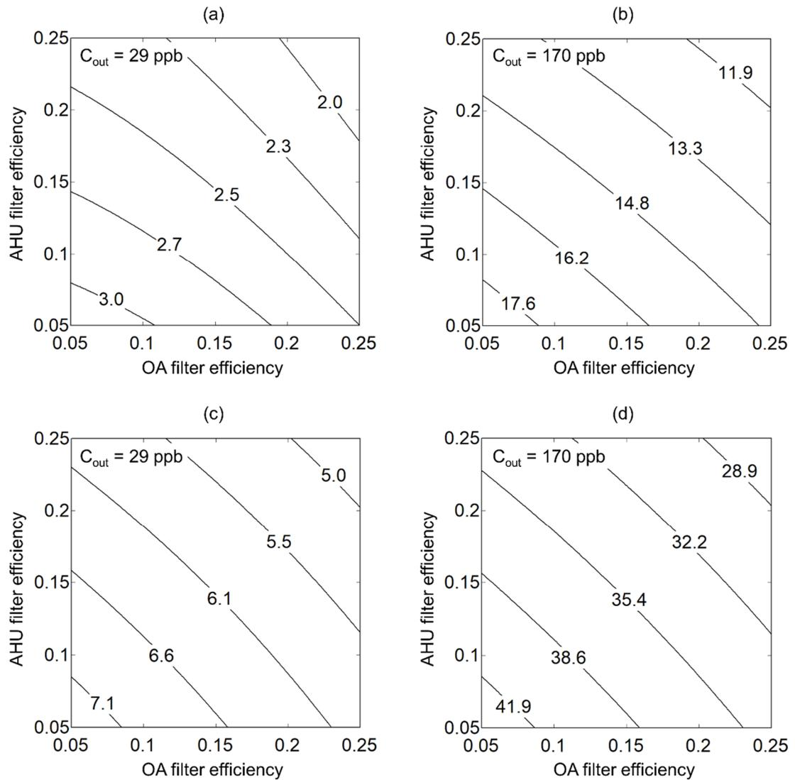
Figure 8. Indoor ozone concentration vs. filter efficiency, AHU filter + OA filter: (a) OA flow rate = 8.5 L/s/pers,  $C_{out} = 29$  ppb; (b) OA flow rate = 8.5 L/s/pers,  $C_{out} = 170$  ppb; (c) OA flow rate = 34 L/s/pers,  $C_{out} = 29$  ppb; (d) OA flow rate = 34 L/s/pers,  $C_{out} = 170$  ppb.
