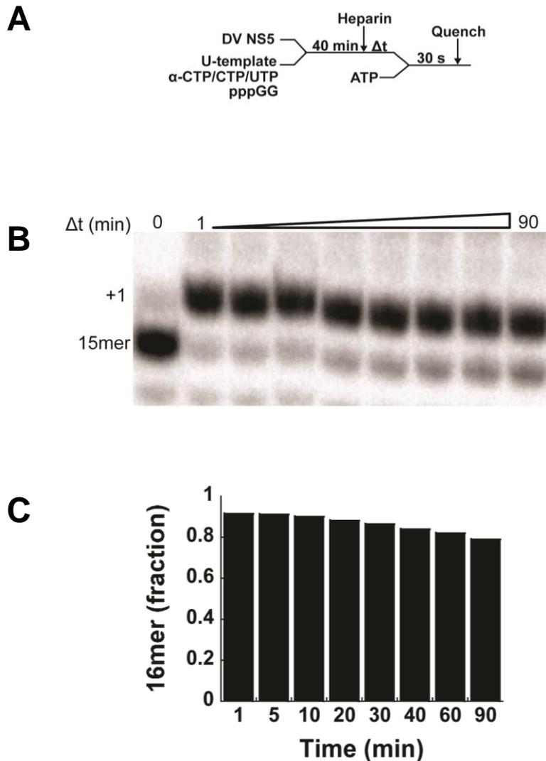
**Figure 14: DV NS5 Assembles in Stable Complexes Competent for AMP Incorporation (A)** Experimental design. After the addition of heparin, the reaction was mixed with ATP at the indicated times, and after 30 s quenched. **(B)** Samples were resolved in a 20% denaturing polyacrylamide gel. **(C)** Shown is the time course of 16-mer product formation from the experiment described in A.
