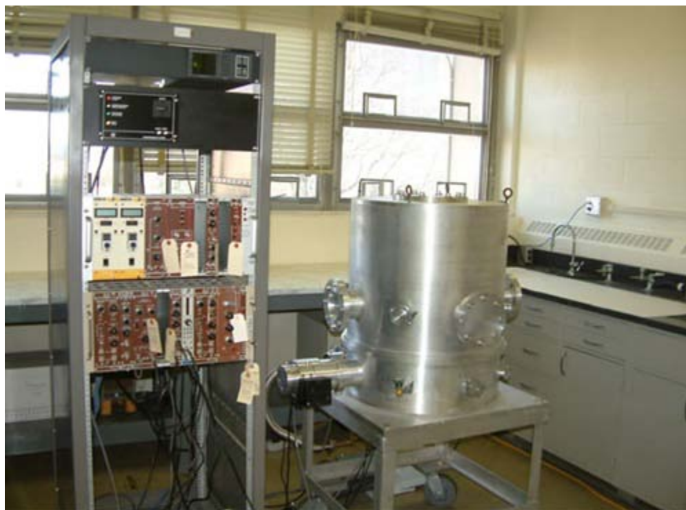
Figure 3-3: Picture of the NDP setup: electronic instruments (left) and vacuum chamber (right)
