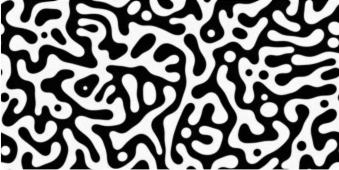
Figure 4-3. Spatial distribution of the two-phase structure of the P(VDF-TrFE)/P(VDF-TrFE-CFE) composite with a 50/50vol% phase fraction. P(VDF-TrFE) is shown by the white regions, while P(VDF-TrFE-CFE) is shown by the black regions.
