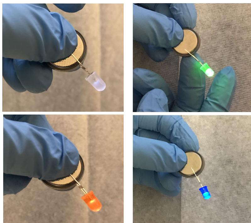
Figure 3-23 Light-emitting diodes with different color could be lighted up by Li/CPOSS-IL-LiTFSI/Li cell at room temperature.
