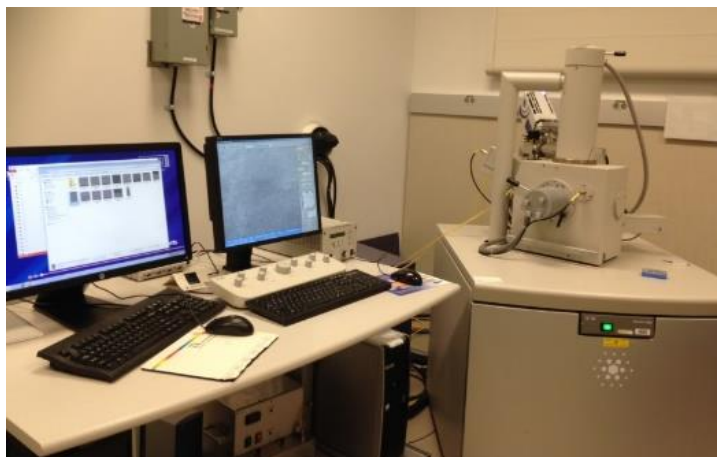
Figure 2-10. The FEI Quanta 200 Environmental scanning electron microscope (SEM) instrument located within the Materials Characterization Laboratory at the Pennsylvania State University.
