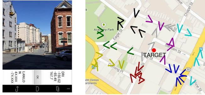
**Figure 5.2.** (a) Screenshot of the programmed phone. (b) We take 40 photos and assign them to 8 nodes in the trace. The locations and orientations of the photos are shown in V shapes, where the photos assigned to different nodes have different colors.
