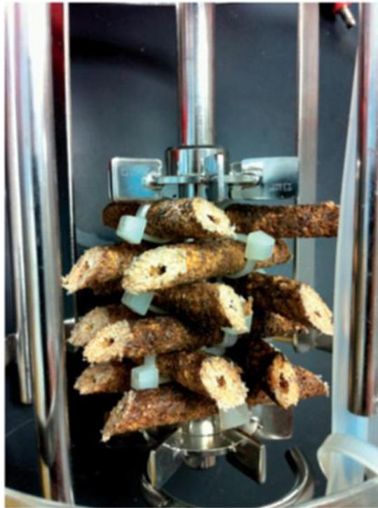
Figure 4.1. PCS grid formation in bioreactors.
