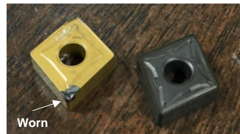
Figure 4-13. A worn (left) and a new (right) coated tungsten carbide cutting tools.
