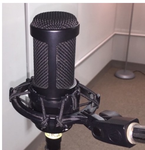
Figure 3.11 This is a picture of the condenser microphone seated within a shock mount. The shock mount protects vibrations from the attached stand (bottom right) from transmitting into the transducer element.
