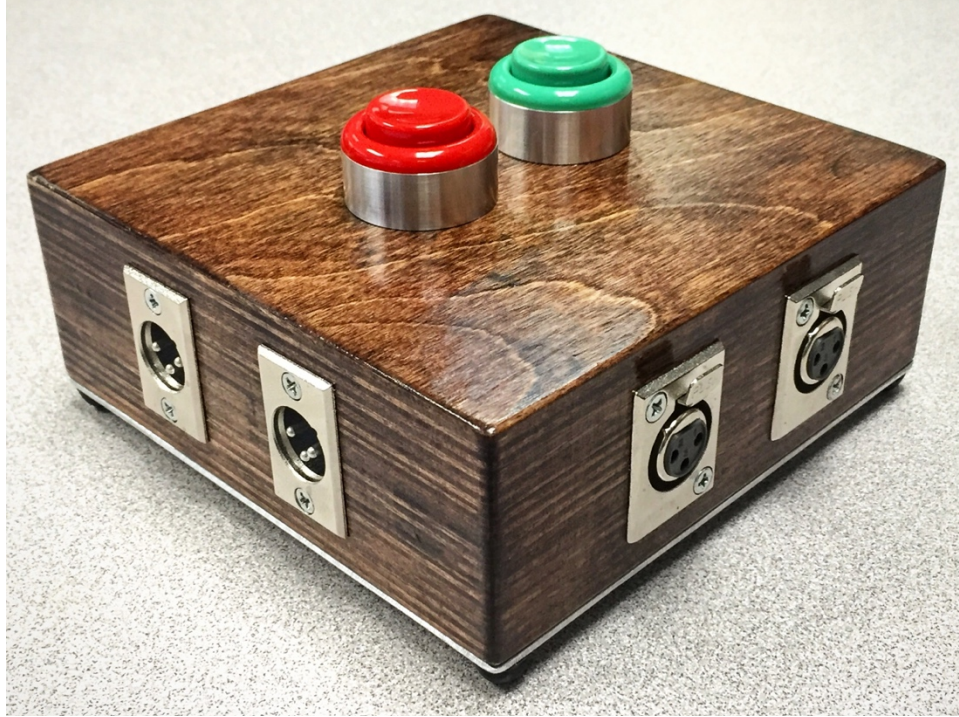
Figure 3.9 This is a picture of the "Push-to-Talk" box. This device features two input-output pairs each accompanied by a button that mutes (red) or unmutes (green) the connection to the microphone.
