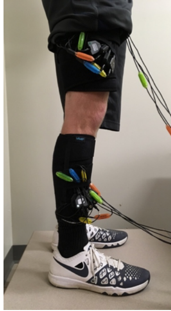
Figure 6.2. Surface EMG setup on the right leg for muscle demand measurement
