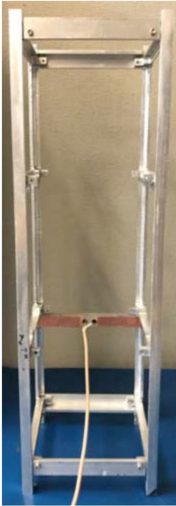
Figure 20: Dipole with ground plane in CubeSat frame
