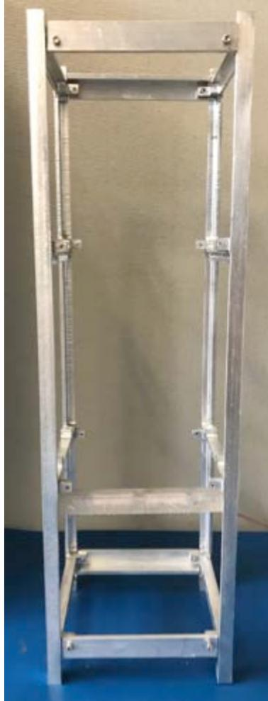
**Figure 18: Dipole attached to CubeSat frame as cross-brace**
