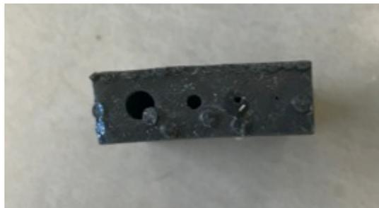
**Figure 9: Resin leakage after vacuum testing**
