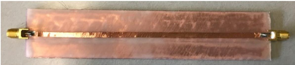
**Figure 13: Microstrip line (Front View)**
