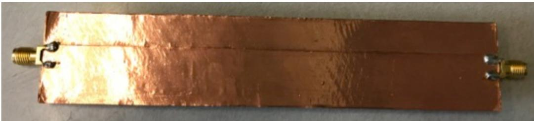
**Figure 14: Microstrip line (Back View)**
