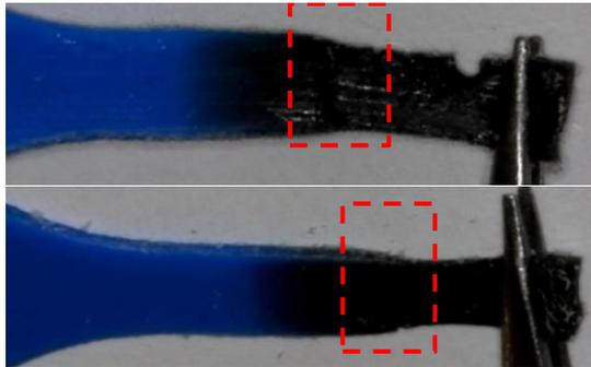
Figure 5-3: Tested fatigue specimens with continuous material gradients showing failure in the flexible, TB+, region and a step discontinuity in the transition region.
