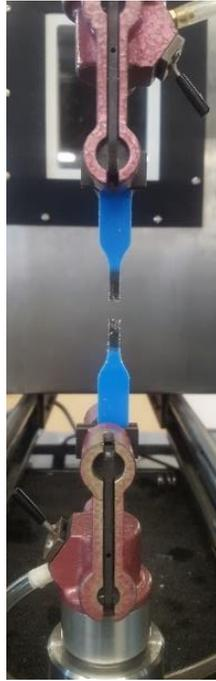
Figure 4-2: Fatigue testing with the Instron 5866 Mechanical Testing System showing a failed specimen.
