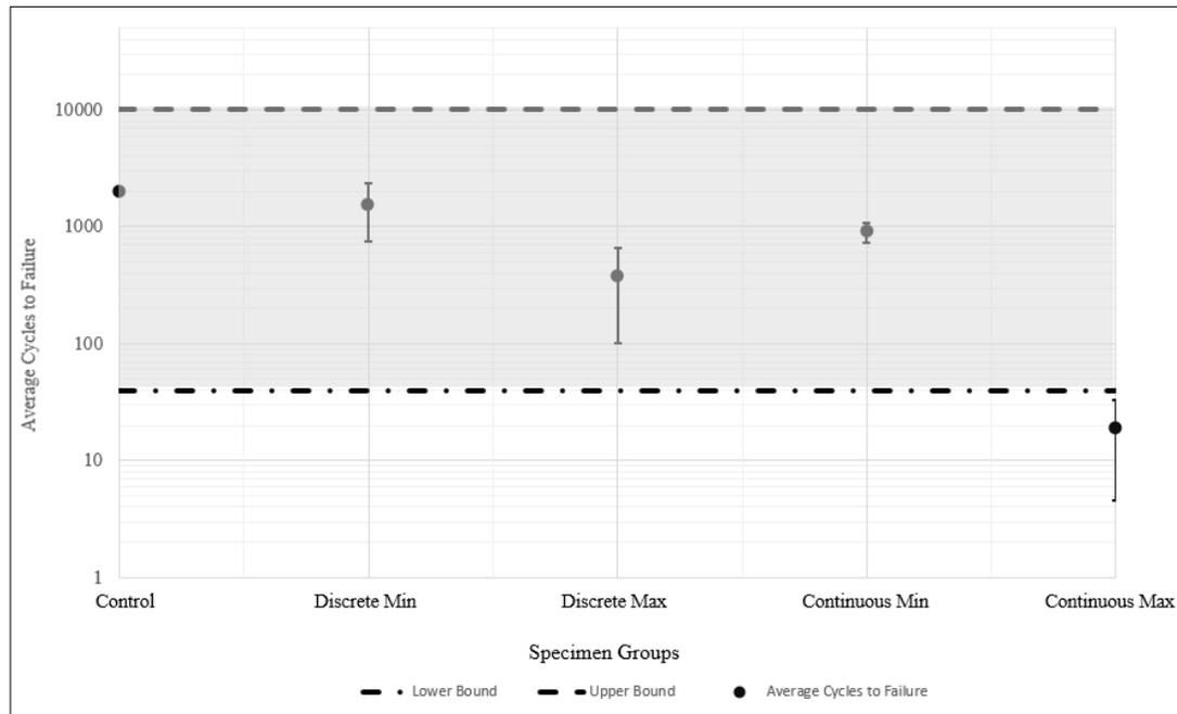
Figure 5-2: The average number cycles to failure with the standard deviations error bars compared against all specimen groups tested.
