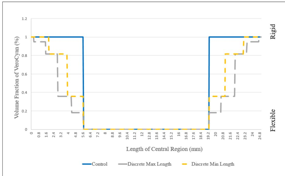
Figure 3-13: Plot showing the maximum and minimum lengths of the discrete material gradients in relation to the material transition of the control specimens for a constant TB+ length.
