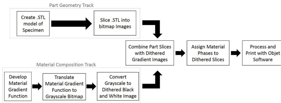
Figure 3-3: Flowchart showing the systematic design process of the continuous material gradient specimens.
