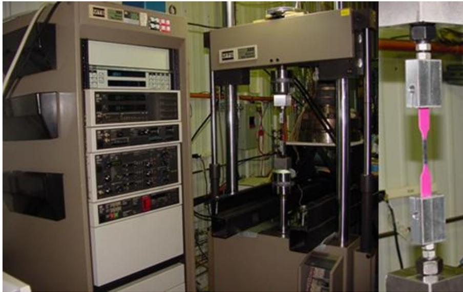
Figure 4-1: The MTS 880 Servo hydraulic Material Test System (left) and the non-compression grips and a sample specimen (right).
