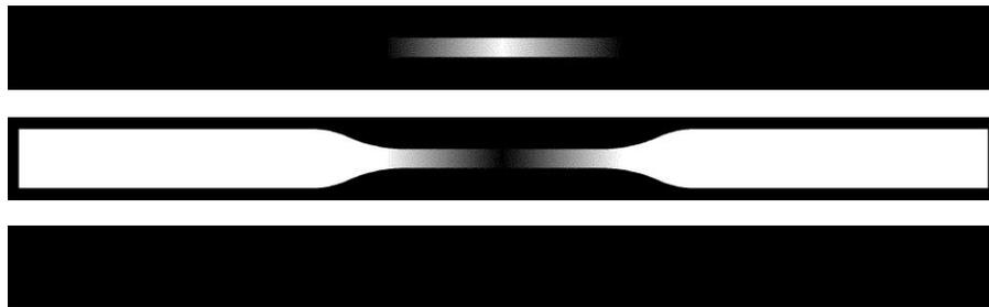
Figure 3-9: Examples of bitmap slices showing combined images of specimens with constant TB+ volume including material assignments for TB+ (top), VC (middle), and VeroZ (bottom) materials.
