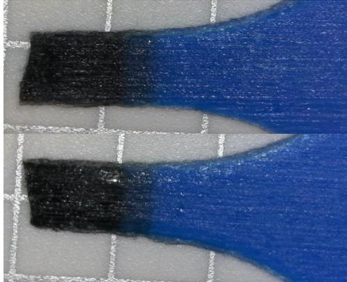
Figure 5-8: Tested fatigue specimens showing failure at the material interface for discrete gradient specimens with a constant TB+ length.
