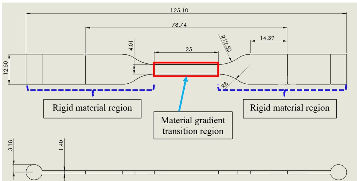
Figure 3-1: A CAD model of a specimen. All units are in millimeters.
