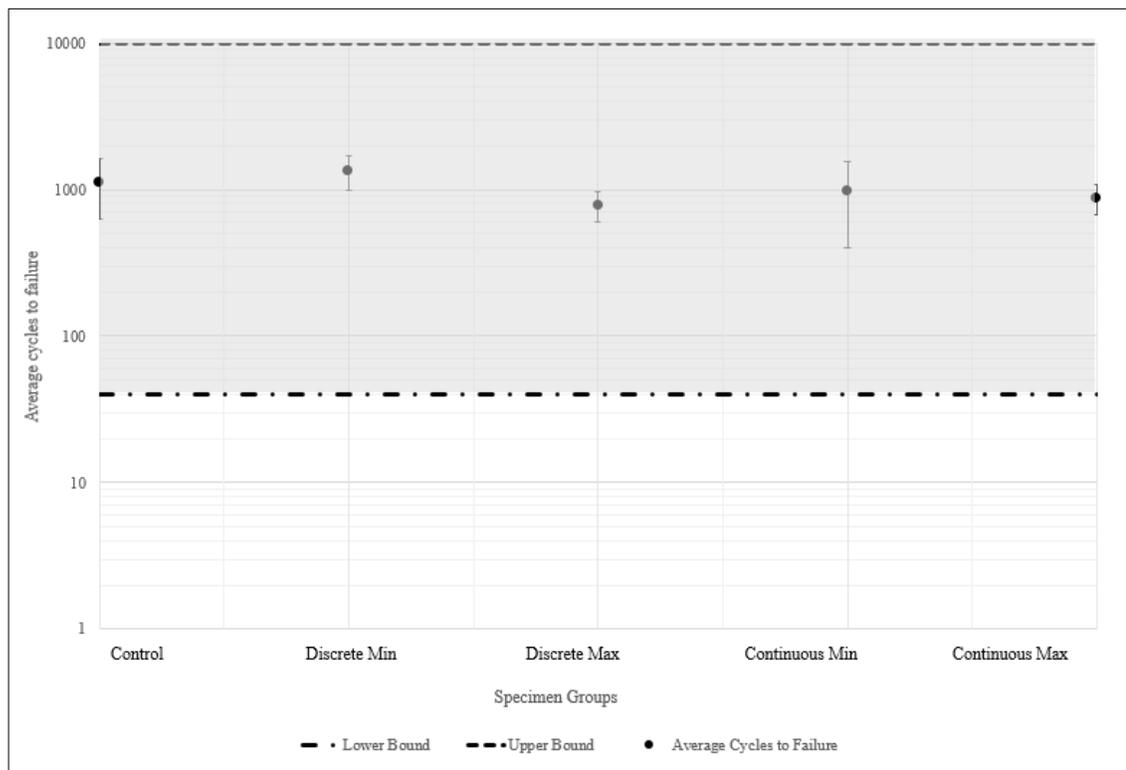
Figure 5-6: The average cycles to failure with the standard deviations as error bars for all specimen tested.
