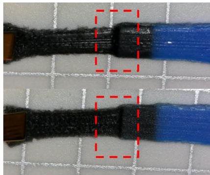
Figure 5-10: Tested fatigue specimens with discrete material gradients showing a step discontinuity in the material gradient transition region.
