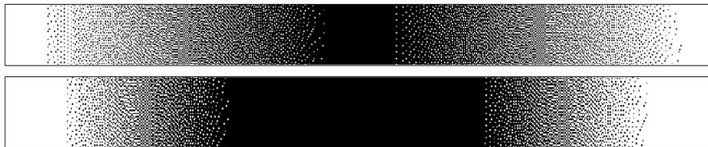
Figure 3-7: Dithered binary images showing a linear pattern of material transitions for specimens with a constant TB+ volume: max-length (top) and min-length (bottom).
