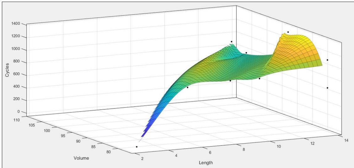
Figure 5-7: Graphical representation of all fatigue tested specimens relating the length of the region with 100% TB+, the overall volume, and the average number of cycles to failure.
