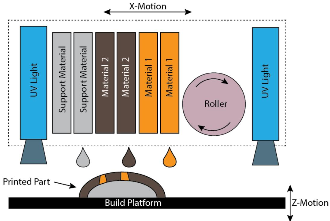
Figure 1-2: Schematic showing the material jetting printing process.
