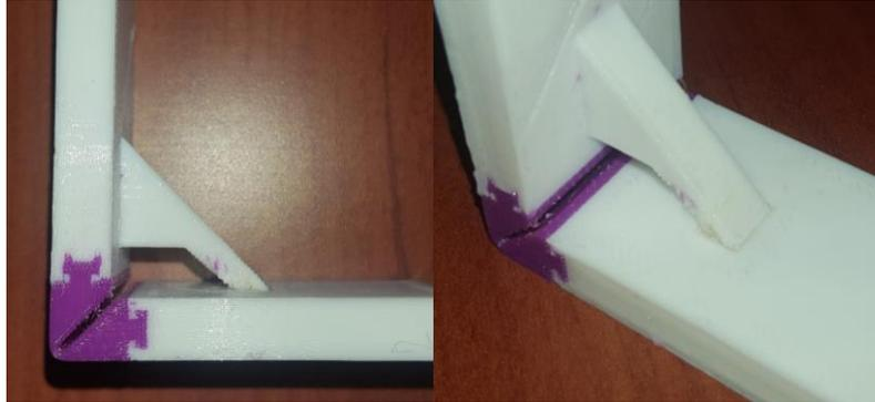
Figure 1-4: Example of a CAD model for a living hinge with a close-up view of the living hinge design.
