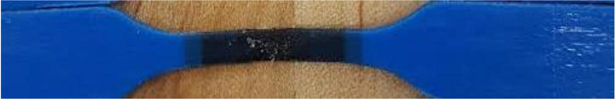
Figure 3-15: Printed specimen showing the discrete material gradient in the central region.
