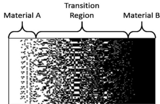
Figure 1-3: Example of a functionally graded structure with a gradient transition between material A and material B.
