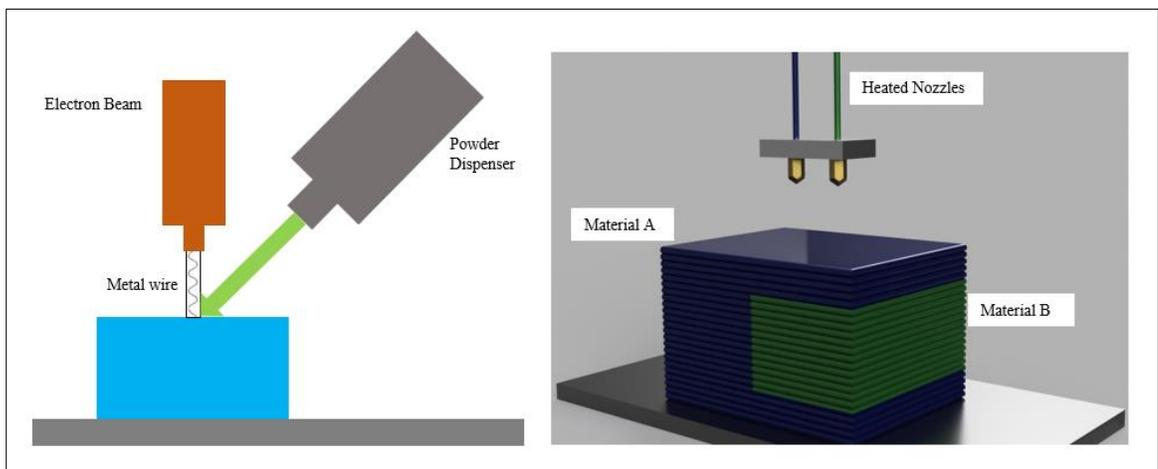
Figure 1-1: Schematics of the material extrusion (left) and the DED (right) processes.
