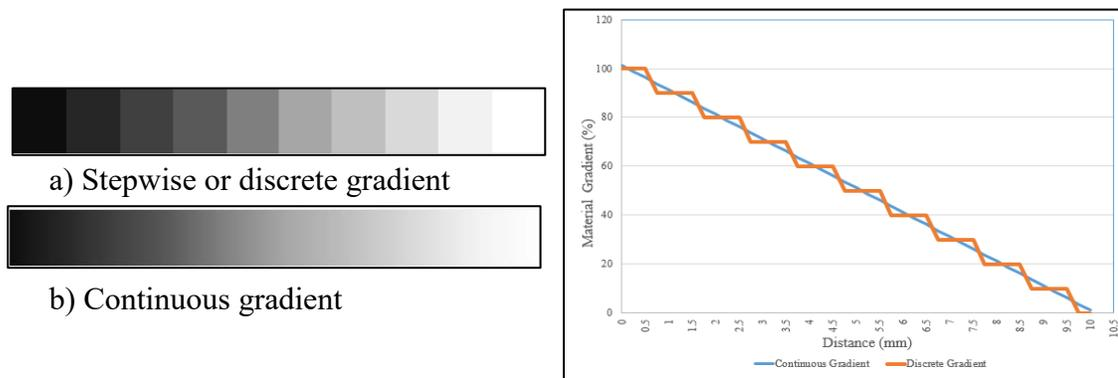
Figure 2-1: Stepwise or discrete gradients (a) and continuous gradients (b) with accompanying gradient plots.
