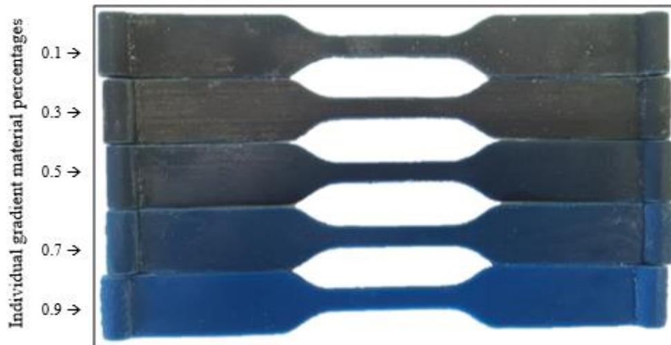
Figure 3-16: Printed specimens showing individual material composites with increasing percentages, from top to bottom, of the rigid material, VC.
