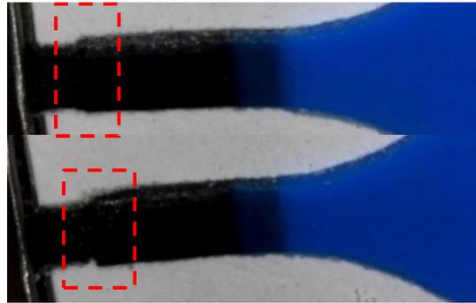
Figure 5-4: Tested fatigue specimens with discrete material gradients showing failure in the flexible, TB+, region and a step discontinuity in the transition region.
