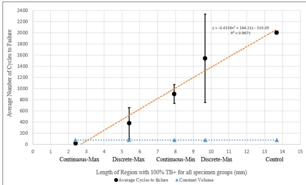
Figure 5-1: The average number of cycles to failure with the standard deviations error bars based on the regions with 100% TB+ for all specimens tested.
