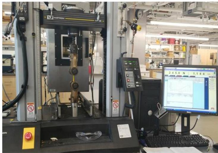
Figure 4-3: Tensile testing with the Instron 5866 Mechanical Testing System.
