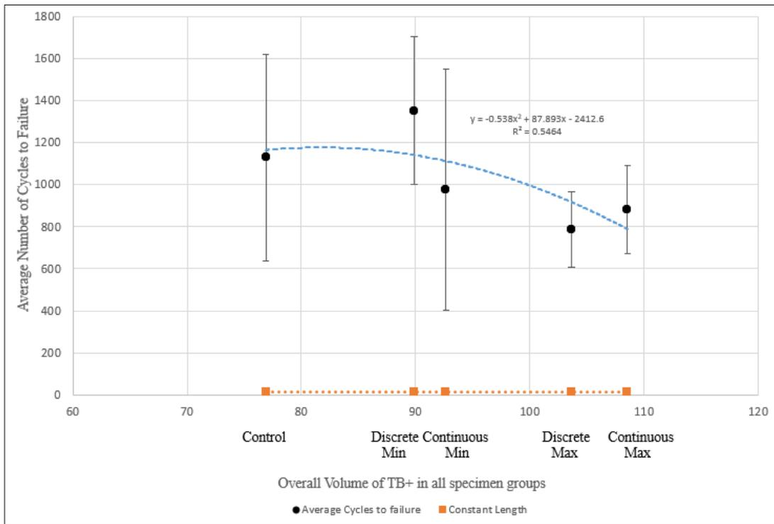
Figure 5-5: The average number of cycles to failure with the standard deviations error bars based on the overall volume of TB+ in all fatigue specimens tested.
