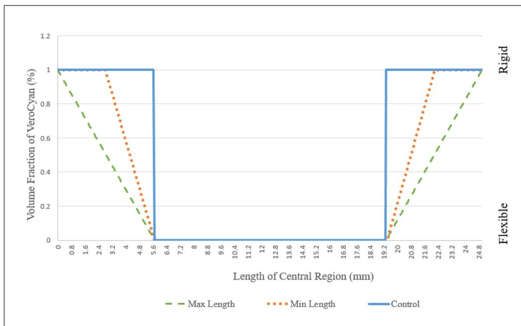
Figure 3-5: Plot showing the maximum and minimum material transition lengths in relation to the material transition of the control specimens for a constant TB+ length.
