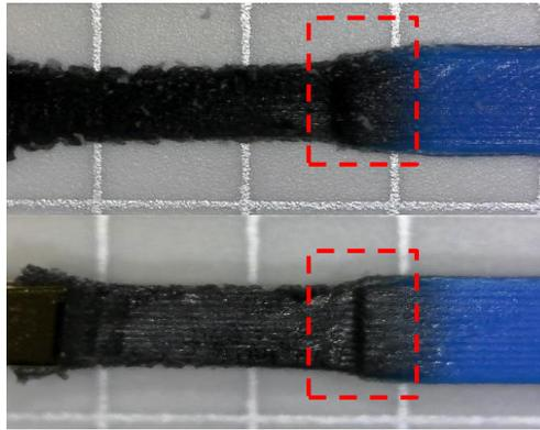
Figure 5-9: Tested fatigue specimens with continuous material gradients showing a step discontinuity in the material gradient transition region.
