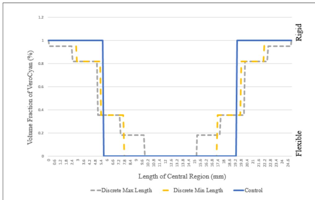
Figure 3-12: Plot showing the maximum and minimum lengths of the discrete material gradients in relation to the material transition of the control specimens for a constant TB+ volume.
