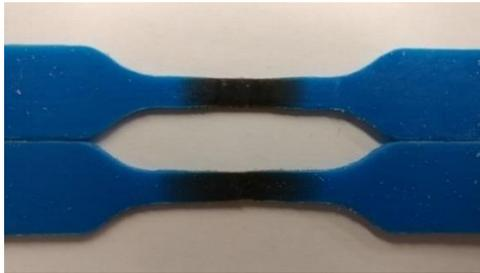
Figure 3-10: Printed specimens showing continuous material gradient applied to the central region: min-length (top) and max-length (bottom).
