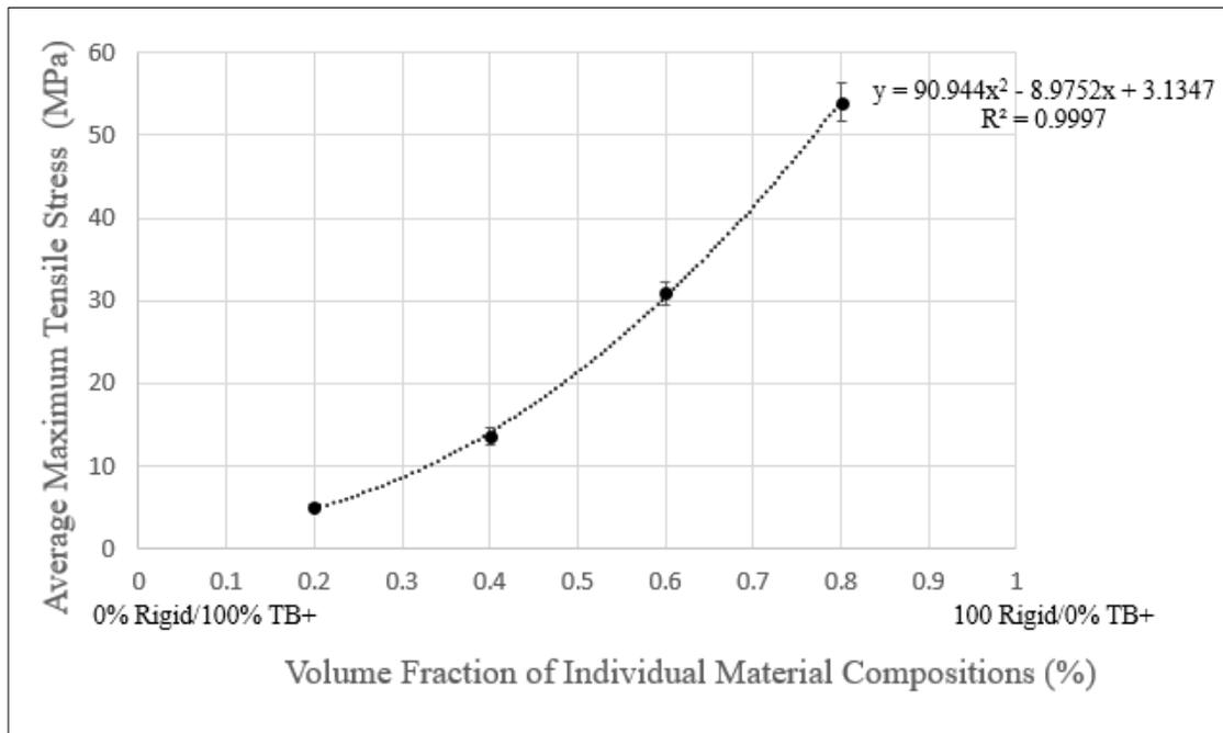
Figure 5-12: The average maximum tensile stress for each individual material composite.
