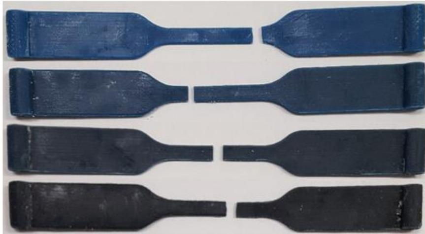
Figure 5-11: Tensile tested specimens with different individual material composites.
