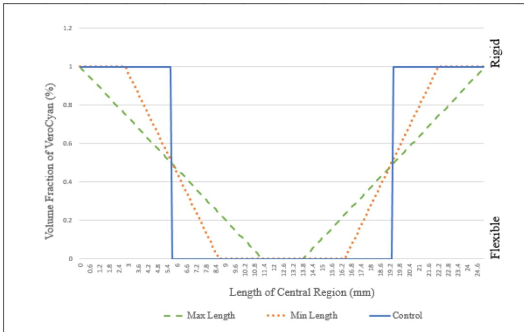
Figure 3-4: Plot showing the maximum and minimum material transition lengths in relation to the material transition of the control specimens for a constant TB+ volume.
