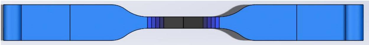
Figure 3-14: SolidWorks rendering of a CAD model with sections of discrete gradients.
