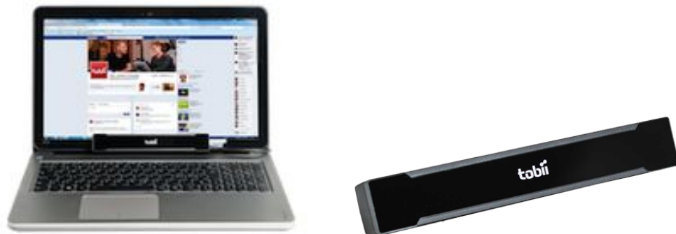
Figure 5- 1: Tobii X2-30 compact eye-tracker
