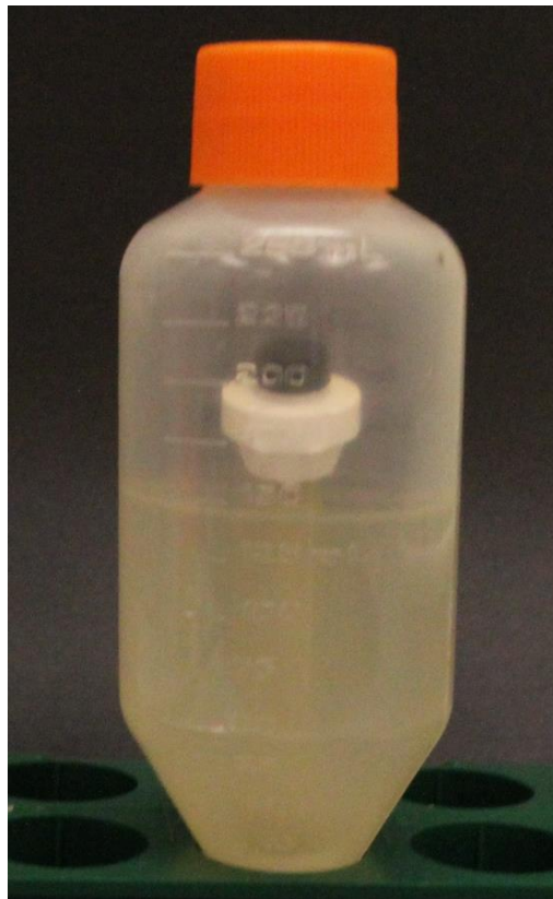
Figure 2-12. The flotation cell showing the illite-filled Float-A-Lyzer surrounded by the bulk phase mineral suspension.
