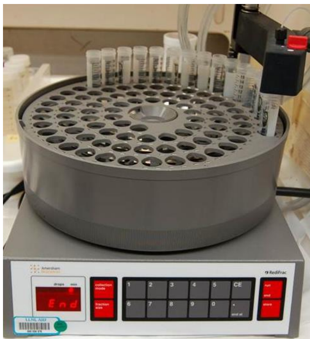
Figure 4-20. The Amersham Redifrac fraction collector that was used to collect eluted fractions from the automated chemical separation system.
