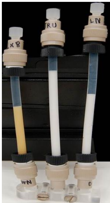
Figure 4-26. The three columns used in the automated chemical separation system. From L to R the AG 1x8 resin column, the TRU resin column and the LN resin column.
