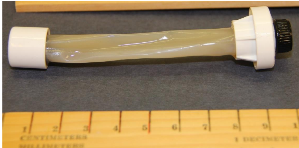
Figure 2-4. A picture of the Spectra/Por Float-A-Lyzer filled with illite mineral suspension before it was added to the flotation cell.
