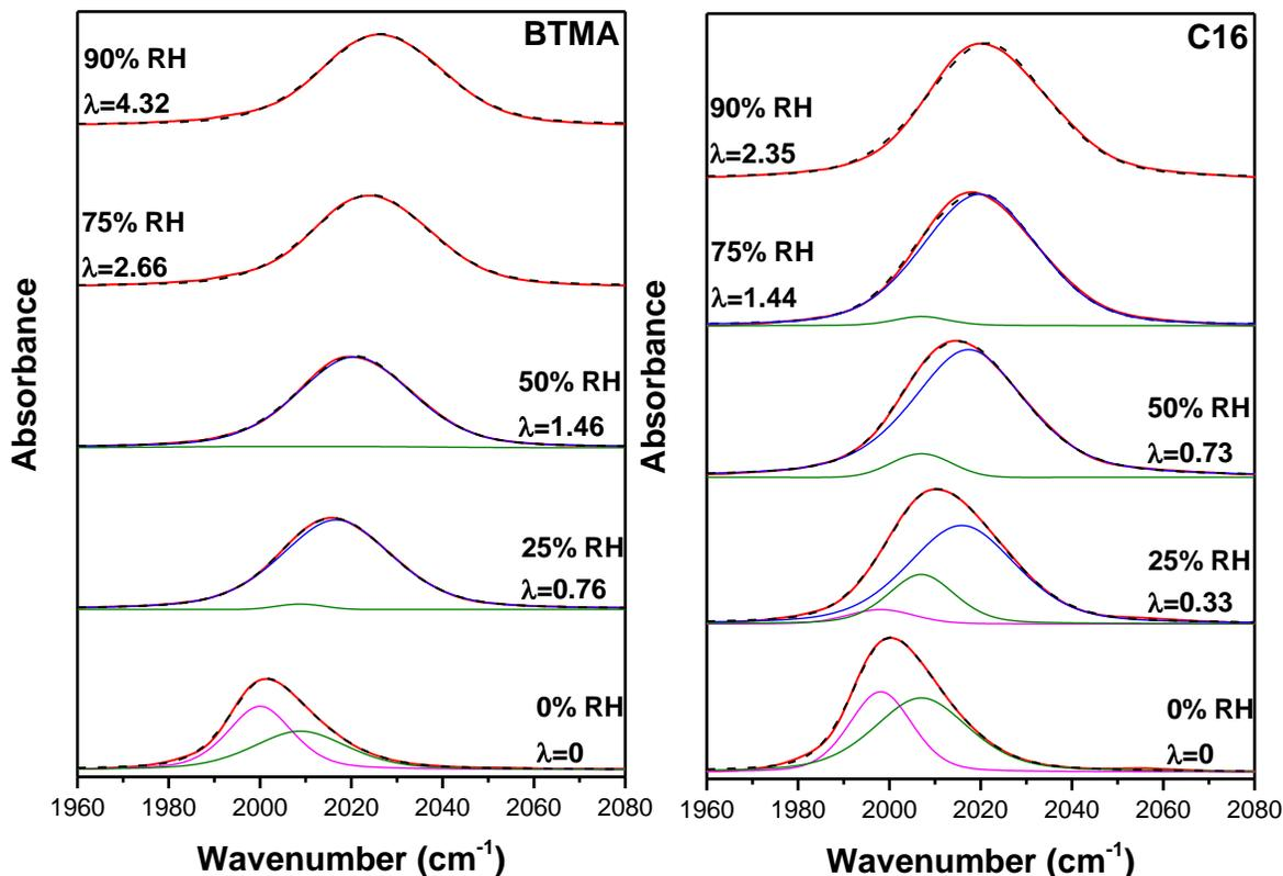
**Fig. 4.9** Deconvolution of all the comb-shaped polymers in the azide asymmetric stretch using the three-population model. Where the red is the experimental spectrum and the dashed black is the fitted spectrum. “wet” band is in blue, azide interacting with the QA is in green and the “free” azides is in magenta.
