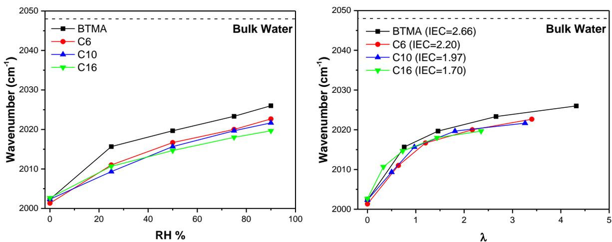
**Fig. 4.8** Changes in the azide asymmetric stretch frequency for all the samples as a a) function of RH and b) function of hydration number and the dashed line represent bulk water.
