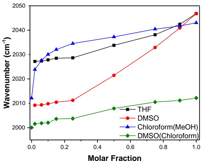
**Fig. 4.6** Representative summary of the azide solutions work done with DMSO-H<sub>2</sub>O, THF-H<sub>2</sub>O, Chloroform-Methanol and DMSO-Chloroform mixtures expressed as wavelength position vs. molar fraction.
