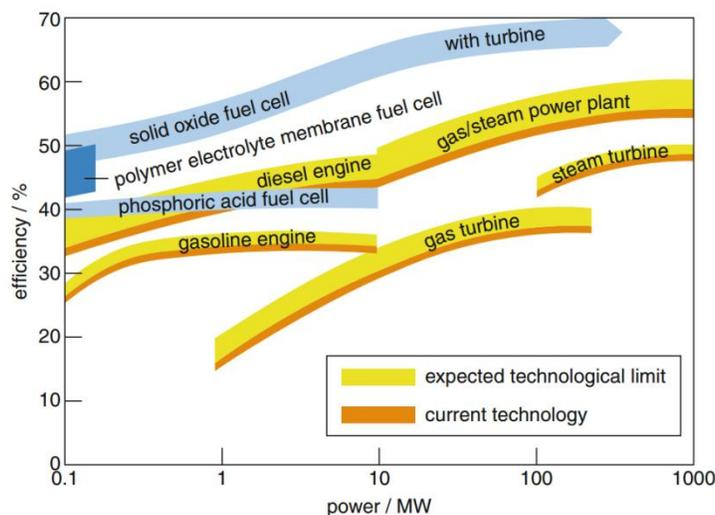
**Fig. 2.1** Efficiency vs. power for different fuel cell types compared to other energy technologies.<sup>1</sup>
