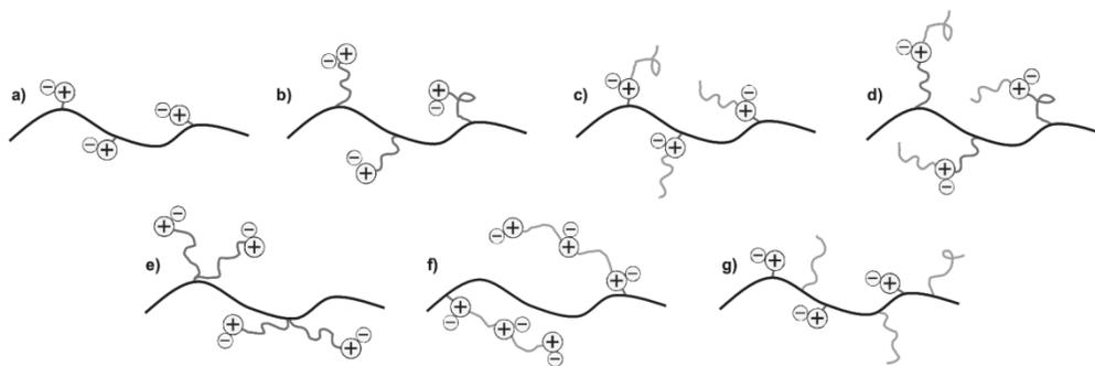
**Fig. 2.8** Different strategies to attach the cationic groups to the polymer backbone with side chains: a) directly on the backbone, b) via spacer chains, c) directly on the backbone with extender chains pendant to the cations, d) via spacer and extender chains, e) via spacer chains in pairs, f) multiple cations via connecting chains, and g) directly on the backbone with separate side chains.<sup>15</sup>
