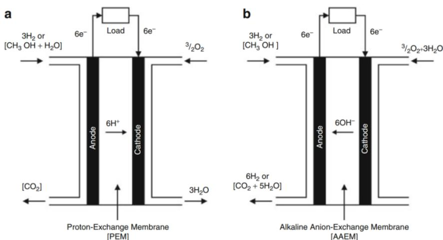
**Fig. 2.6** Schematic presentation of PEM(a) and AEM(b) both fueled with  $\text{H}_2$  gas or methanol. The stoichiometric ratios of reactants and products are shown.<sup>9</sup>
