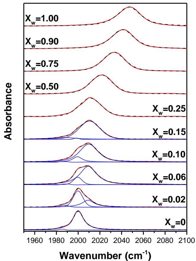
**Fig. 4.1** FTIR spectra of TBAN<sub>3</sub> in various mole fraction mixtures of water and DMSO. The red solid line represents the experimental spectrum. The black dashed line is the total fit. The blue lines are the individual components for the bands.
