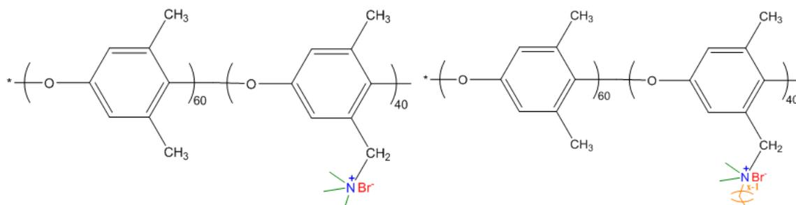
**Fig. 3.1** Chemical structure of the comb-shaped QA-PPO, where  $x$  = number of carbons in the *n*-alkyl side chain.
