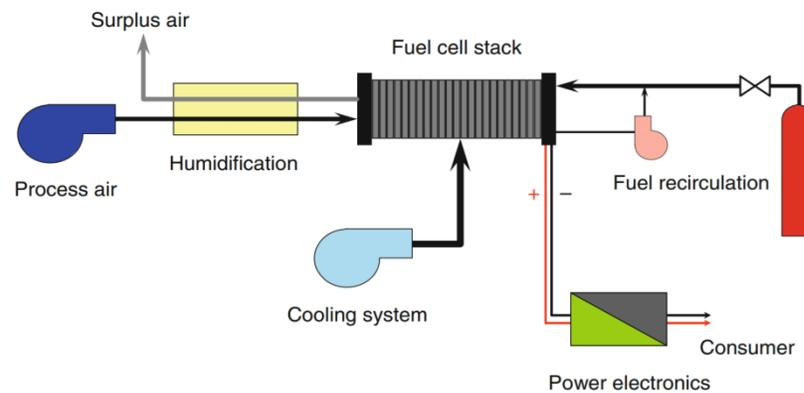
**Fig. 2.4** Simplified fuel cell system.<sup>4</sup>
