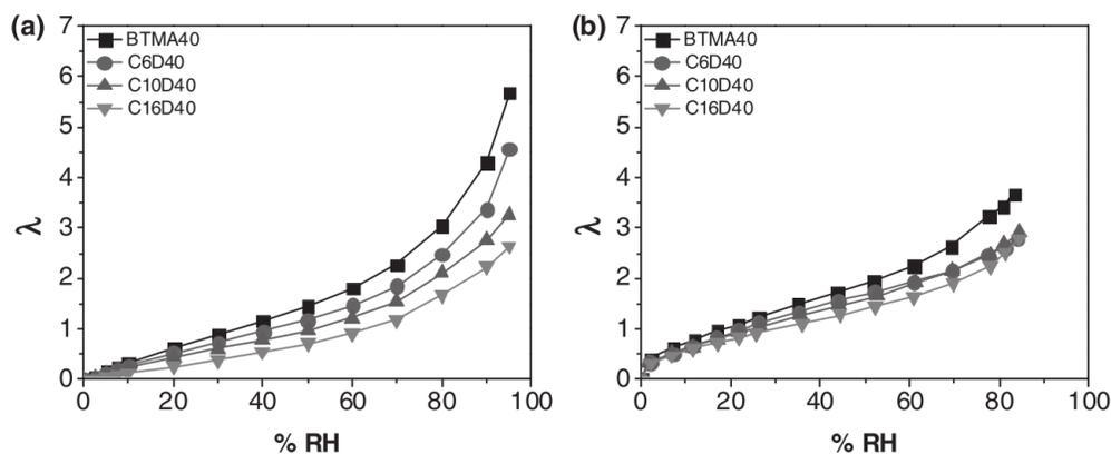
**Fig. 2.10** Hydration number as a function of % relative humidity (RH) for: a) bulk membrane and b) thin films.<sup>25</sup>
