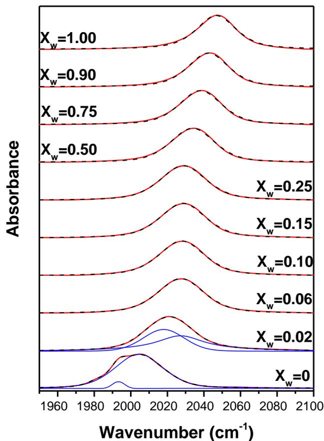
**Fig. 4.3** FTIR spectra of TBAN<sub>3</sub> in various mole fraction mixtures of water and THF. The red solid line represents the experimental spectrum. The black dashed line is the total fit. The blue lines are the individual components for the bands.
