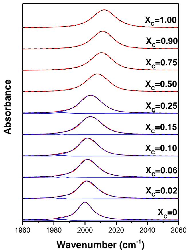
**Fig. 4.5** FTIR spectra of TBAN<sub>3</sub> in various mole fraction mixtures of DMSO and chloroform. The red solid line represents the experimental spectrum. The black dashed line is the total fit.
