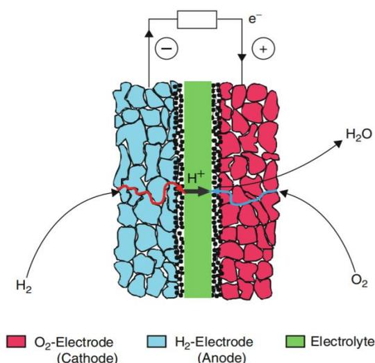
**Fig. 2.3** Simplified polymer electrolyte fuel cell (PEFC), showing only the porous gas diffusion electrodes and electrolyte, cell housing is not shown. Fuel:  $\text{H}_2$ , oxidant:  $\text{O}_2$ .<sup>4</sup>
