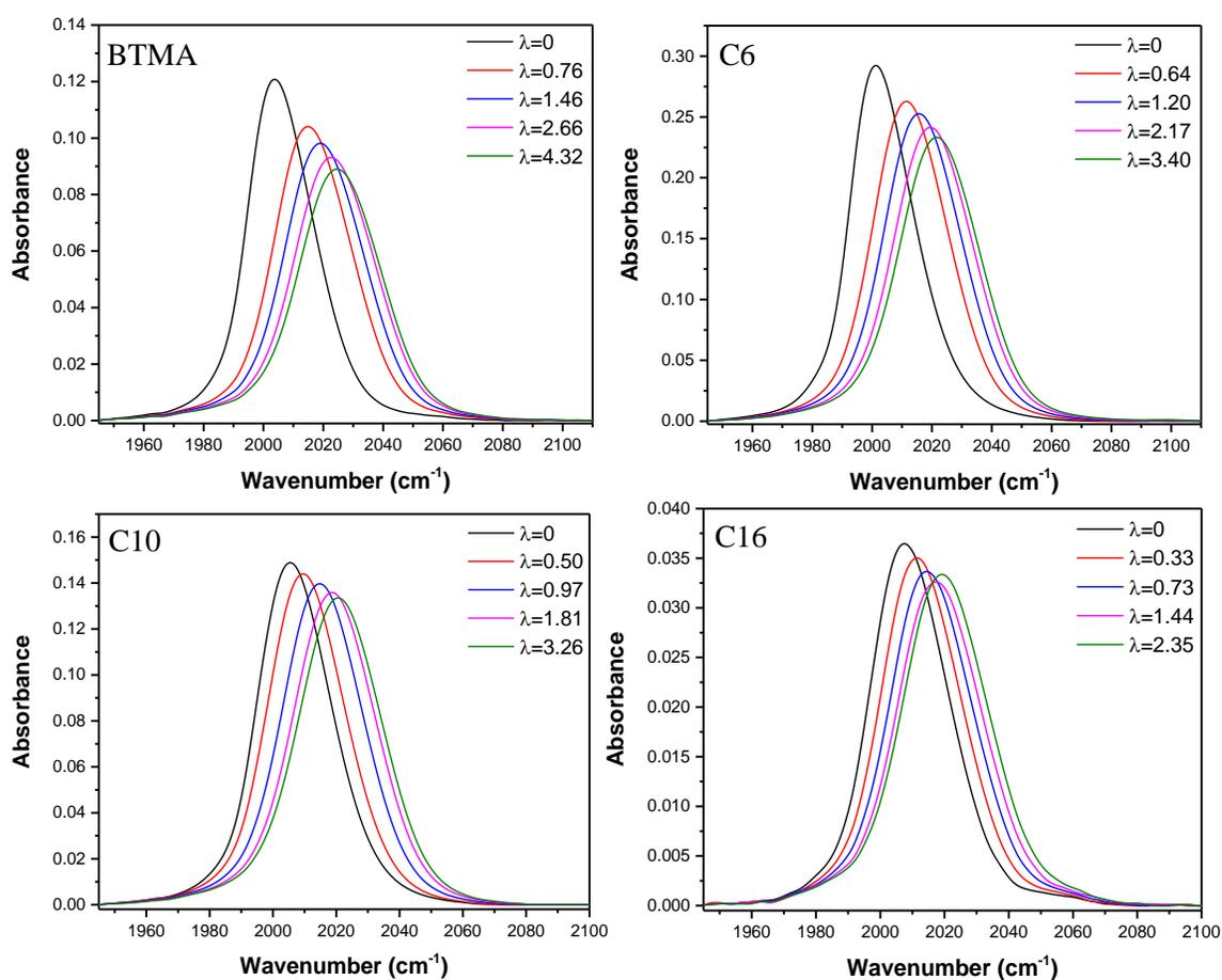
**Fig. 4.7** The azide asymmetric stretch in the different comb-shaped polymers.
