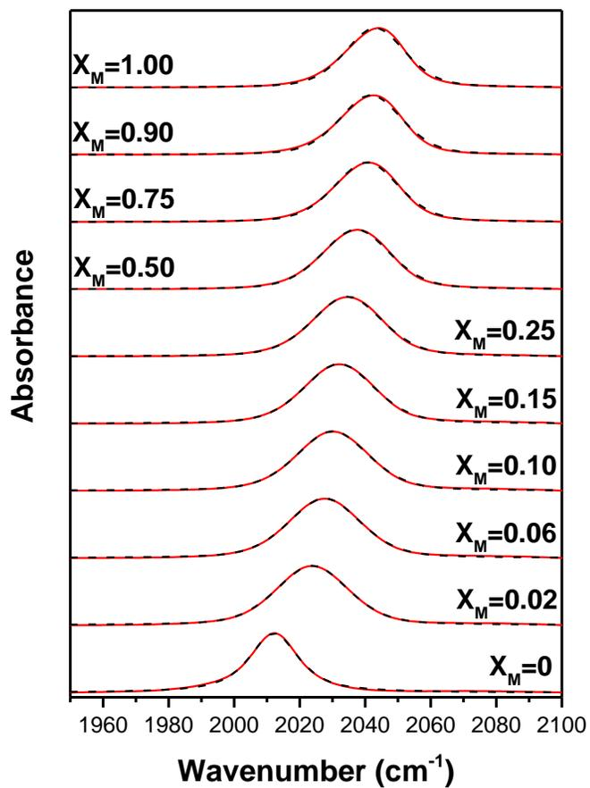
**Fig. 4.4** FTIR spectra of TBAN<sub>3</sub> in various mole fraction mixtures of chloroform and methanol. The red solid line represents the experimental spectrum. The black dashed line is the total fit.
