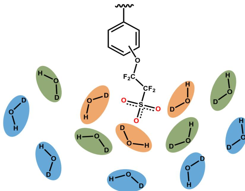
**Fig. 2.11** Schematic of the different populations of water absorbed into the polymer membrane. Blue represent bulk water, green intermediate water and orange the water bounded to the sulfonate group.<sup>41</sup>
