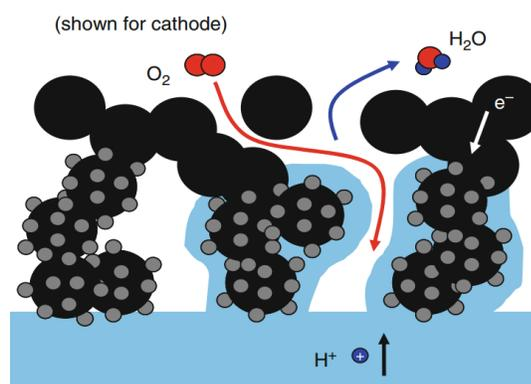
**Fig. 2.7** Electrode layer interphase with three phase boundary of a PEFC (cathode side). *Blue*: polymer electrolyte, *black*: carbon particles, *gray*: platinum nanoparticles.<sup>4</sup>
