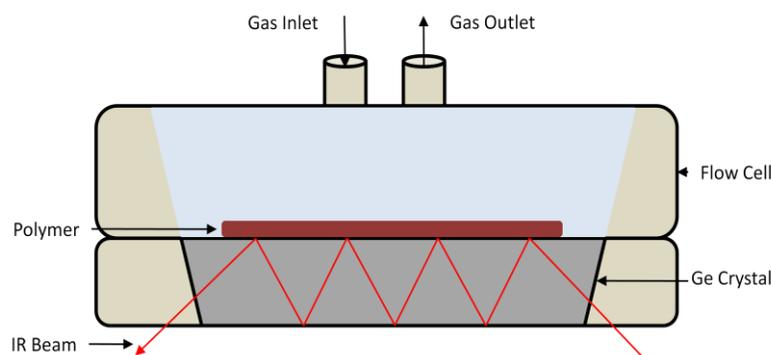
**Fig 3.3** Schematic of ATR flow cell used to introduce humidified air in the chamber containing the polymer sample while doing *in-situ* measurements.
