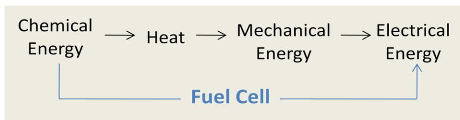
**Fig. 2.2** Schematic representation of direct energy conversion in an electrochemical cell as compared to thermal conversion in an internal combustion engine.<sup>4</sup>
