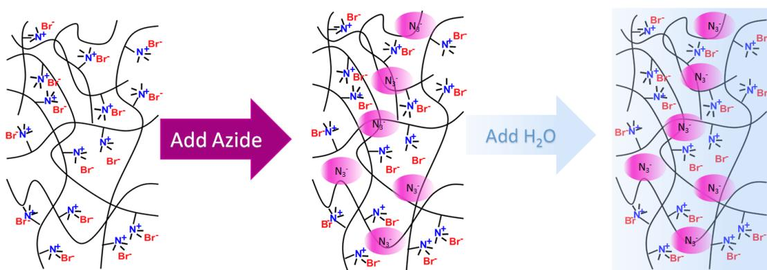
**Fig. 3.2** Schematic of the incorporation of azides ions into the polymer network and soaking procedure.
