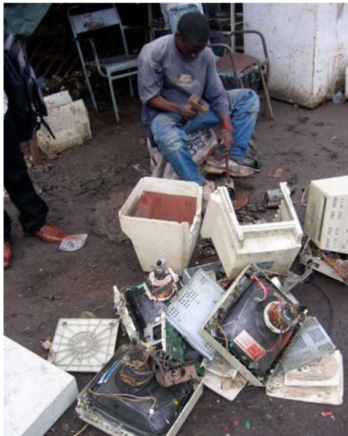
Figure 6: Disassembling CRTs at Agbogbloshie Scrap Market
