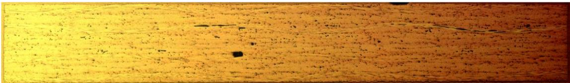
Figure 5-21. Initial microscopy cross section of specimen edge with unwanted brightness gradient
