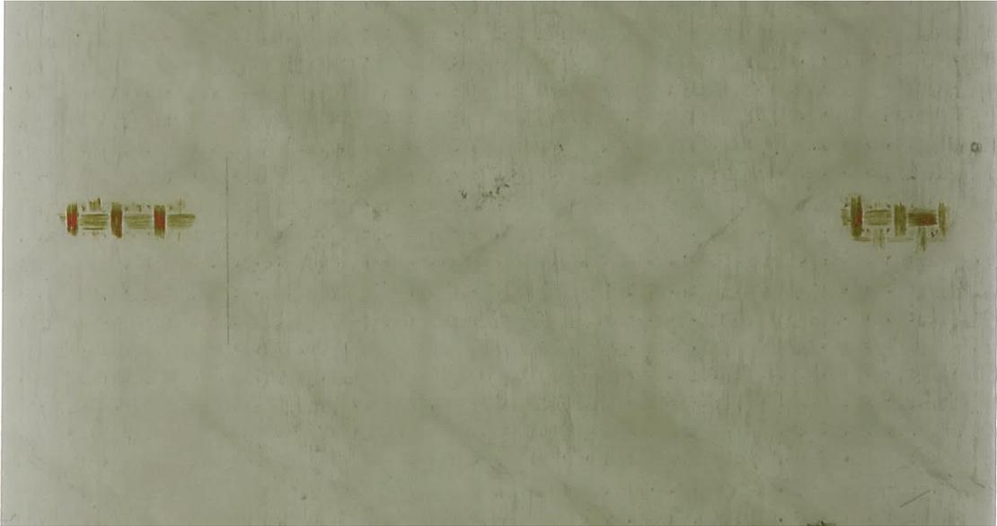
Figure 6-70. Scan of WET conditioned, but unloaded stitched sample without polysulfide edge seals
