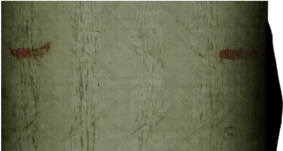
Figure 6-72. Scan of WET stitched sample tested to 13% modulus reduction at 13.75 ksi maximum
