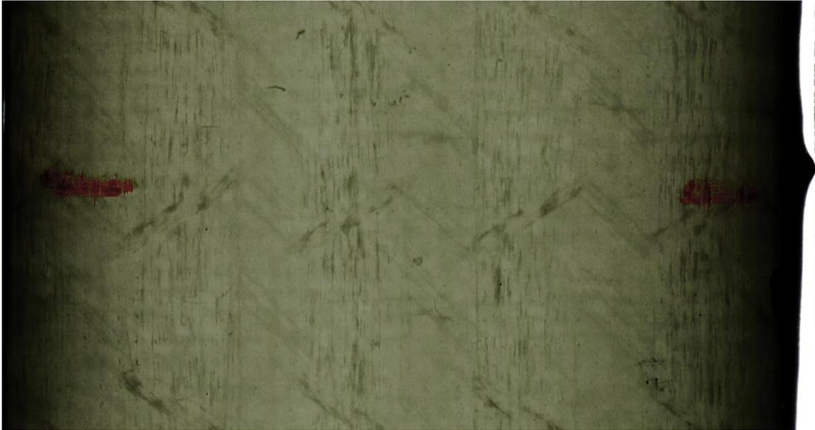
Figure 6-75. Scan of WET stitched sample tested to 16% modulus reduction at 13.75 ksi maximum
