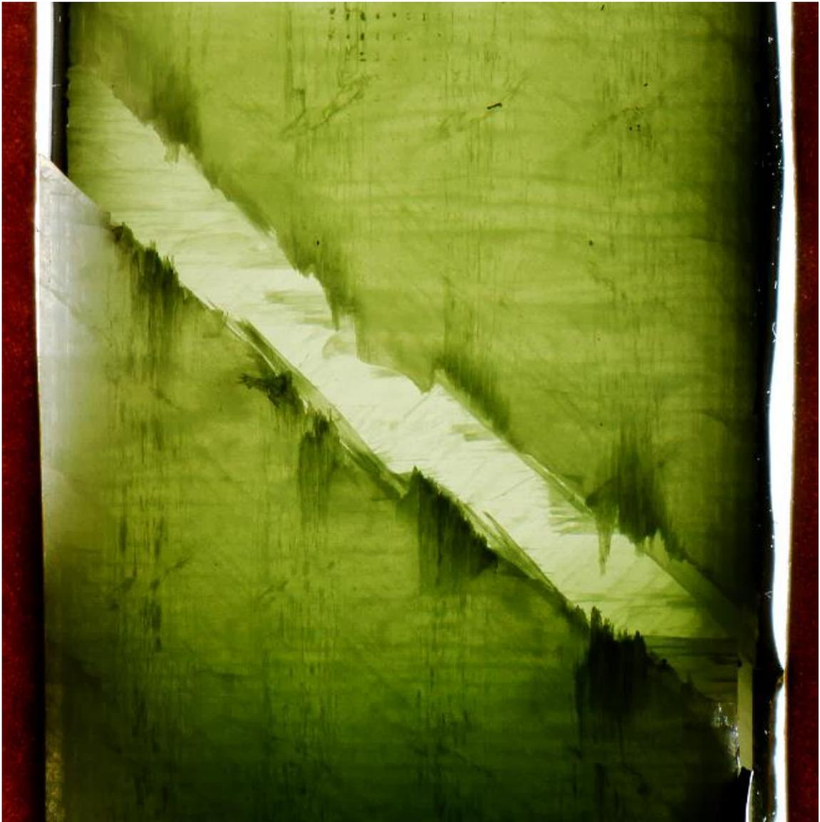
Figure 6-77. Scan of critical crack of WET stitched sample failed at 24 ksi maximum fatigue stress
