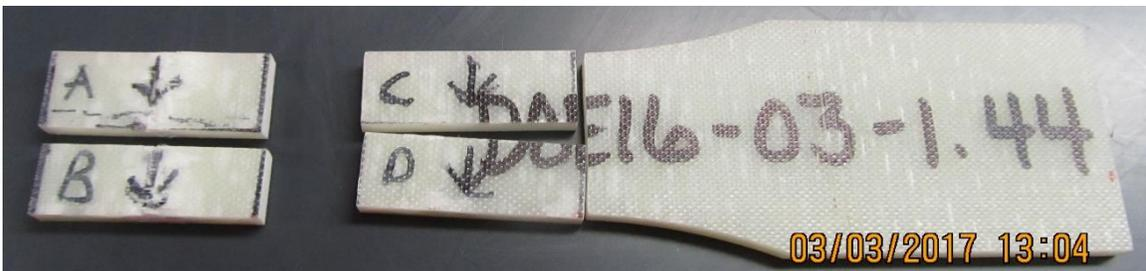
Figure 5-18. Longitudinal sections cut into four pieces.
