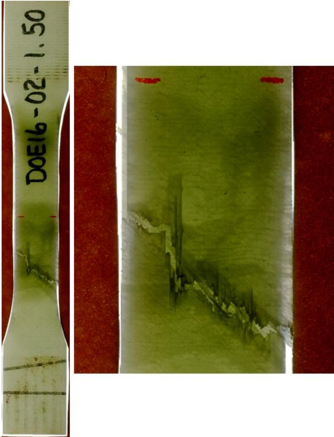
Figure 5-24. Example of scanned image with magnified image displaying macro cracks
