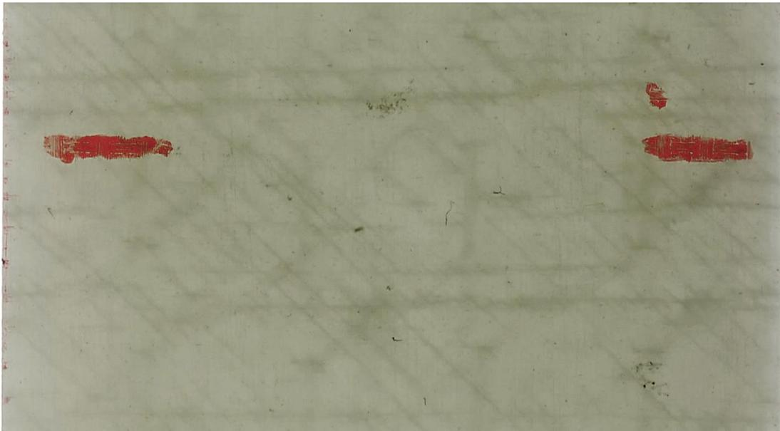
Figure 6-64. Scan of 13.75 ksi maximum stitched sample at nearly 13% modulus reduction
