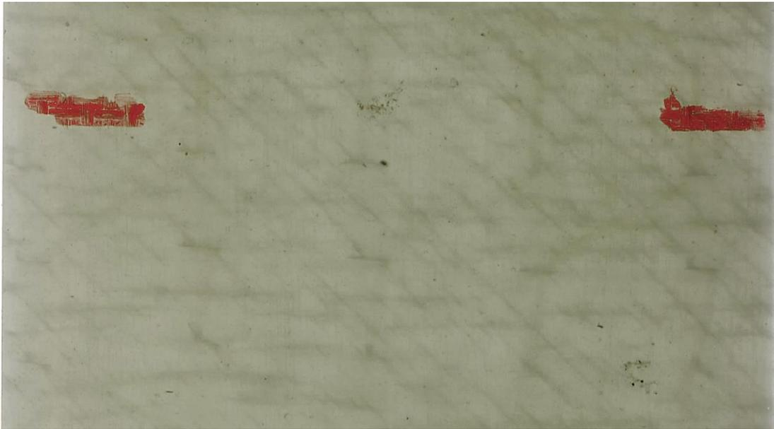
Figure 6-66. Scan of 18 ksi maximum stitched sample at nearly 13% modulus reduction
