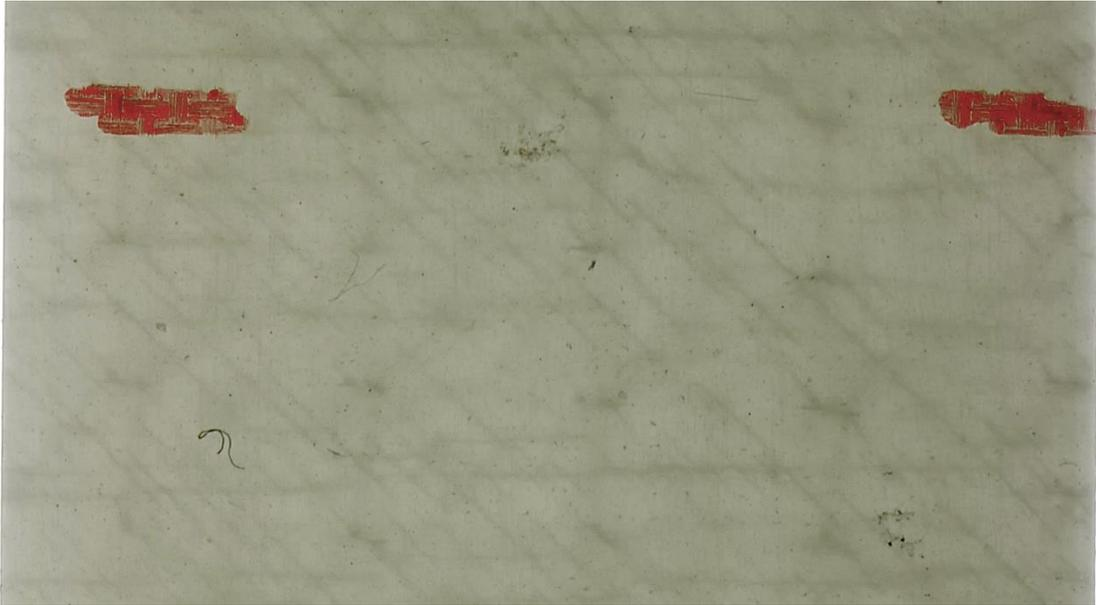
Figure 6-65. Scan of 13.75 ksi maximum stitched sample at nearly 16% modulus reduction
