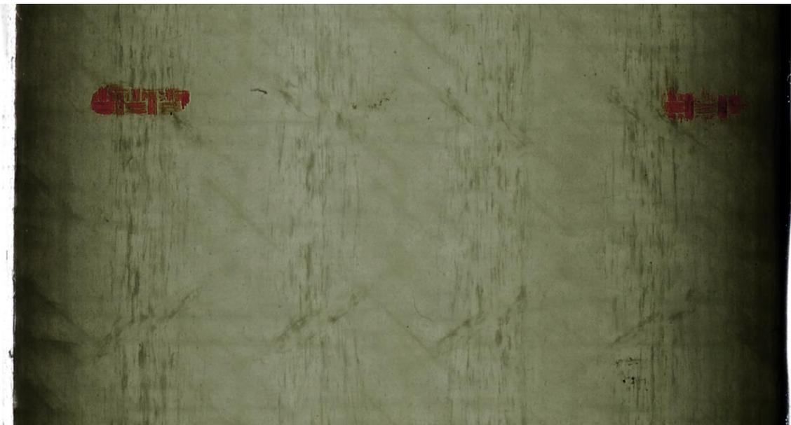
Figure 6-74. Scan of WET stitched sample tested to 10% modulus reduction at 18 ksi maximum
