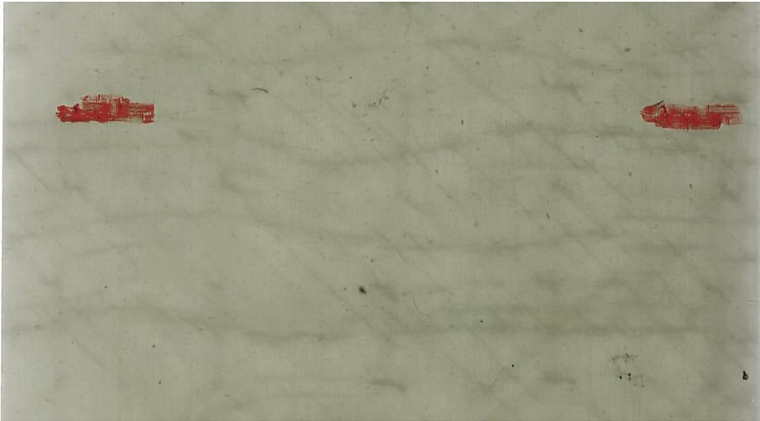
Figure 6-63. Scan of 13.75 ksi maximum stitched sample at nearly 10% modulus reduction
