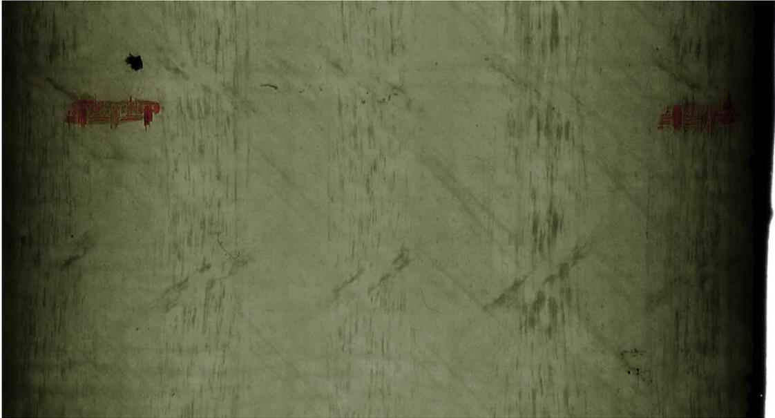
Figure 6-73. Scan of WET stitched sample tested to 16% modulus reduction at 13.75 ksi maximum
