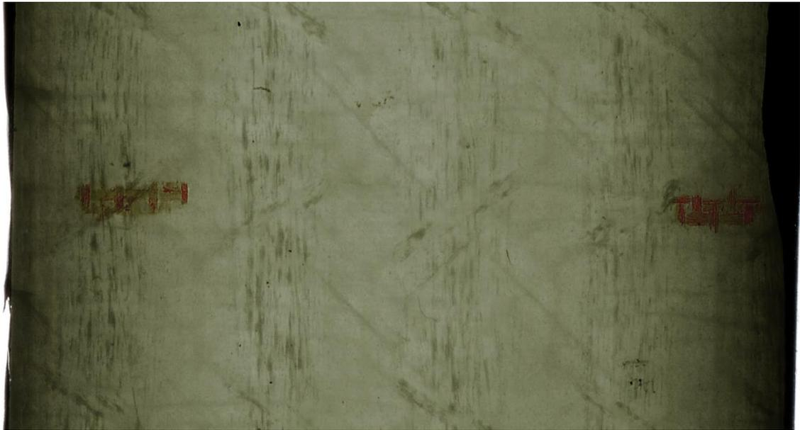
Figure 6-71. Scan of WET stitched sample tested to 10% modulus reduction at 13.75 ksi maximum
