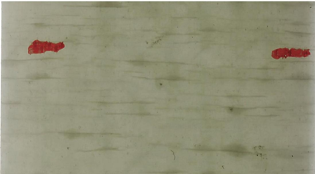
Figure 6-58. Scan of 18 ksi maximum woven sample at nearly 13% modulus reduction
