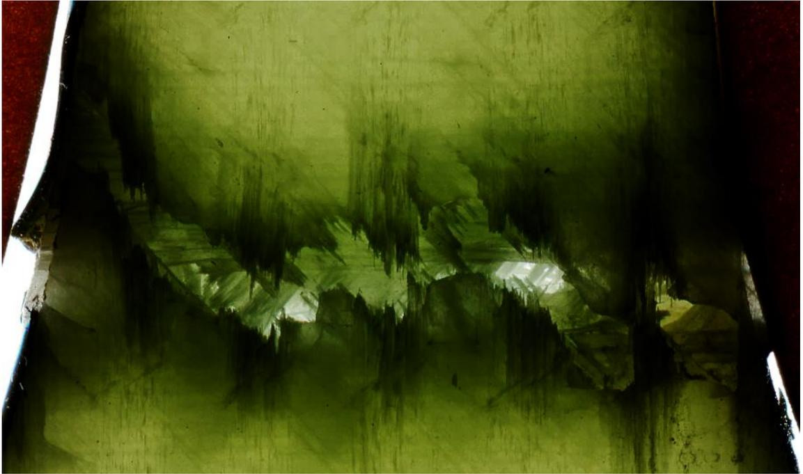
Figure 6-78. Scan of critical crack of WET stitched sample failed at 18 ksi maximum fatigue stress
