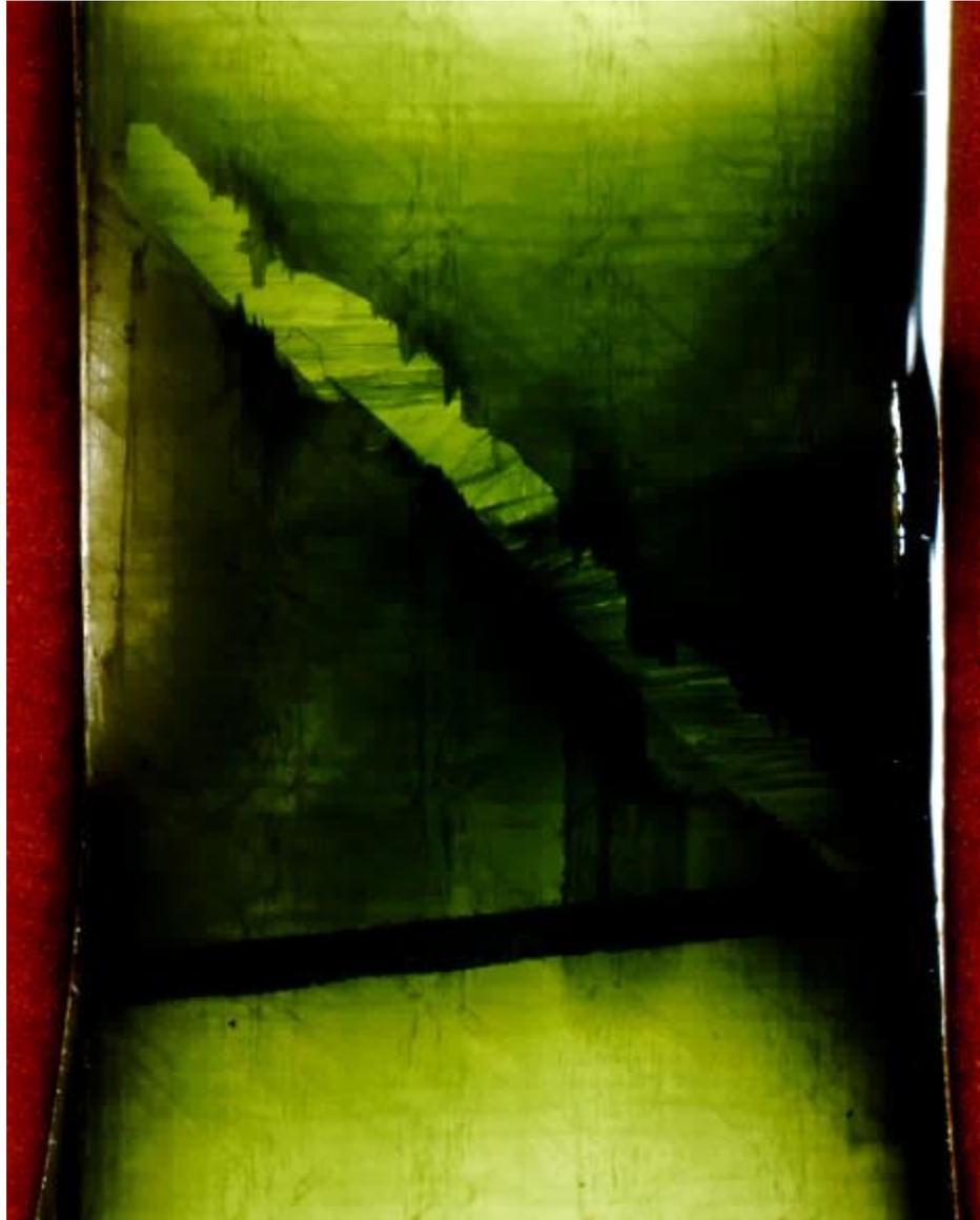
Figure 6-76. Scan of critical crack of WET stitched sample failed at 28.75 ksi maximum fatigue stress
