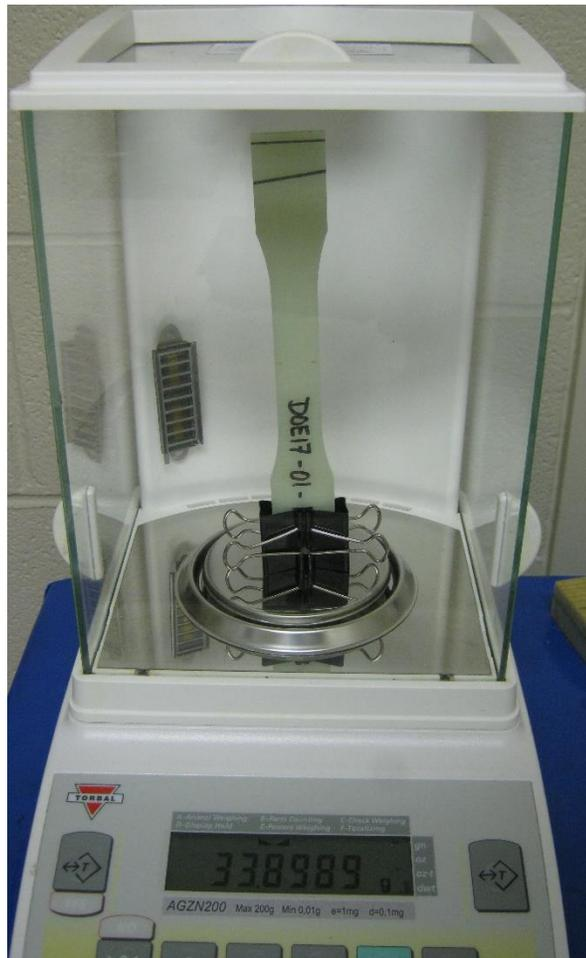
Figure 5-8. Dogbone specimen weight measurement procedure including binder clips
