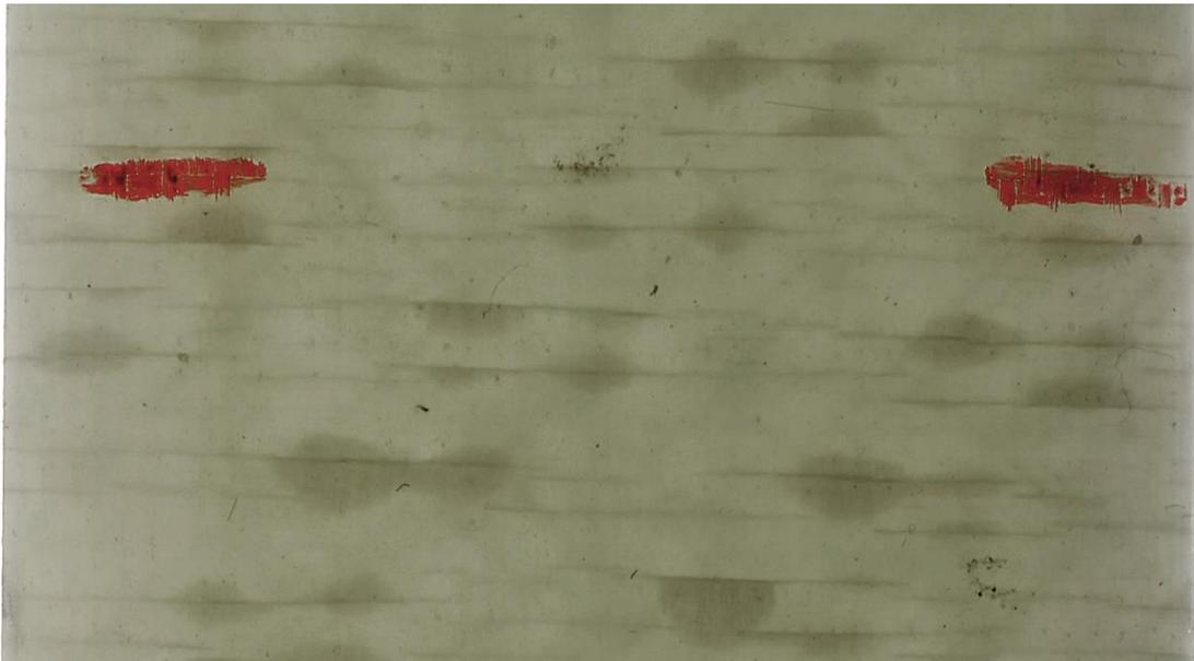
Figure 6-57. Scan of 13.75 ksi maximum woven sample at nearly 16% modulus reduction
