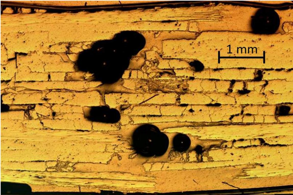
Figure 6-52. Critical flaw within 18 ksi maximum failed sample complete with delaminations of nearly every ply and numerous interlaminar cracks
