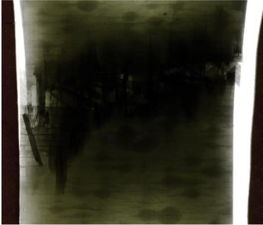
Figure 6-60. Scan of critical crack of woven sample failed at 24 ksi maximum fatigue stress
