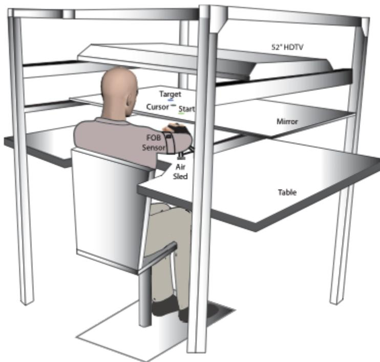
Figure 2. Target reaching and training apparatus.
