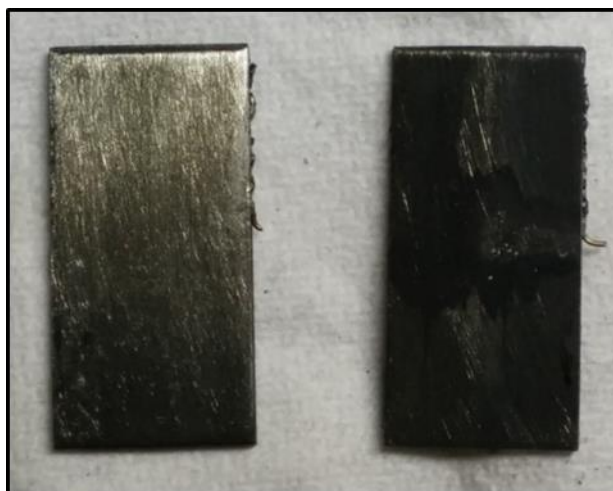
Figure 4-15. Stainless steel samples post testing under caustic treatment. On the left: Sample CT-2 Test solution: \text{pH}_{25^\circ\text{C}} = 9.3 using \text{NH}_4\text{OH} + 0.5 \text{ ppm NaOH} . On the right: Sample CT-1 Test solution: \text{pH}_{25^\circ\text{C}} = 9.3 using \text{NH}_4\text{OH} + 1.2 \text{ ppm NaOH} . Exposure time = 65 hours. Temperature 300^\circ\text{C} .
