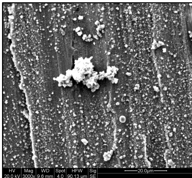
Figure 4-55. Secondary Electron Image (3000x) of the sample AVTPS showing a cluster of particles in a region with deposits. The clusters are agglomerates of smaller particles. Test solution is \text{pH}_{25\text{ }^{\circ}\text{C}} = 9.3 \text{ NH}_4\text{OH(aq)} . Test B: Particle size distribution < 5\mu\text{m} . Exposure time = 65 hours. Temperature 300\text{ }^{\circ}\text{C} .
