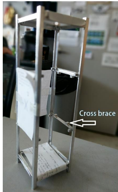
Figure 5-4. Structure of OSIRIS, the 3U CubeSat, showing the cross-brace structure that is to be designed.
