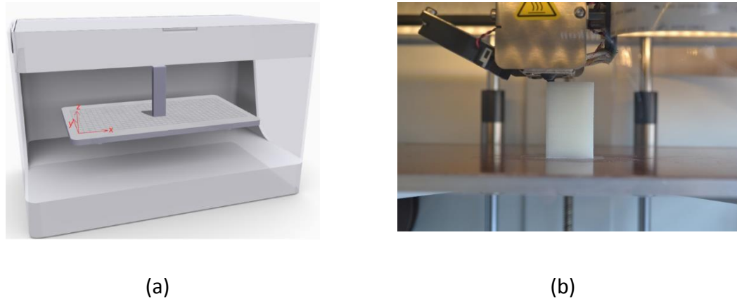
Figure 3-1. Build orientation of the specimen on Mark One and (b) Mark One while printing the specimen.
