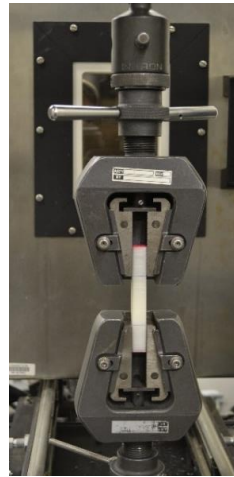
Figure 4-1. Tensile testing on Instron 5866 Mechanical Testing Machine.
