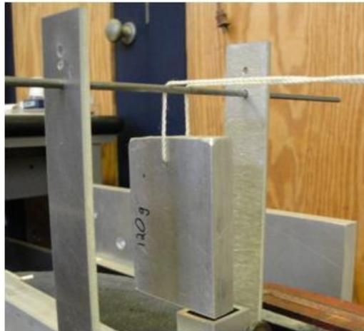
Figure 3-7: Hanging Mass Representing Centrifugal Force. Different masses indicate different values of centrifugal force.
