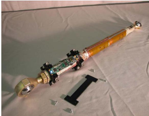
Figure 1-10: MicroStrain's © Piezoelectric Pitch Link Energy Harvester System Used to Monitor Pitch Link Loads.
