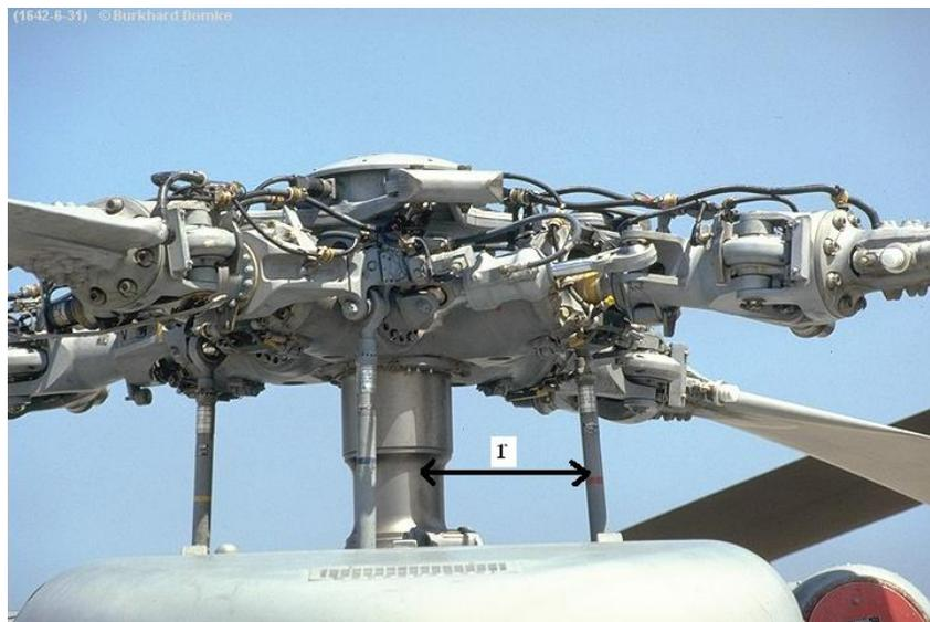
Figure 2-6: Pitch Link Location on the HUB.  $r$  is the distance from the main rotor shaft to the pitch link.
