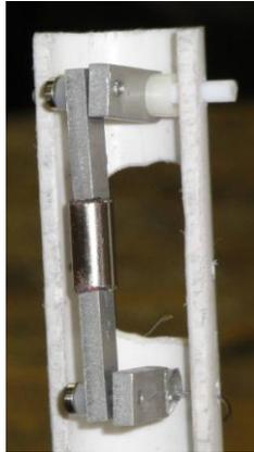
Figure 3-11: Photo of Linear Reverse Pendulum Harvester. The magnet was attached with spring pins. The top back hinge is a Teflon rod and the other two hinges are shoulder bolts. Plastic spacers were used to keep the device in line
