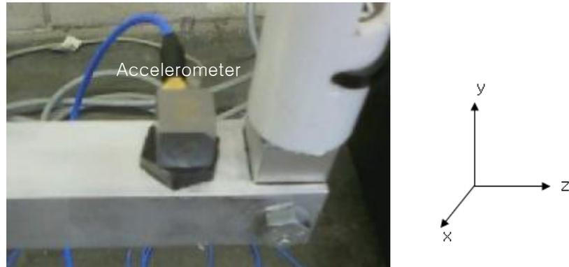
Figure 3-3: Tri-axial Accelerometer to Monitor Base Motion System. The accelerometer measures vibrations in three directions ensuring that the base motion system produces accelerations that mimic a pitch link in flight
