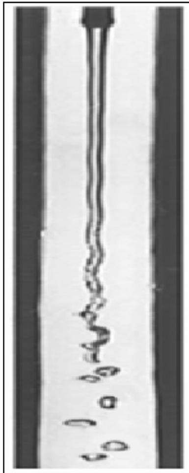
Figure 3-3: Photographic example of a turbulent liquid jet
