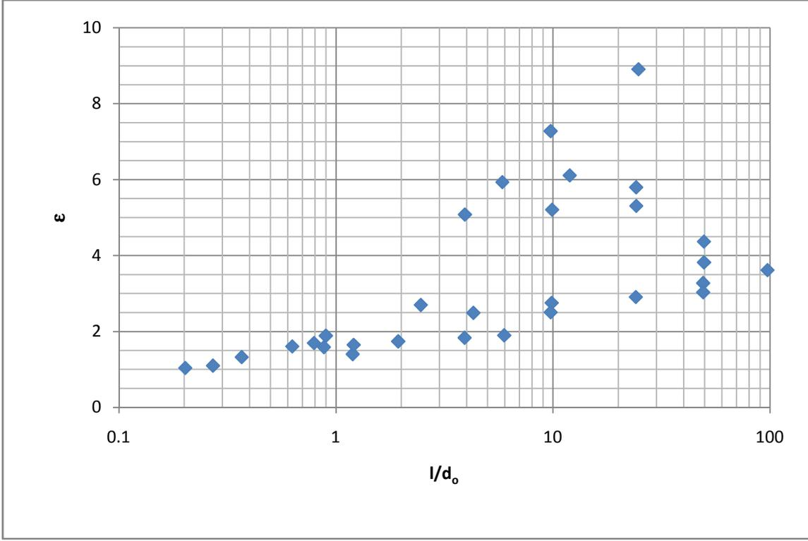
Figure 3-8: Ellipsicity of droplets based upon the normalized streamwise distance from the nozzle for turbulent jets in the wind-induced regimes [57].
