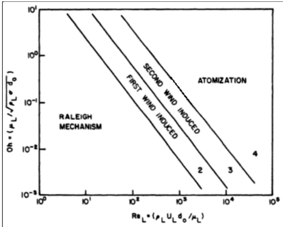
Figure 2-4: Modes of jet disintegration [24].
