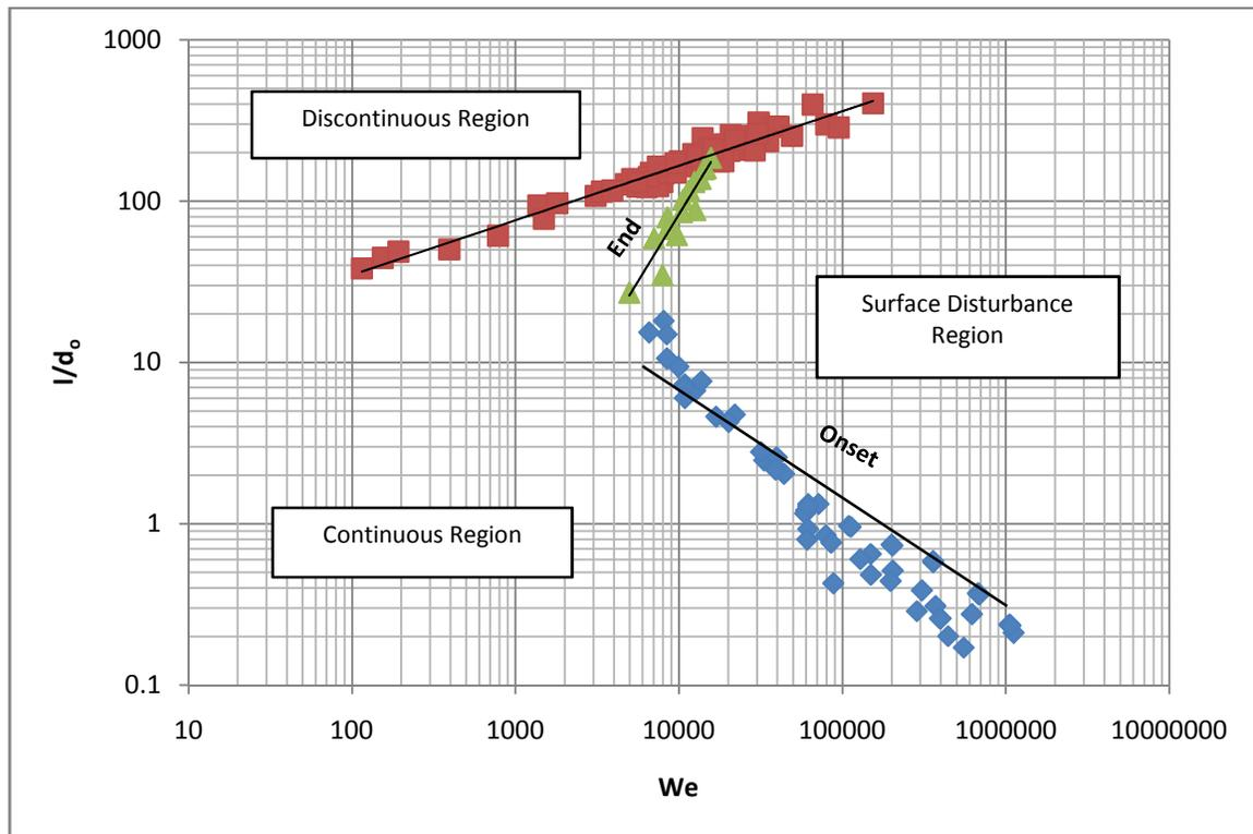
Figure 3-4: Disintegration data and characteristic lengths
