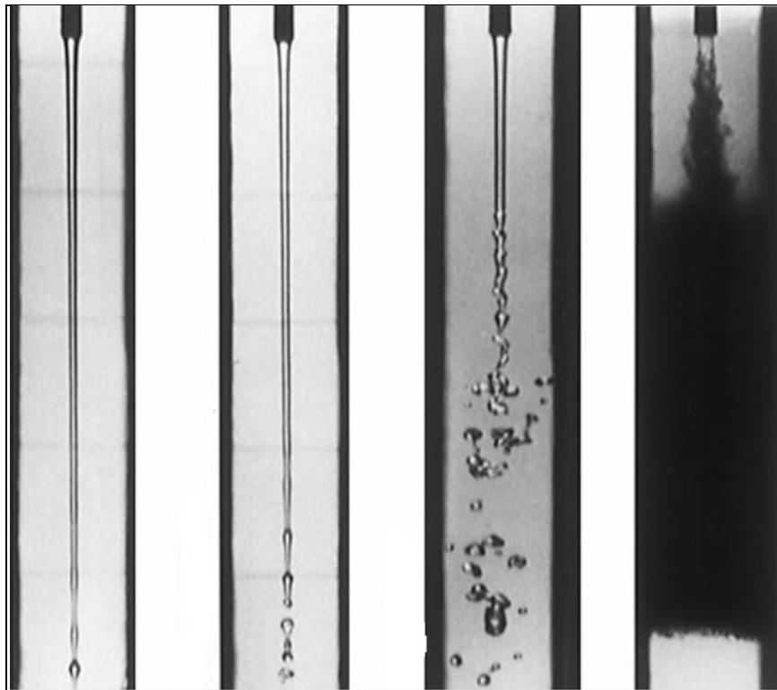
Figure 1-1: Multiple modes of liquid jet disintegration [21].
