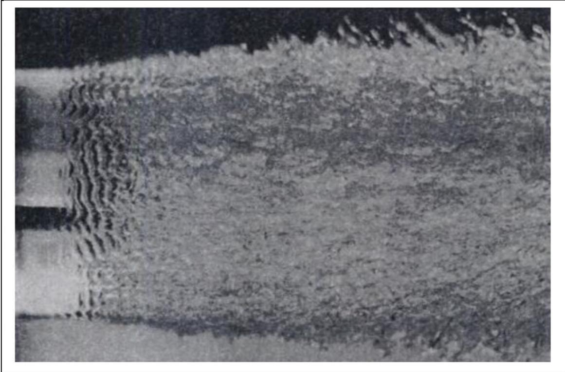
Figure 2-12: Enlarged view of a turbulent water jet [24].
