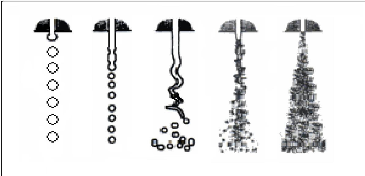
Figure 2-5: Illustration of jet disintegration modes [26].
