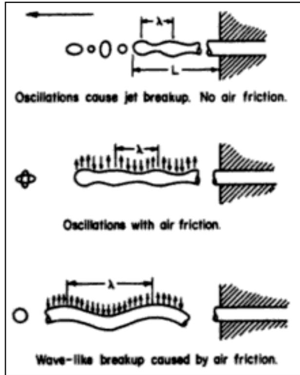
Figure 2-1: Mechanisms of drop formation [14].
