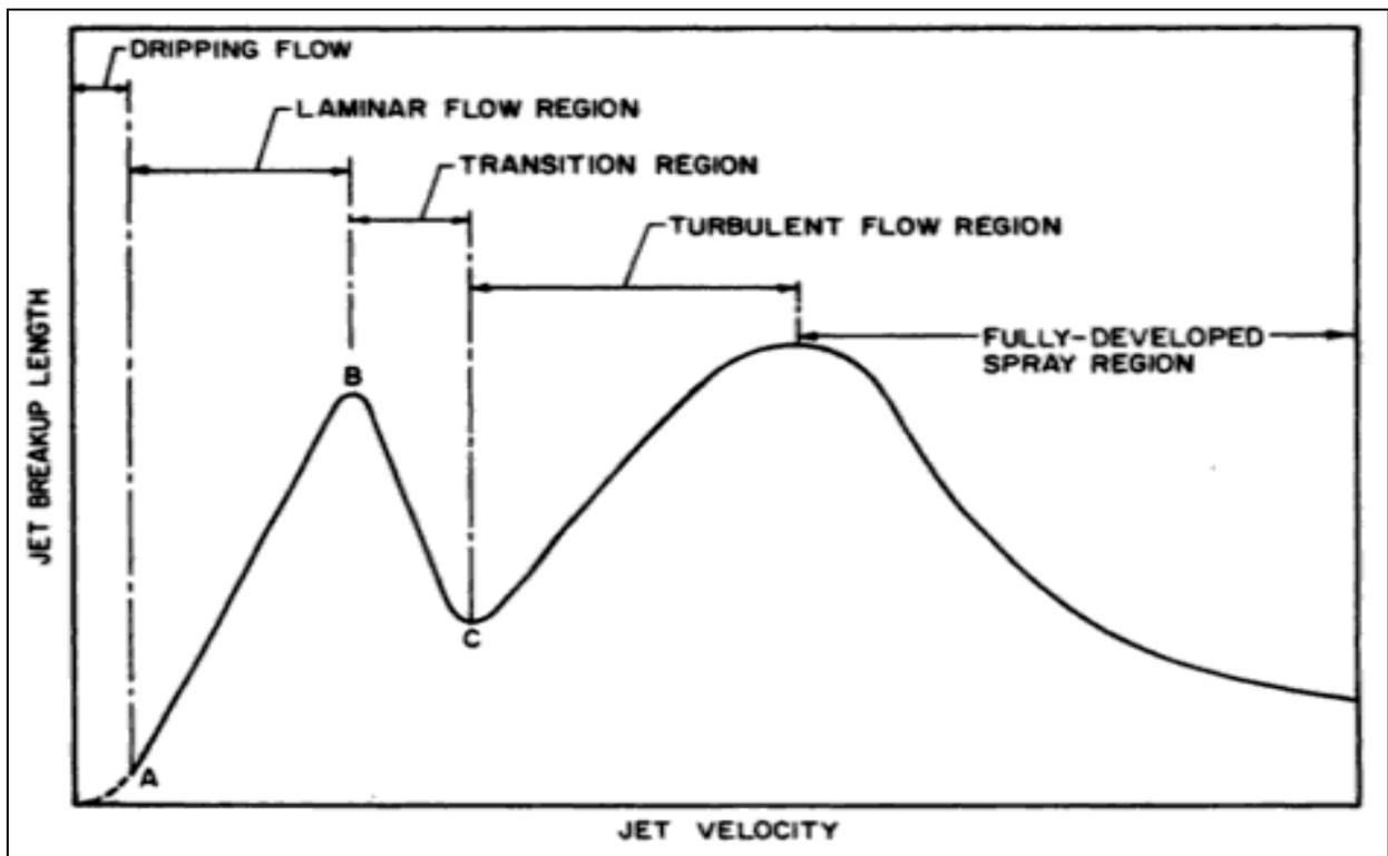
Figure 2-9: Illustration of jet stability with regard to velocity [24].
