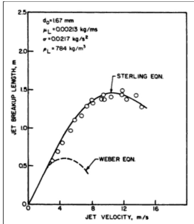
Figure 2-11: Comparison of experimental data with analytical predictions using the results of Weber and Mahoney and Sterling [24].
