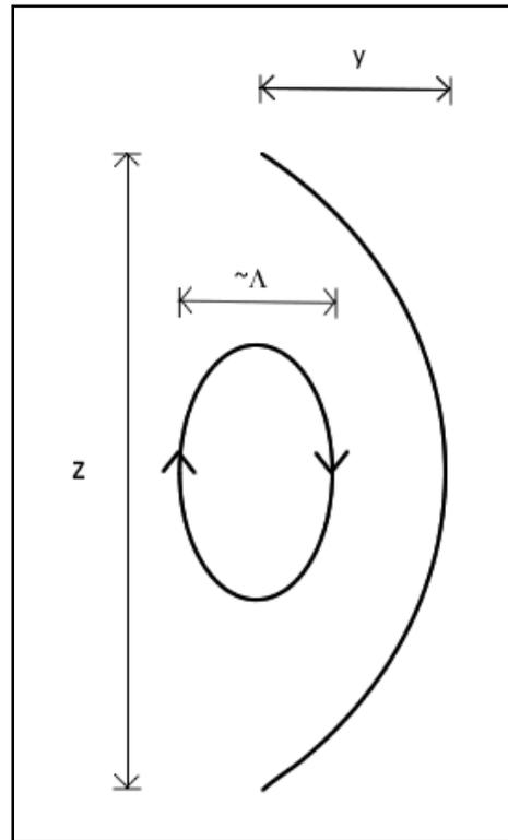
Figure 3-7: Depiction of a turbulent eddy and surface disturbance for a turbulent liquid jet in the FWI breakup regime.
