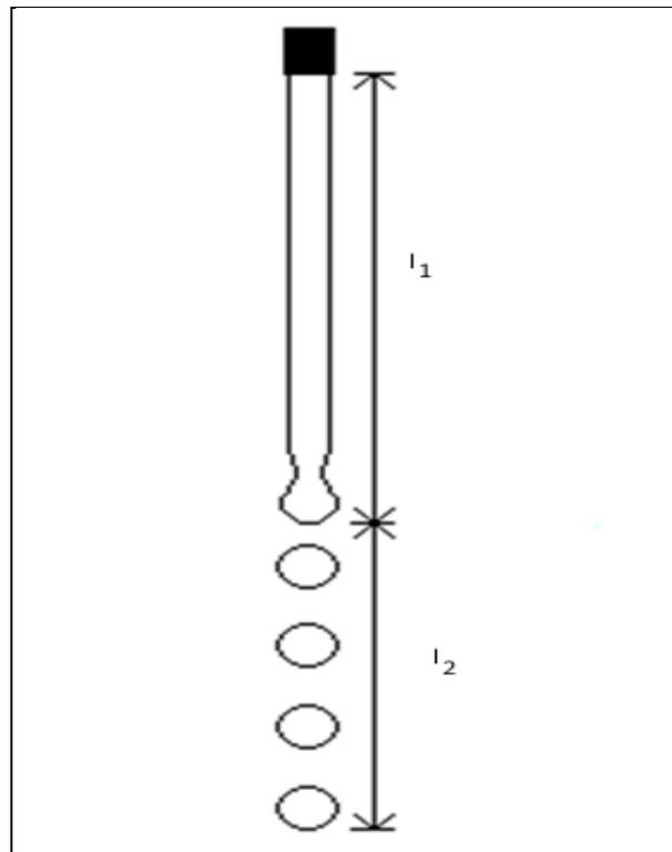
Figure 3-2: Discretization of turbulent liquid jet
