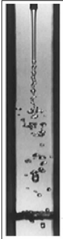
Figure 2-7: Jet disintegration example in the FWI [21].
