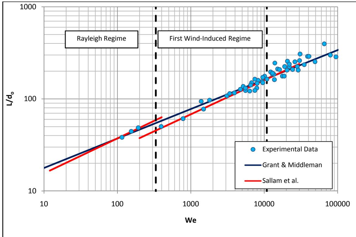
Figure 2-13: Mean liquid column breakup lengths of turbulent round jets [39].
