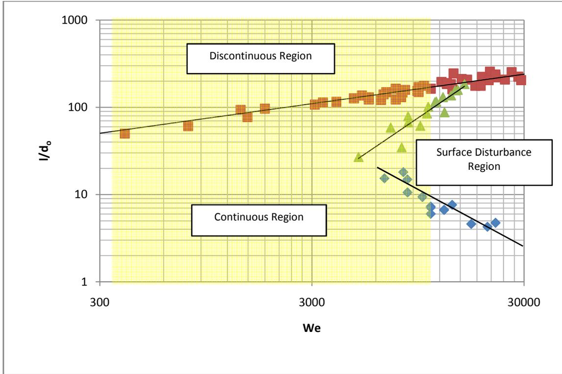
Figure 3-5: Disintegration data and characteristic lengths for turbulent liquid jets in the FWI breakup regime according to Sallam et al. [39] and the present analysis.
