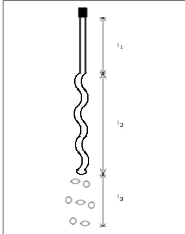
Figure 3-6: Discretization of turbulent liquid jet
