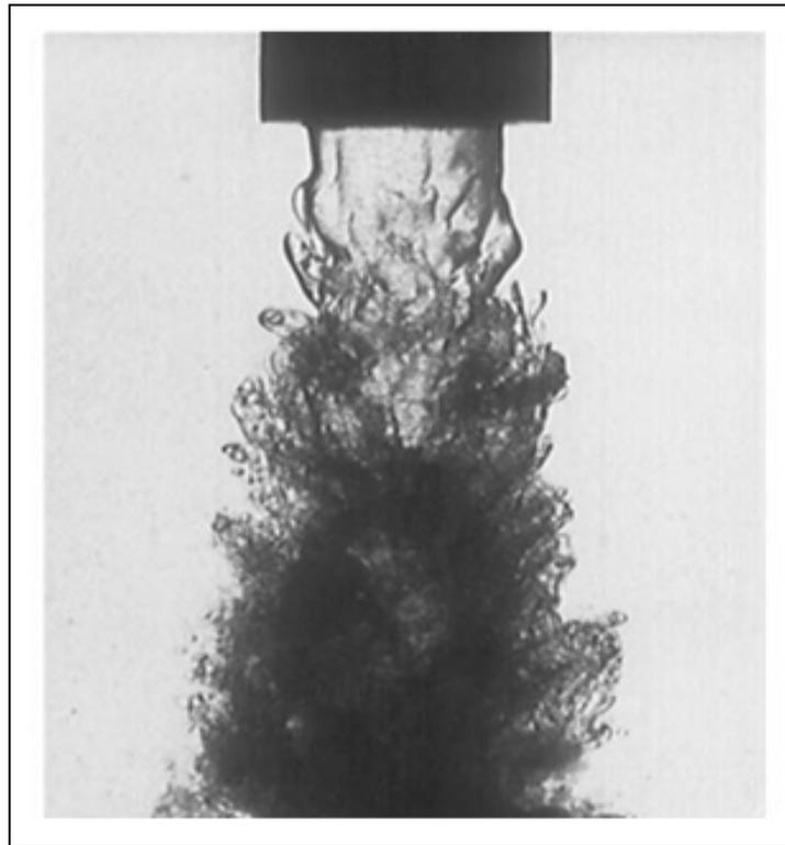
Figure 2-9: Jet disintegration example in the atomization regime [21].
