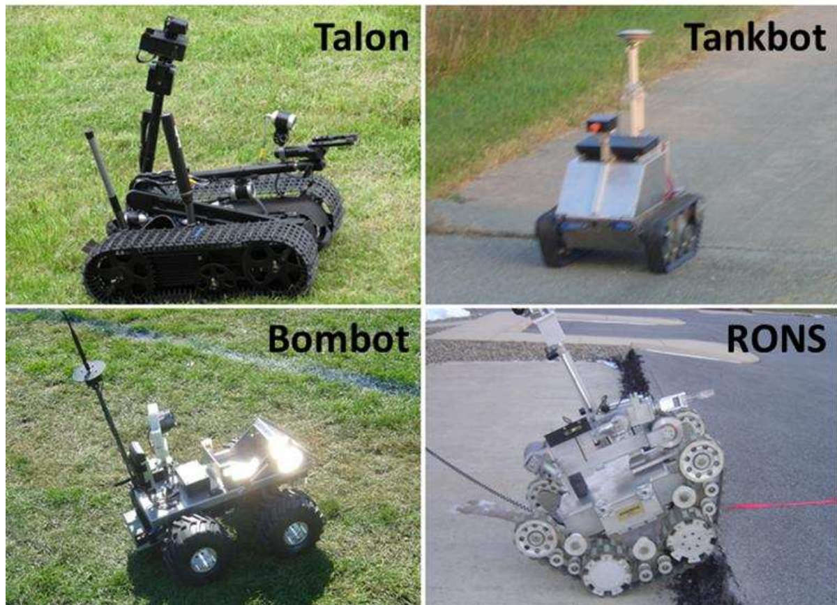
Figure 3-12: Mobile Robot Platforms Used for Testing
