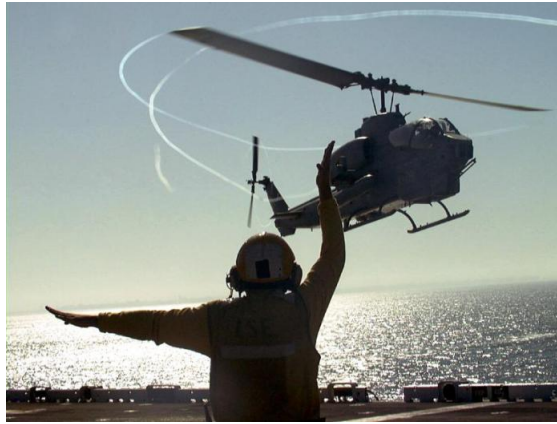
Figure 1.3. Natural condensation trails generated by the tip vortices of the helicopter wake (Photo source: www.jazzroc.wordpress.com ).
