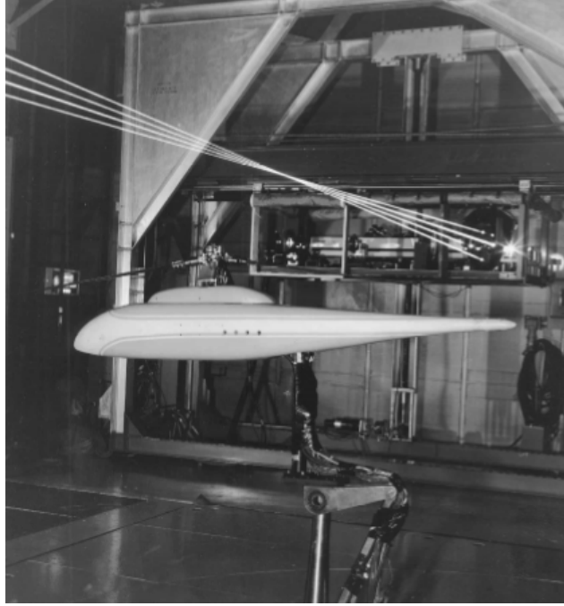
Figure 4.23. Wind-tunnel model used for the current validation cases. [20]
