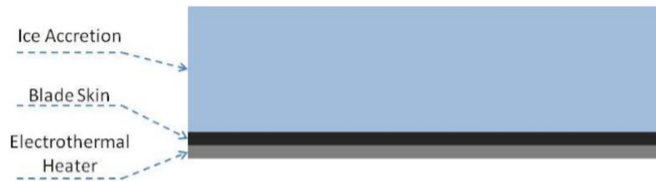
Figure 1.16. Simple Schematic of Electrothermal IPS [2]
