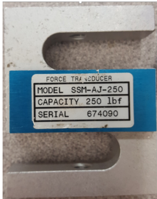
Figure 3.19. 250 lb Range Interface Sealed Load Cell
