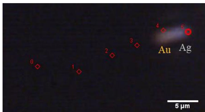
Figure 2-12. Time-tracked image of Au-Ag nanorod moving in iodine (42.3 \mu\text{M} ), recorded in reflectance mode.
