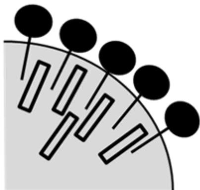
Figure 1.3. Alkane molecules (open rectangles) align with surfactant at the interface and produce a template for crystal nucleation (adapted from Awad and Sato, 2002).
