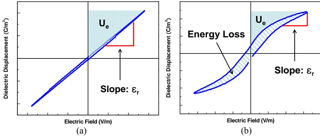
Figure 1.3: P-E of (a) a linear dielectric material and (b) a ferroelectric material that exhibits a hysteretic non-linear response
