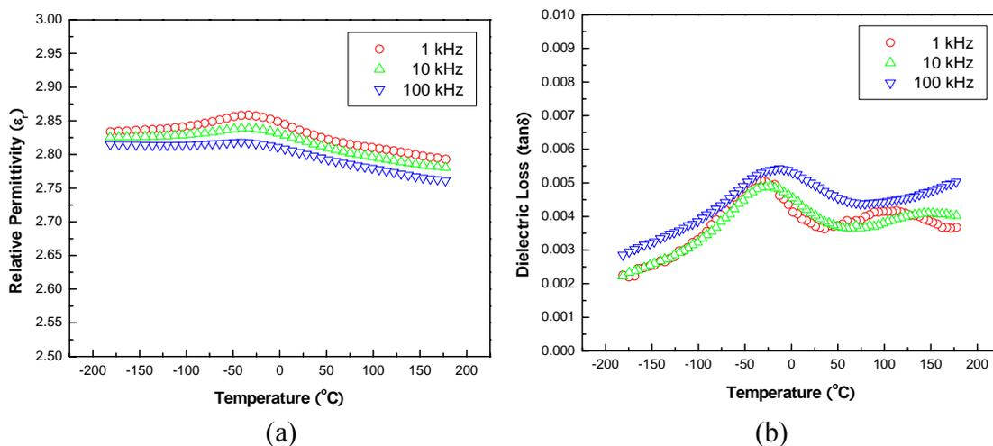
Figure 4.2: Temperature dependence of low-field (a) permittivity ( $\epsilon_r$ ) and (b) dielectric loss ( $\tan\delta$ ) in PI
