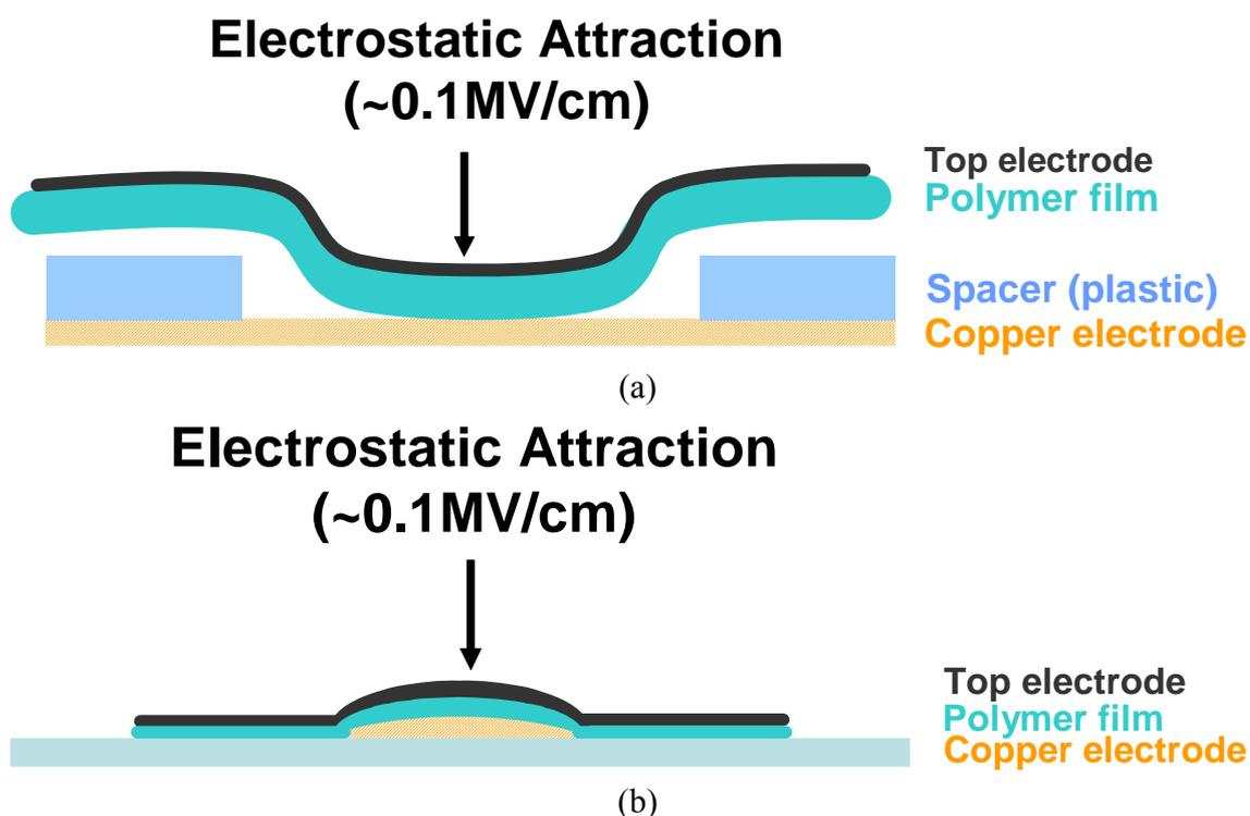
Figure 3.10: Two sample holders including (a) trough holder and (b) mushroom holder used for breakdown-strength measurements
