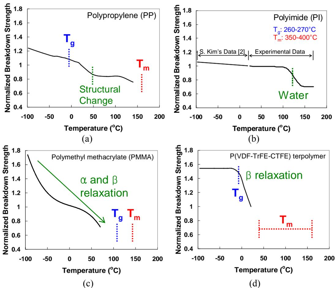
Figure 5.1: Normalized breakdown strength of various polymer films including (a) PP, (b) PI [2], (c) PMMA, and (d) P(VDF-TrFE-CTFE) terpolymer
