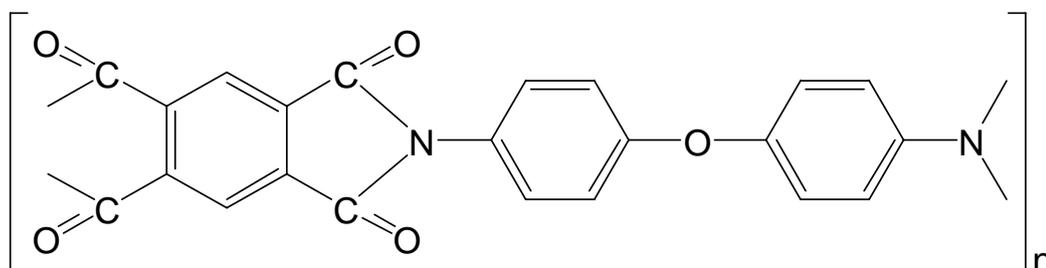
Figure 3.2: Chemical structure of polyimide (PI). The chemical structure of the polyimide is derived from polyamic acid [23]
