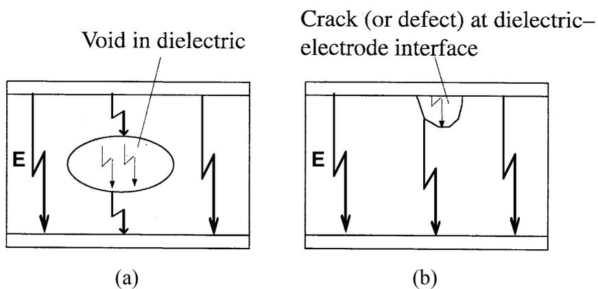
Figure 2.2: Partial discharge when an electric field is applied to (a) a void of a dielectric material, and (b) a crack between the dielectric material and a metallic electrode [1]
