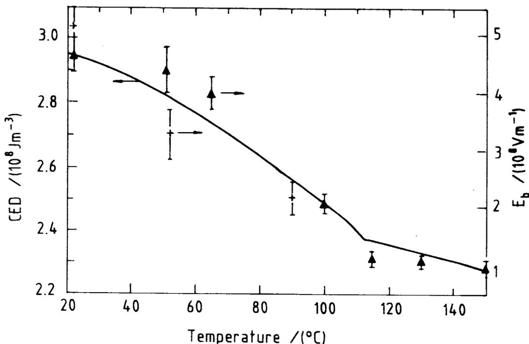
Figure 2.11: Correlation between breakdown strength ( $E_b$ ) and cohesive-energy density (CED) with changing temperature for low-density polyethylene (LDPE). The solid line indicates the cohesive-energy density, and the symbols define the breakdown strength [2]
