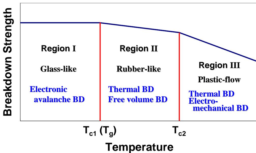
Figure 2.8: Outline of the temperature dependence of breakdown strength in linear polymers [4]
