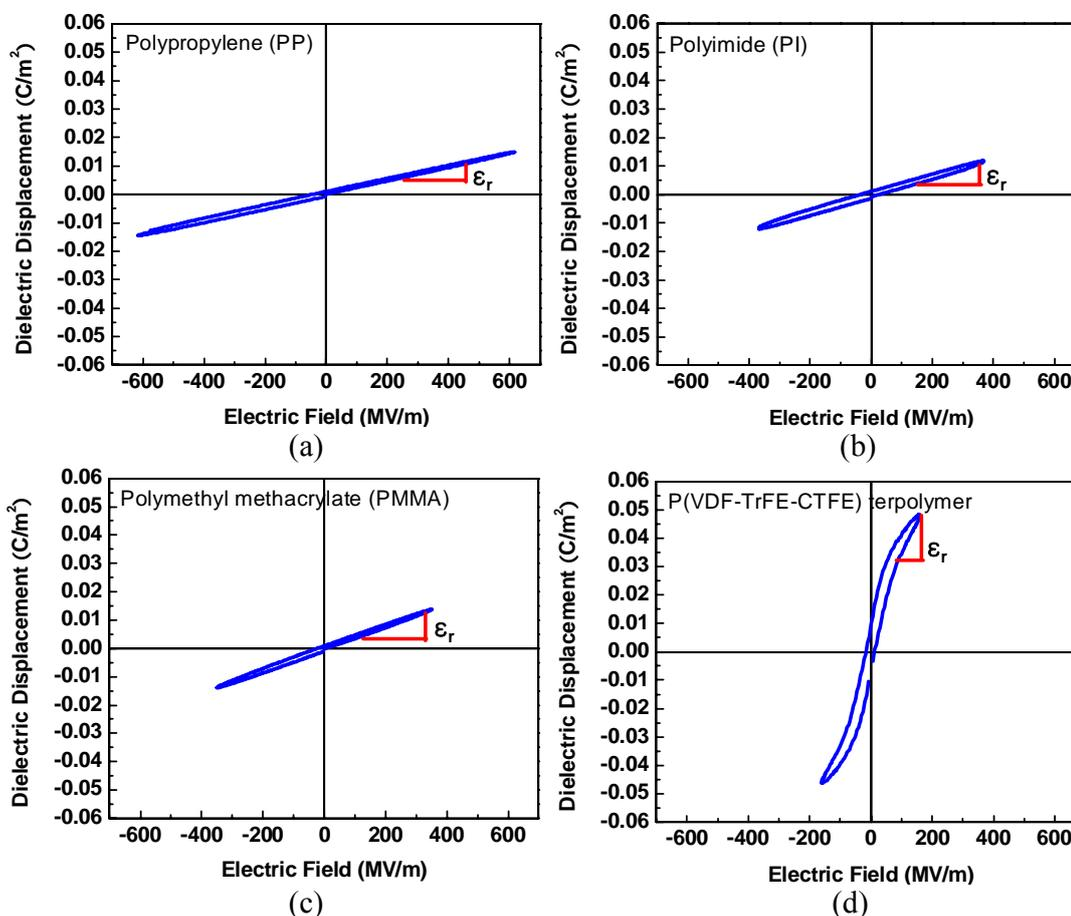
Figure 4.5: Dielectric displacement of various polymer films including (a) PP, (b) PI, (c) PMMA, and (d) p(VDF-TrFE-CTFE) terpolymer at room temperature
