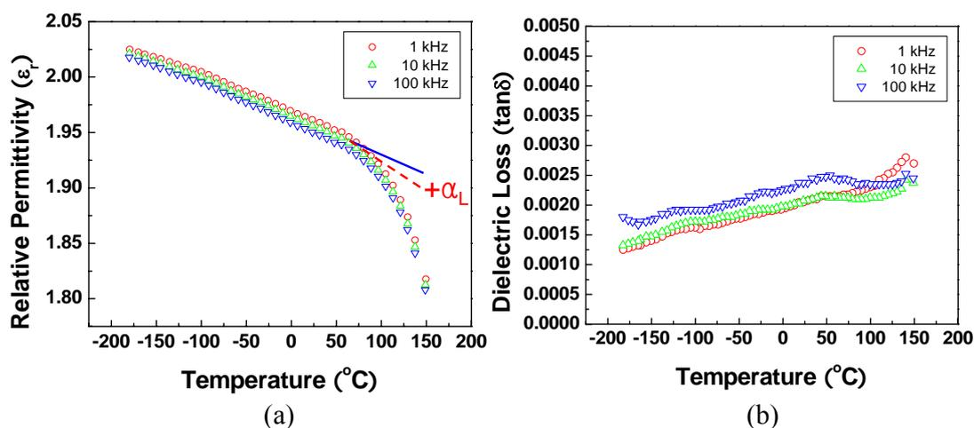
Figure 4.1: Temperature dependence of low-field (a) permittivity ( $\epsilon_r$ ) and (b) dielectric loss ( $\tan\delta$ ) of PP films
