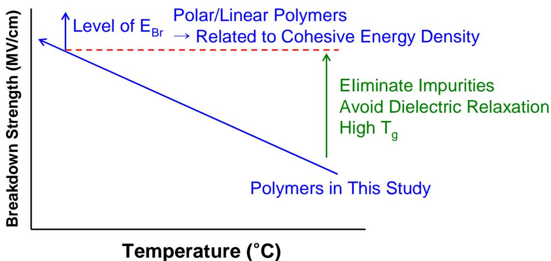
Figure 5.3: Design of optimum polymers to enhance energy density
