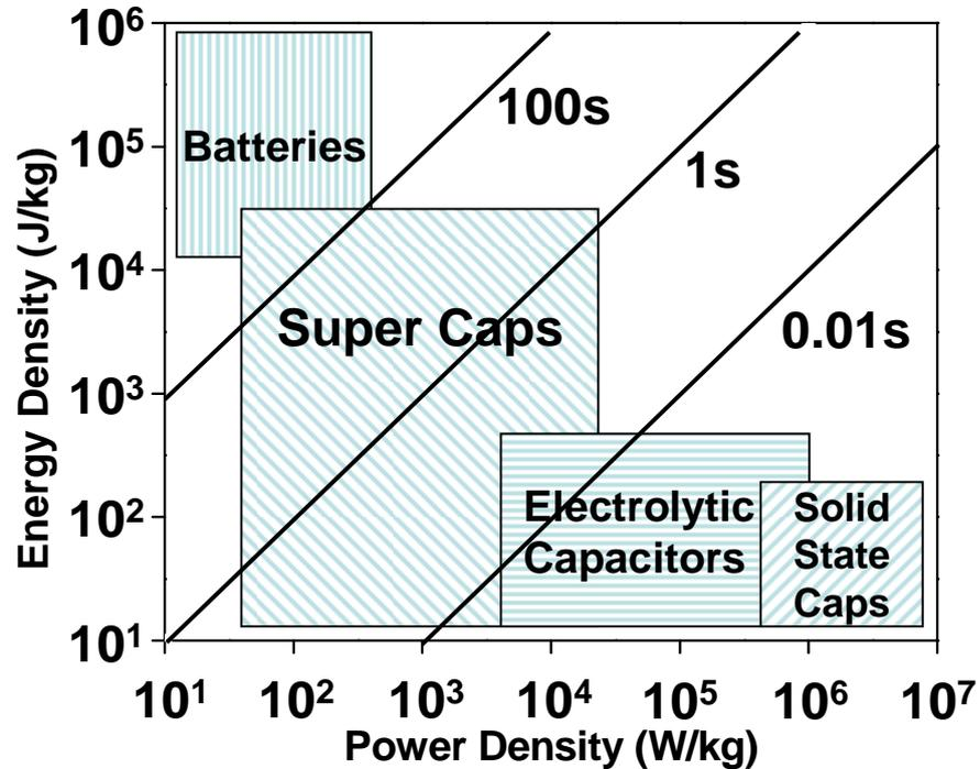
Figure 1.1: Power density vs. energy density for various energy storage components. Capacitors possess high-power densities as a result of a short discharging time [1]
