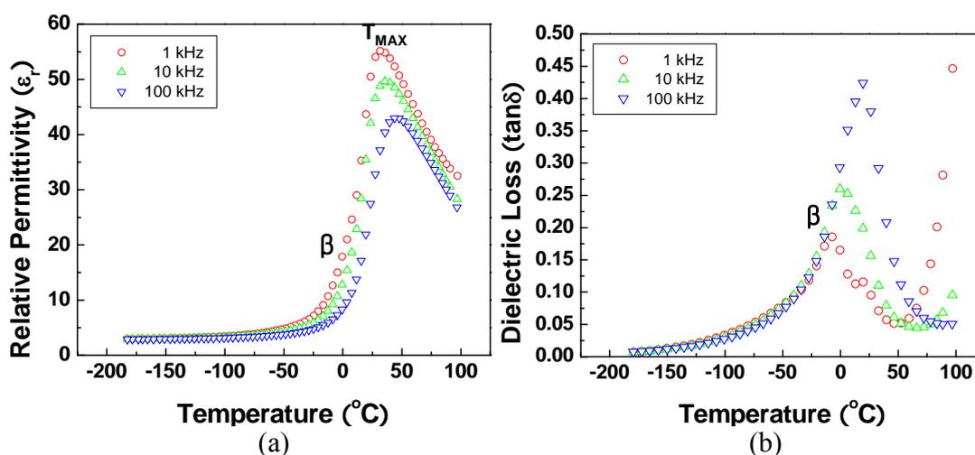
Figure 4.4: Temperature dependence of low-field (a) permittivity ( $\epsilon_r$ ) and (b) dielectric loss ( $\tan\delta$ ) of p(VDF-TrFE-CTFE) terpolymer
