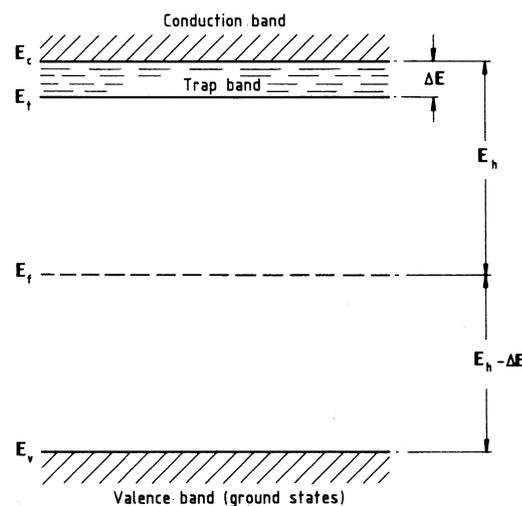
Figure 2.3: Fröhlich's energy band model. It is assumed that a trap band is directly below a conduction band [2]
