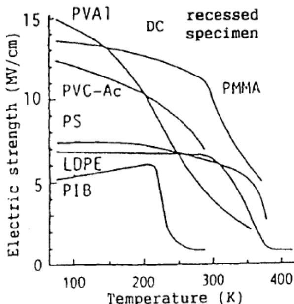
Figure 1.5: Temperature dependence of electric strength in polymer dielectrics. The electric strength increased with decreasing temperature [7]
