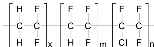
Figure 3.4: Chemical structure of p(VDF-TrFE-CTFE) terpolymer. CTFE is introduced into the p(VDF-TrFE) copolymer. Properties of the terpolymer vary with changing chemical composition
