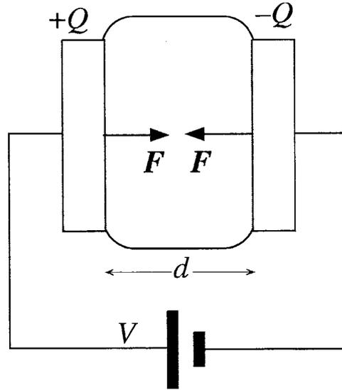
Figure 2.6: Electrostatic force is induced between electrodes when an electric field is applied to the electrodes [1]
