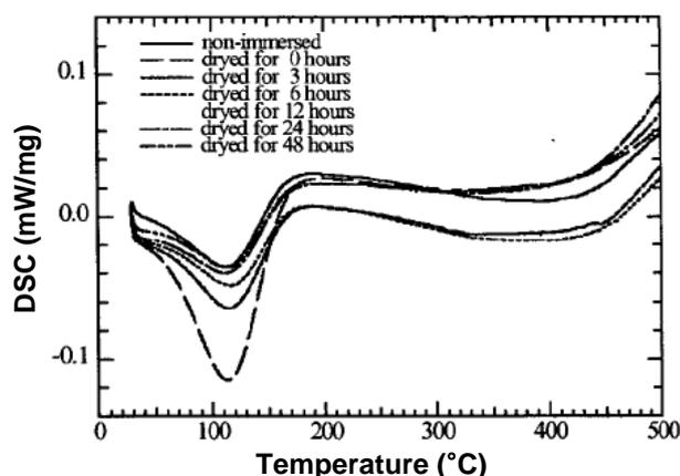
Figure 4.7: Differential scanning calorimetry (DSC) data for PI with various water contents [17]
