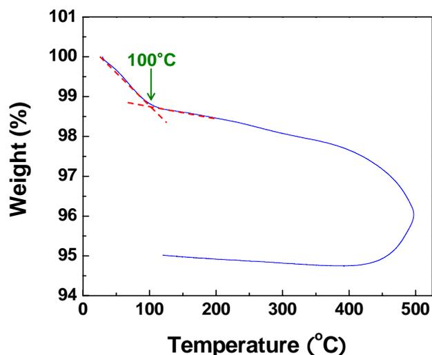
Figure 4.8: Thermogravimetric analysis (TGA) data for PI which shows a change in weight percent with changing temperature
