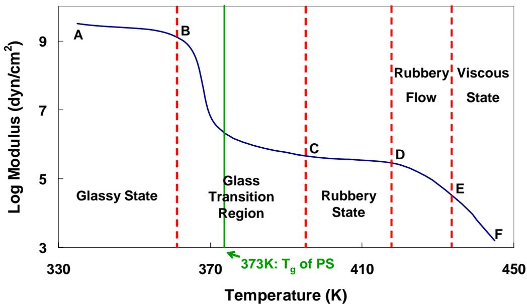
Figure 2.9: Five regions of viscoelasticity depending on temperature for polystyrene (PS). Relaxation modulus of PS varies with temperature [8]
