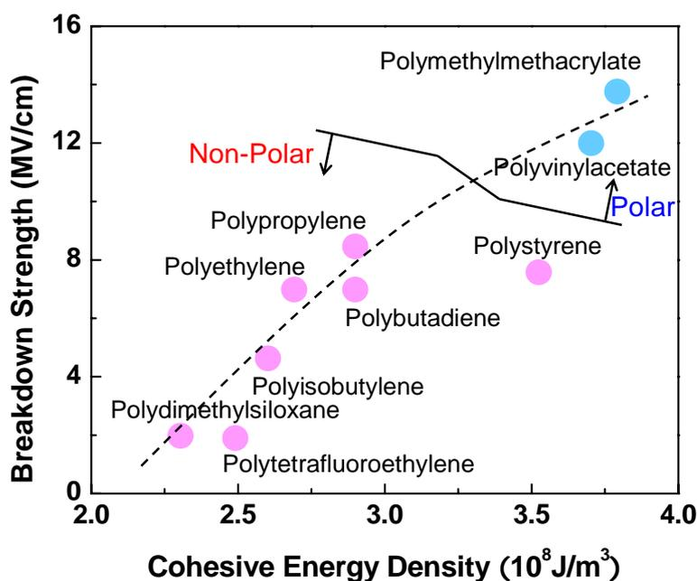
Figure 2.10: Correlation between breakdown strength and cohesive energy-density in polar/non-polar polymers [2, 13, 14]
