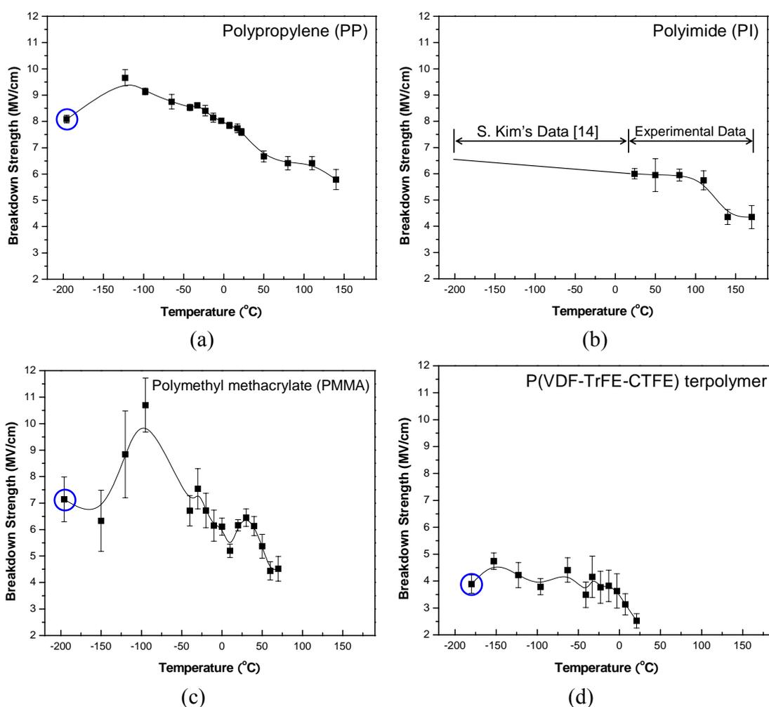
Figure 4.9: Temperature dependence of breakdown strength in various polymer films including (a) PP, (b) PI [14], c) PMMA, and (d) p(VDF-TrFE-CTFE) terpolymer. Circles (○) indicate breakdown data using liquid nitrogen
