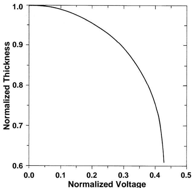
Figure 2.7: Normalized thickness of a rubbery material as a function of normalized voltage [2]
