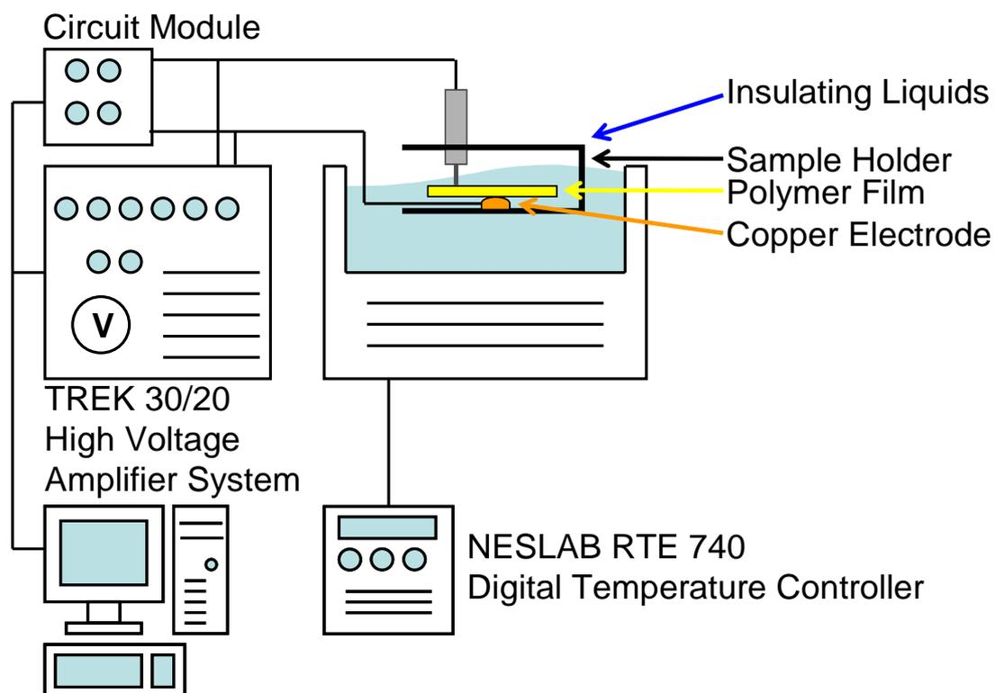
Figure 3.8: Experimental setup for dielectric-displacement and -breakdown measurements. Temperatures were maintained for the breakdown measurements [27]
