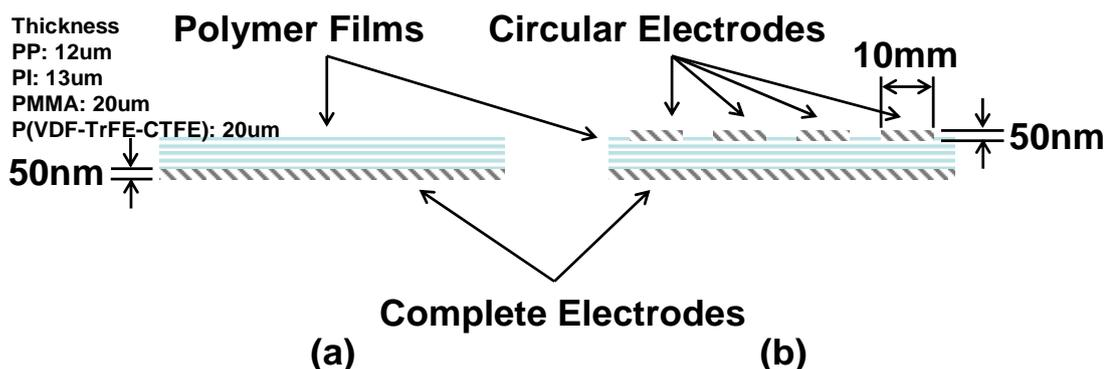
Figure 3.6: Electrode configurations for measurements of electrical properties including (a) breakdown (b) relative permittivity, dielectric loss, and dielectric displacement
