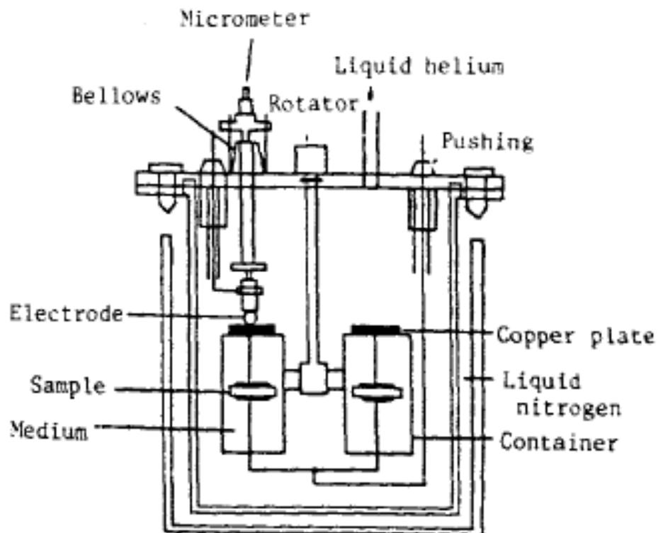
Figure 5.2: Experimental setup for low-temperature breakdown measurements [2]
