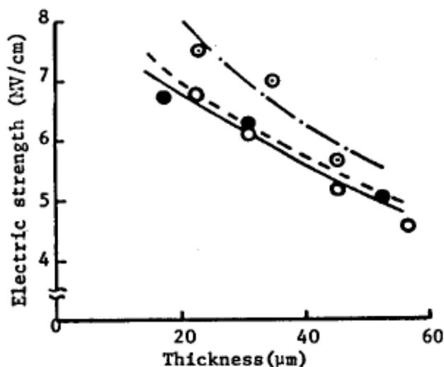
Figure 2.4: Thickness-dependent DC breakdown strength in LDPE films at  $-196^{\circ}\text{C}$  [5].
