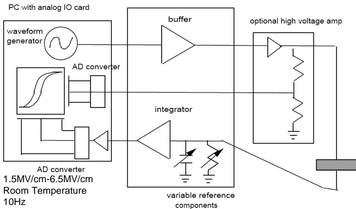
Figure 3.9: Modified Sawyer-Tower circuit at 1.5MV/cm–6.5MV/cm, 10Hz, and room temperature. In P-E, a linear dielectric shows a linear response, and a ferroelectric material exhibits a non-linear response [27, 29]
