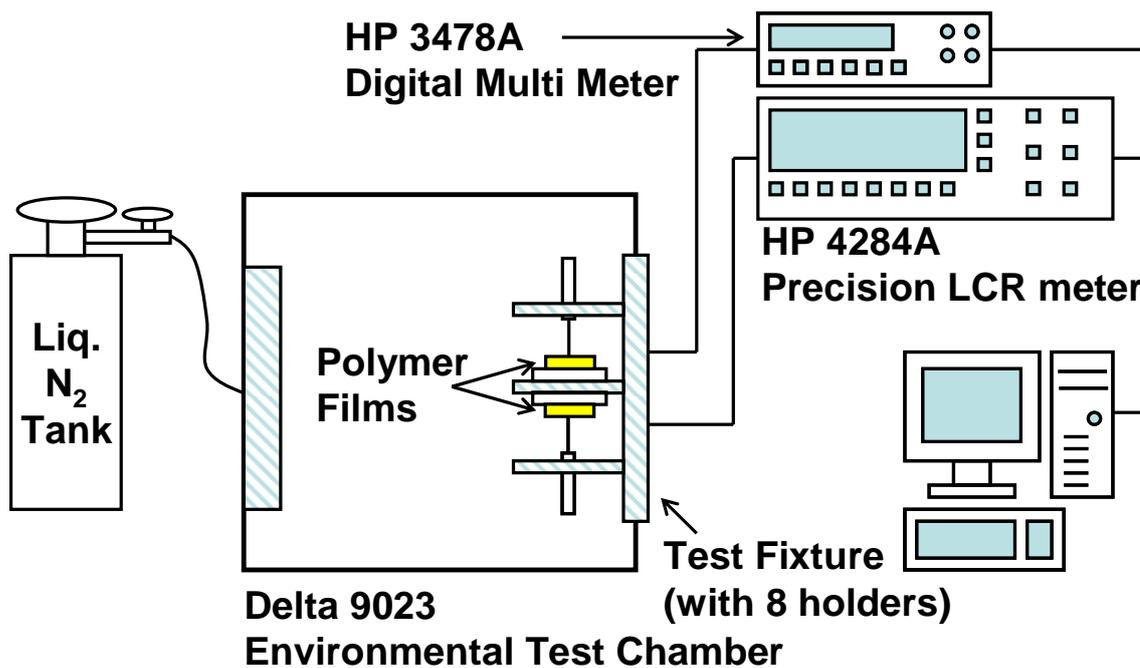
Figure 3.7: Experimental setup for relative permittivity and dielectric-loss measurements [26]
