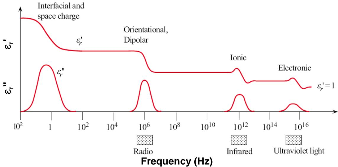
Figure 1.2: Frequency dependence of dielectric permittivity. Dielectric permittivity ( $\epsilon_r'$ ) and loss ( $\epsilon_r''$ ) are affected by frequency [5]
