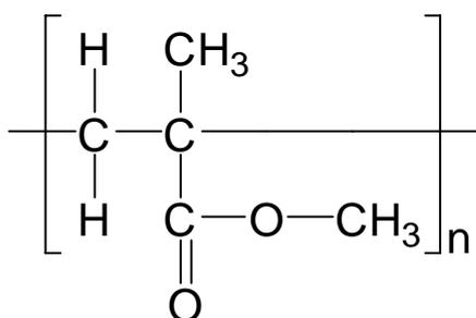
Figure 3.3: Chemical structure of polymethyl methacrylate (PMMA). A monomer of PMMA contains a methyl and a methacrylic group. The tacticity of PMMA chains is defined by the orientation of the groups
