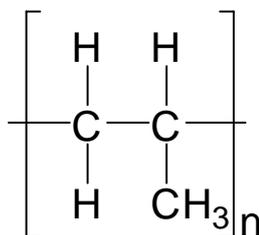
Figure 3.1: Chemical structure of PP. A methyl group is bonded with a carbon of a propylene monomer. The orientation of the methyl groups defines tacticity in PP
