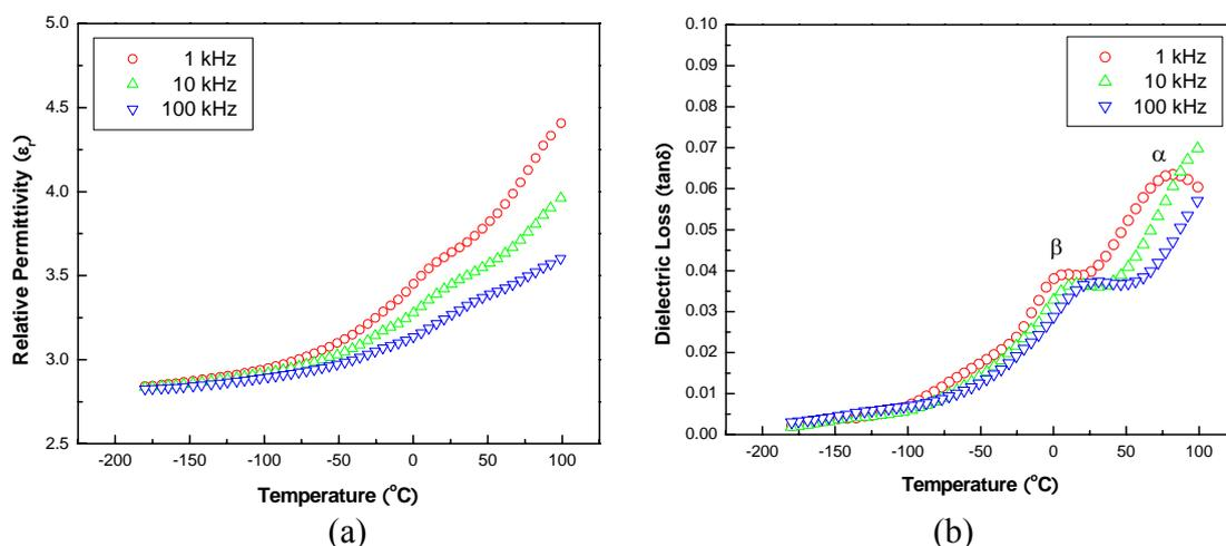
Figure 4.3: Temperature dependence of low-field (a) permittivity ( $\epsilon_r$ ) and (b) dielectric loss ( $\tan\delta$ ) of PMMA
