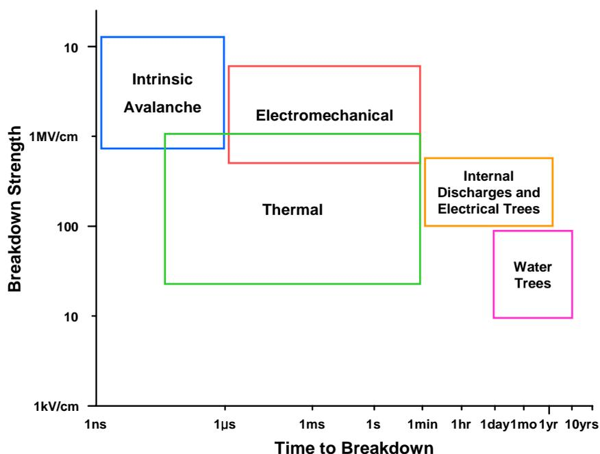
Figure 2.1: Mechanisms of time to breakdown and breakdown strength ( $E_{Br}$ ) when breakdown occurs [1]
