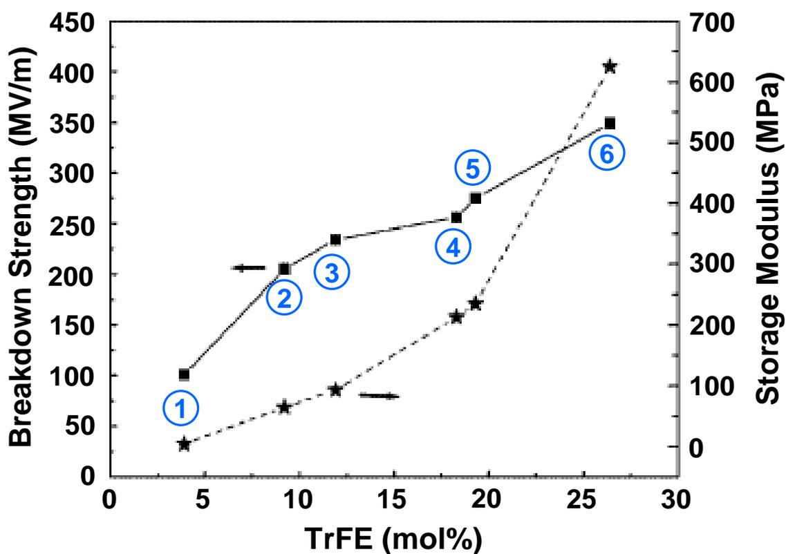
Figure 3.5: TrFE concentration dependence of breakdown strength and storage modulus for p(VDF-TrFE-CTFE) terpolymer [15]
