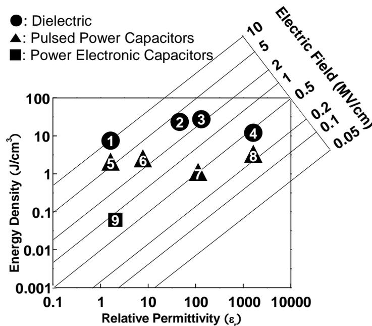
Figure 1.4: Comparison of energy density for various dielectric materials for high-power capacitors. Energy density is limited by dielectric permittivity and the electric field due to breakdown strength of a material. 1) biaxially oriented PP, 2) modified poly(vinylidene fluoride) polymer, 3) titanium oxide dielectric, 4) antiferroelectric/ferroelectric phase switch ceramic, 5) PP film capacitor, 6) PVDF film capacitor, 7, 8) ceramic capacitors, 9) commercial polymer film power capacitor [6]
