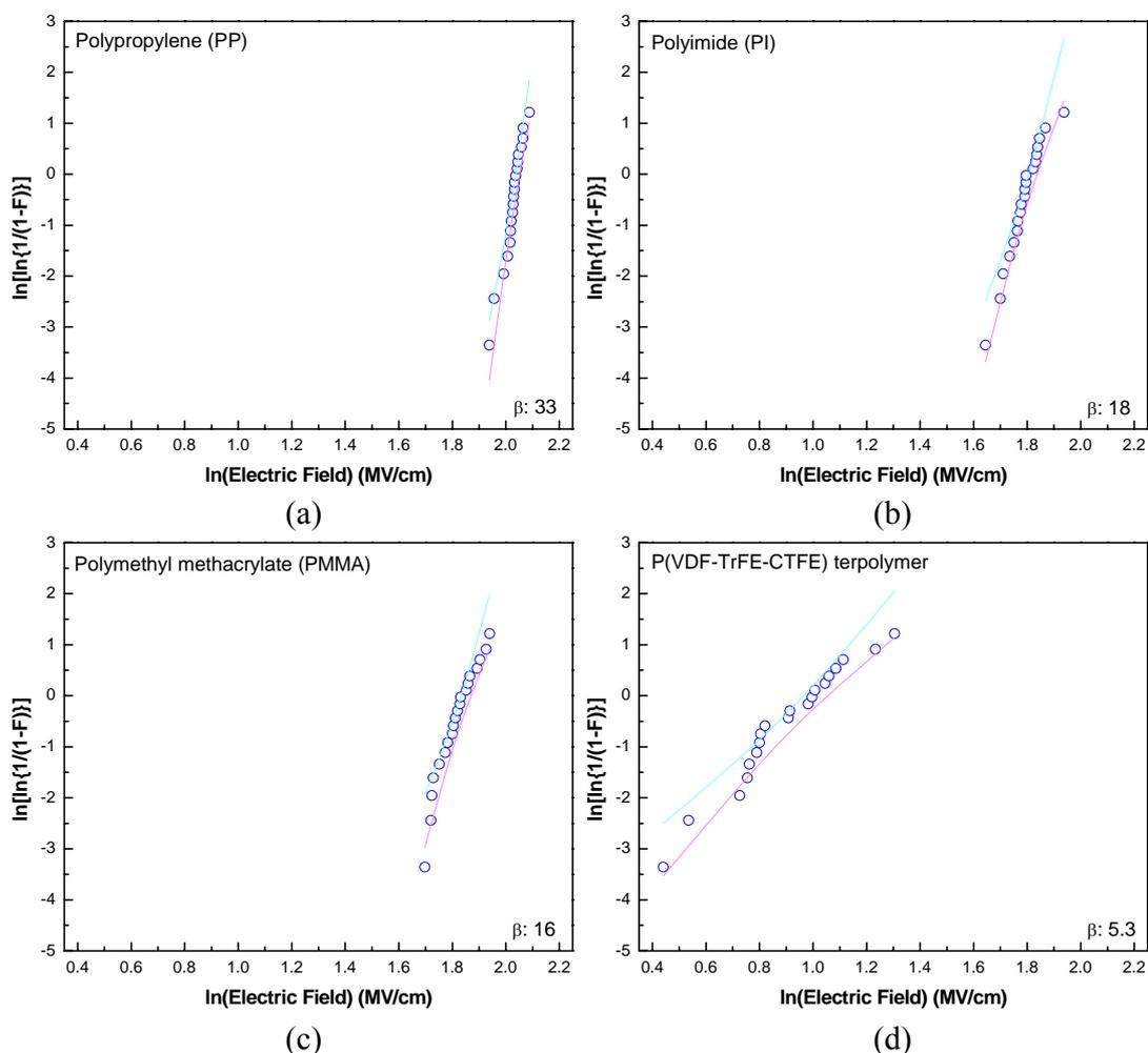
Figure 4.6: Weibull distribution of breakdown in various polymer films at room temperature including (a) PP, (b) PI, (c) PMMA, and (d) p(VDF-TrFE-CTFE) terpolymer
