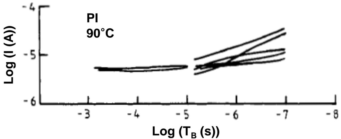
Figure 2.5: Time backward from breakdown dependence of current before breakdown of PI at 90°C [6]
