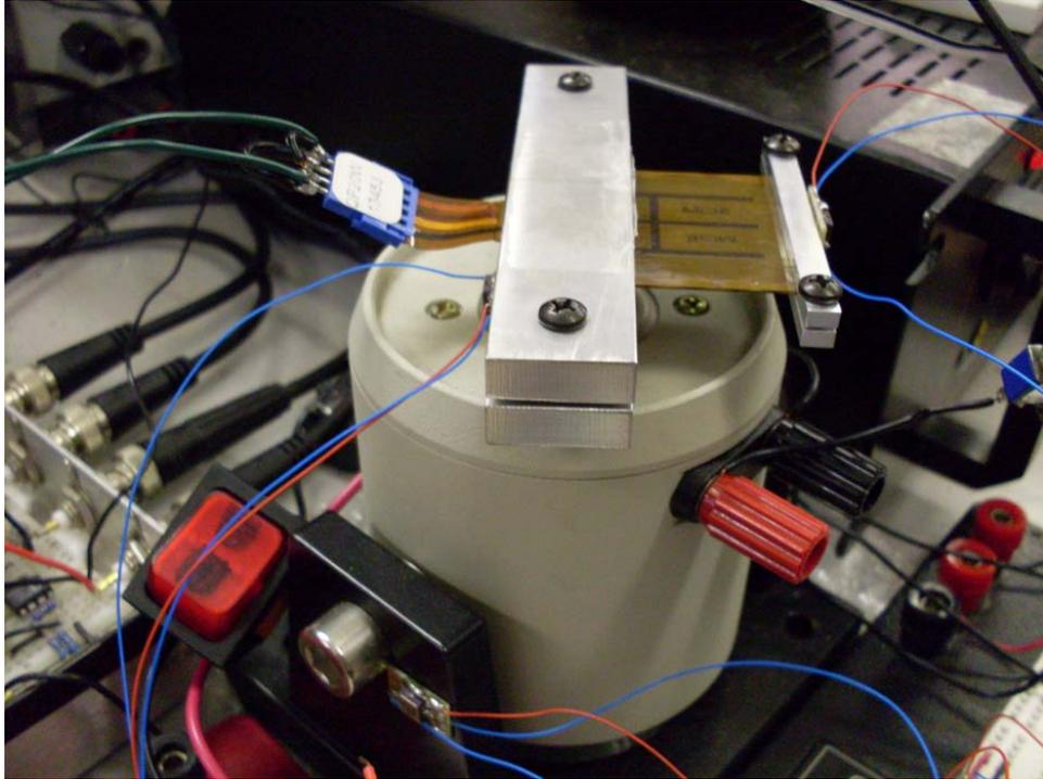
**Figure 6.1.** Experimental setup of the piezoelectric dynamic system
