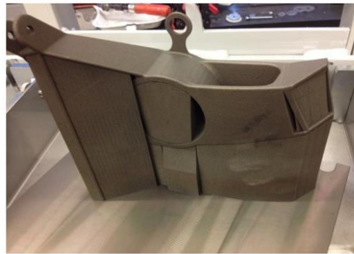
a) Before removing supports
