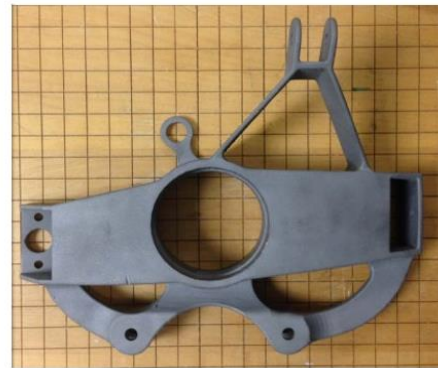
a) After removing supports
