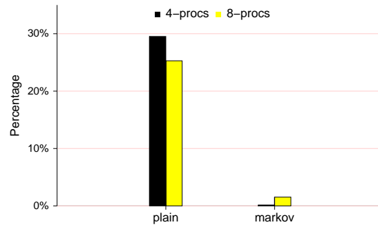
Fig. 3.10. Percentage increase in execution time for mgrid: Last-Value Predictor vs. Markov Predictor.
