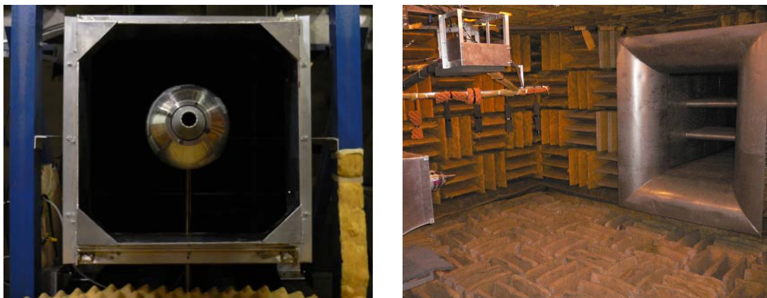
Figure 2-11: Pictures of upstream 15 inches square duct and downstream exhaust collector for forward flight simulation of acoustic measurements inside the anechoic chamber at Penn State.
