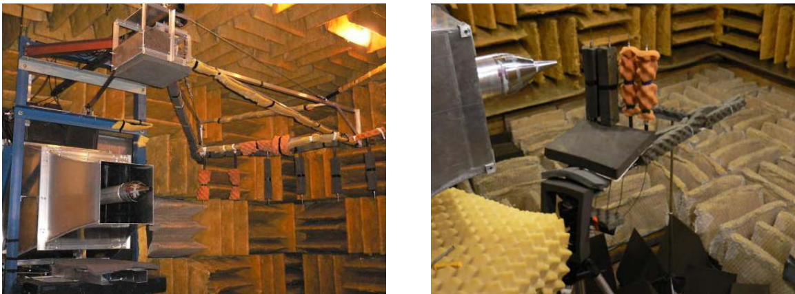
Figure 2-2: Microphone array in The Pennsylvania State University high speed jet noise facility.
