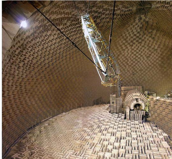
Figure 4-1: The AeroAcoustic Propulsion Laboratory with high flow jet exit rig in the NASA Glenn Research Center.
