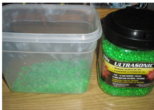
Figure C.1 Material used for the measurement of the singlets-doublets packing fraction. The green BB's are on the right of the image. The container used for the measurement with some BB's is on the left.
