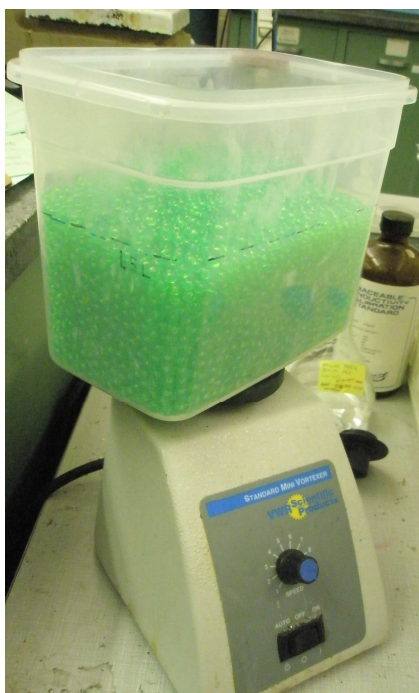
Figure C.2 Measurement of the singlets-doubles packing fraction. The plastic container filled with BB's until the line of 1.5 L was placed on the vortexer to pack the particles tightly.
