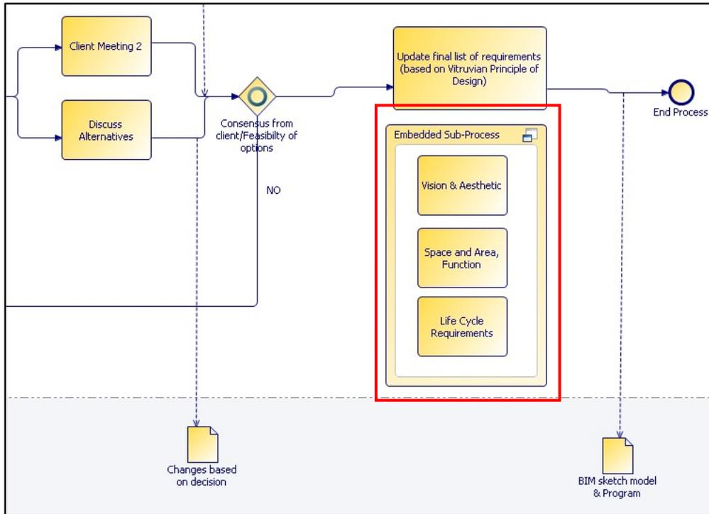
Figure 5-8: Embedded process should not be used as part of template map
