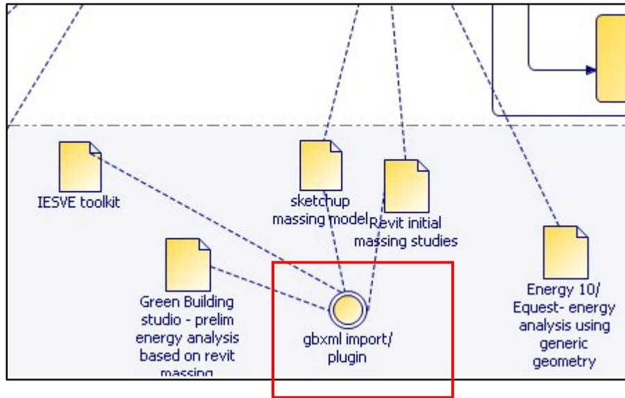
Figure 5-14: Incorrect use of intermediate event
