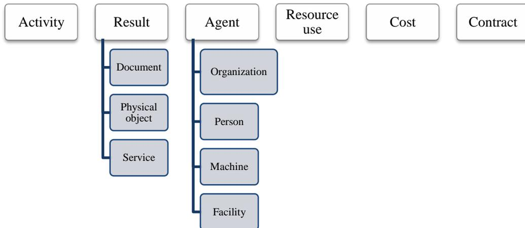
Figure 3-5: Subtypes of the construction process entity (Bjork 1992)
