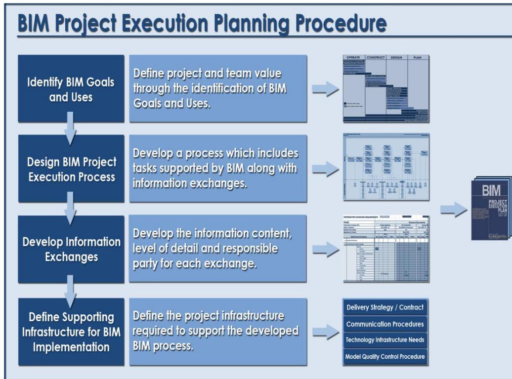
Figure 7-1: The BIM Execution Planning Procedure (The Computer Integrated Construction Research Program 2009)
