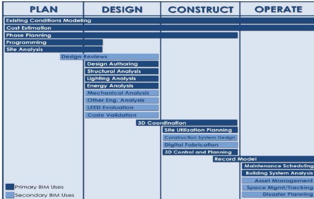
Figure 2-2: BIM Uses throughout a building lifecycle
