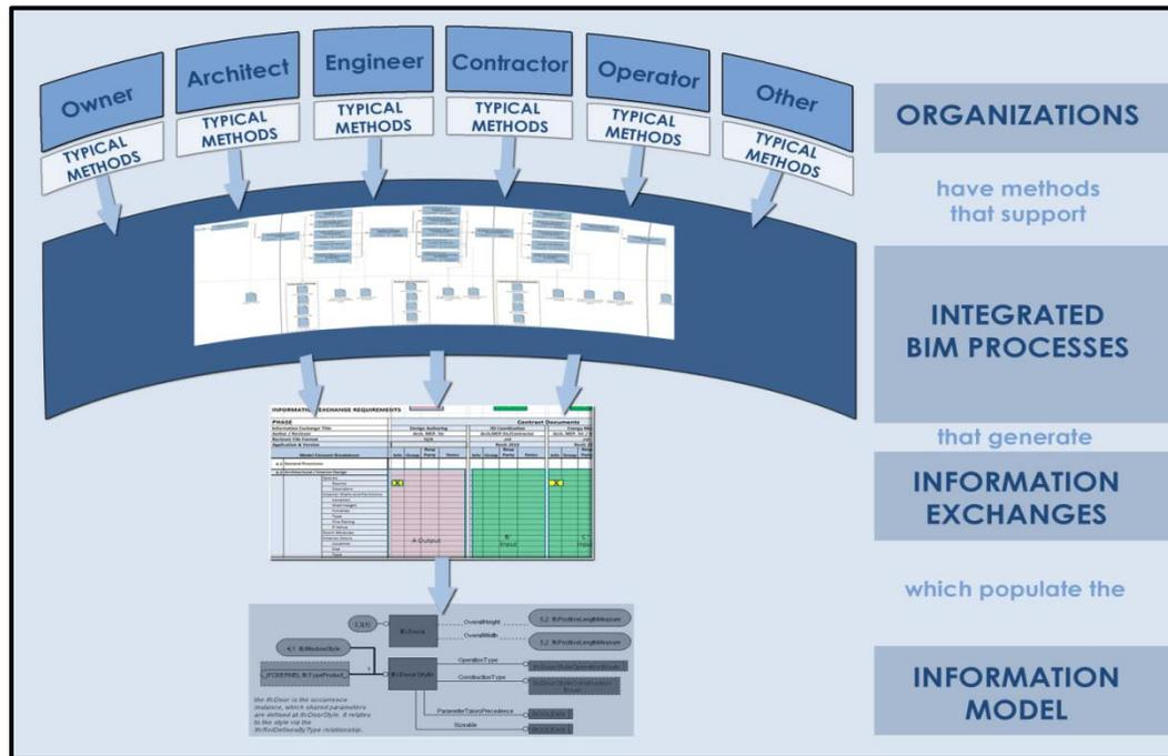
Figure 1-1: BIM Project Execution Planning Process
