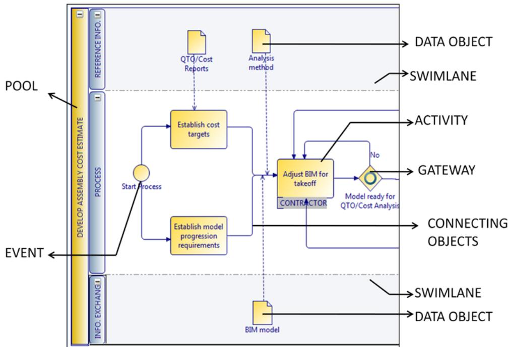
Figure 4-1: Key process mapping objects
