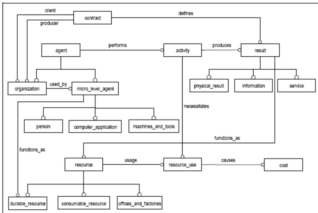
Figure 3-6: A model of generic construction categories, showing some of their internal relationships (Bjork 1995)
