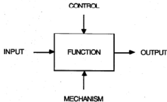
Figure 3-2: IDEF0 box and arrow graphics (Sanvido et al. 1990)
