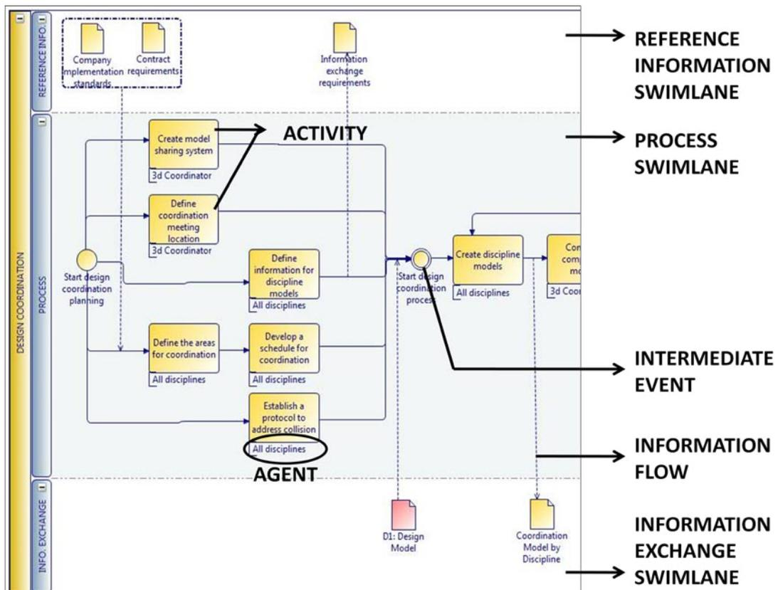
Figure 4-5: Terminology used for BIM process mapping (adopted from BPMN)
