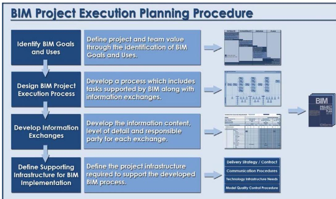
Figure 1-2: BIM Project Execution Planning Procedure
