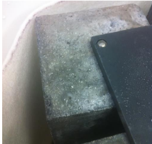
Figure 2-3: Water condensed on the surface of the concrete prism. This water causes alkali leaching and ultimately stops ASR.
