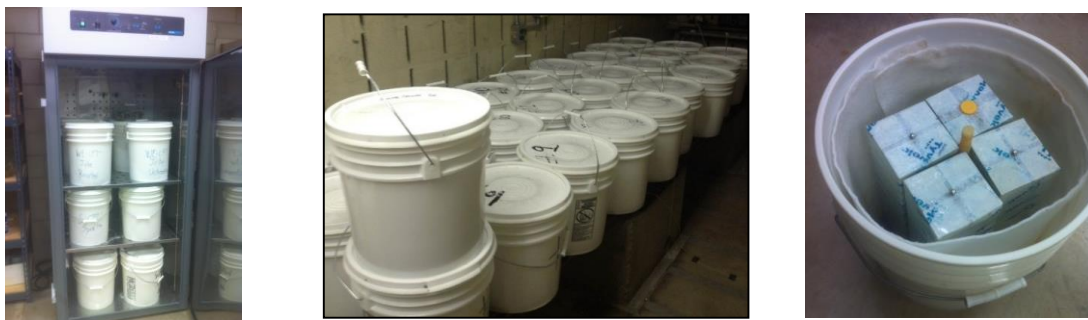
Figure 2-6: Left: 60^\circ\text{C} oven and storage buckets used in this study. Center: 38^\circ\text{C} warm room and buckets used in this study. Right: Sealed prisms placed in identical storage conditions as described in ASTM C1293. These buckets were then stored at 38^\circ\text{C} or 60^\circ\text{C} .
