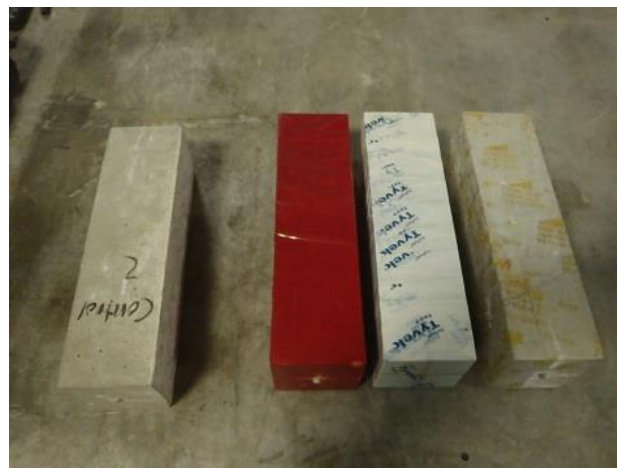
Figure 2-5: Various sealed concrete prism specimens sealed using various moisture barriers. Tyvek tape is used on the third prism from the left and was used in all S-CPT and WE-CPT testing.
