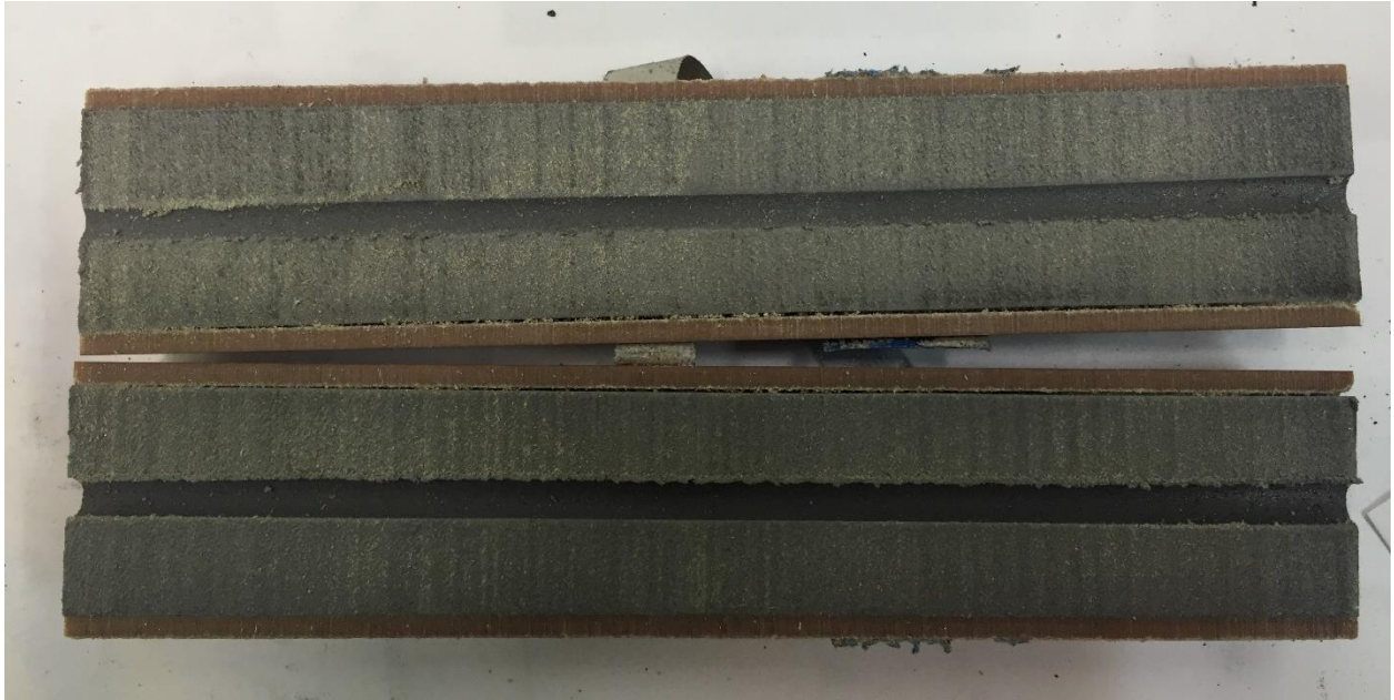
Figure E.4: Sectioned fuel grain that was X-rayed and found to be detaching away from the phenolic casing.
