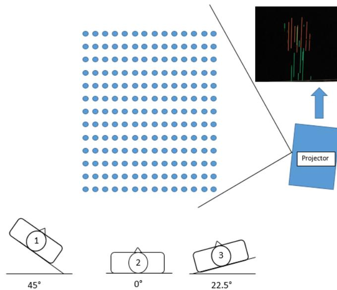
**Figure 5: Schematic drawing showing an overhead view of three different observers (1-3) of the volumetric display. Observers 1 and 2 view the display at  $45^\circ$  and  $0^\circ$ , respectively, which are bad viewing angles because only a few strings may be viewed without obstruction by other strings. Such poor viewing angles are repeated at  $45^\circ$  increments around the display. Observer 3 has a better viewing angle that permits observation of more strings at once.**
