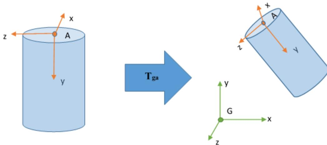
Figure 25: The transformation between the segment anatomical coordinate system A and the ground coordinate system G was used to locate a cylinder representing each segment in the ground coordinate system prior to finding string intersections.
