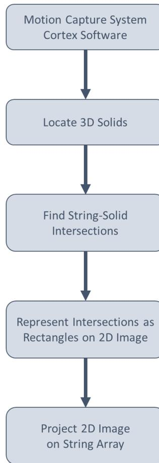
**Figure 6: Overview of steps taken to display three-dimensional motions using the string display.**
