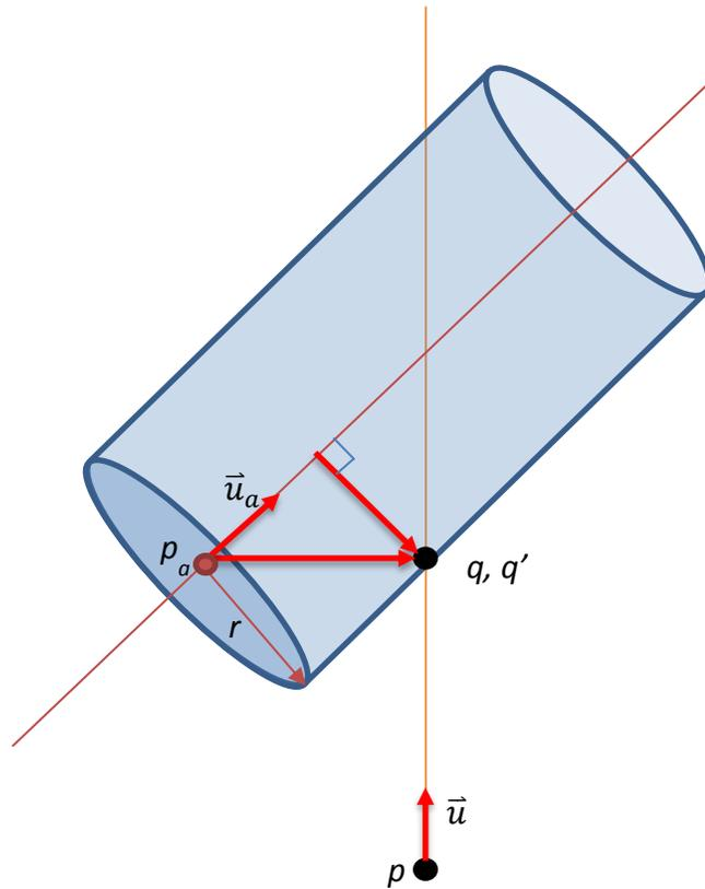
**Figure 15: Intersection of a line (defined by point  $p$  and vector  $u$ ) and a cylinder. The intersection is solved for by finding the roots of a quadratic equation in terms of the distance  $s$  from  $p$  along  $u$ .**
