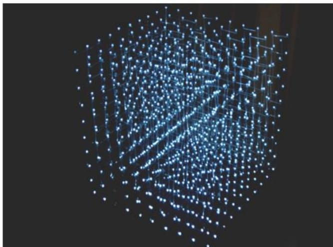
**Figure 3: Volumetric 10 x 10 x 10 LED display (Schubiger-Banz and Eberle, 2008).**
