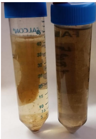
Figure 7. Examples of how minor adjustments in pH can affect the viscosity of the product. Shown at the left is a product of the ligand-free Pt synthesis done at pH > 13. At the right is the product of the same reaction; however the reaction pH was <13.
